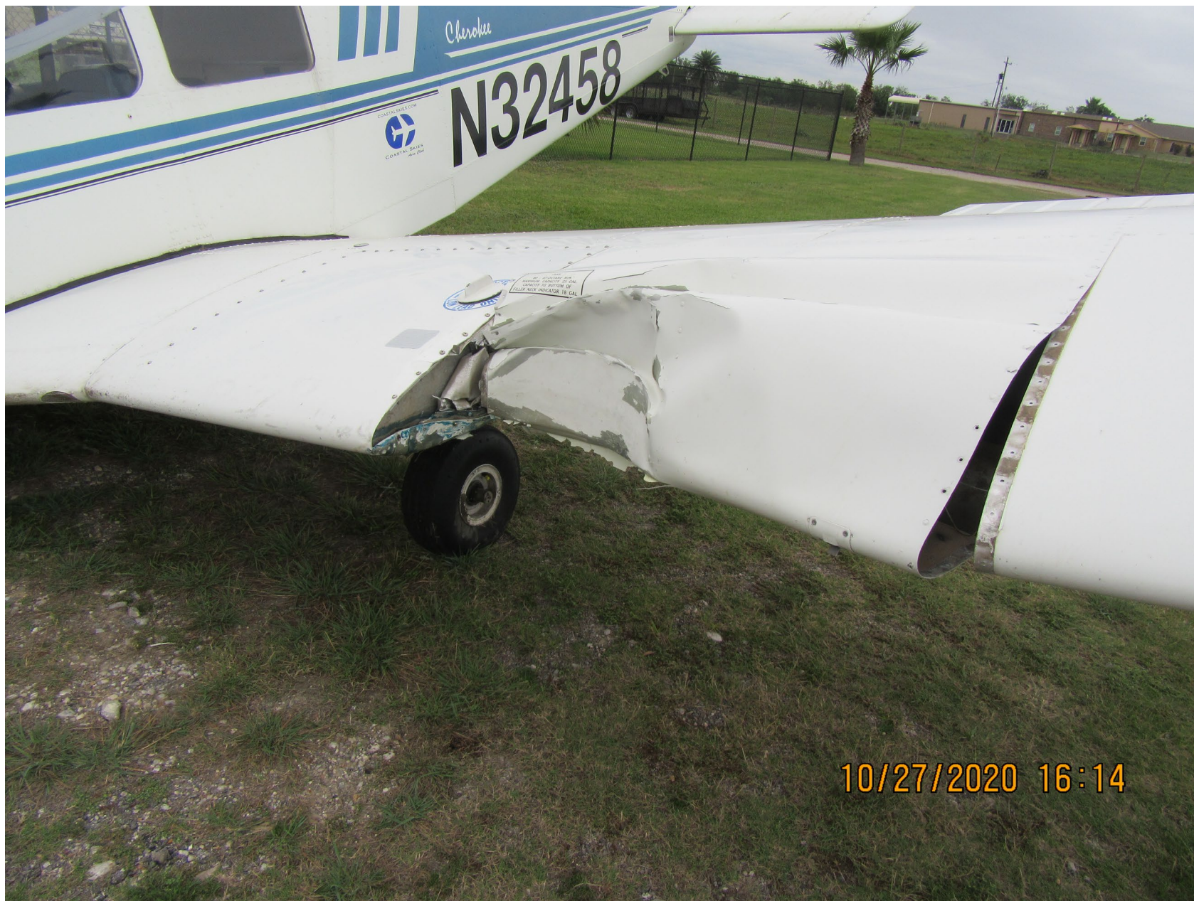
Photo 5 - Left Wing Damage (FAA Photo)
