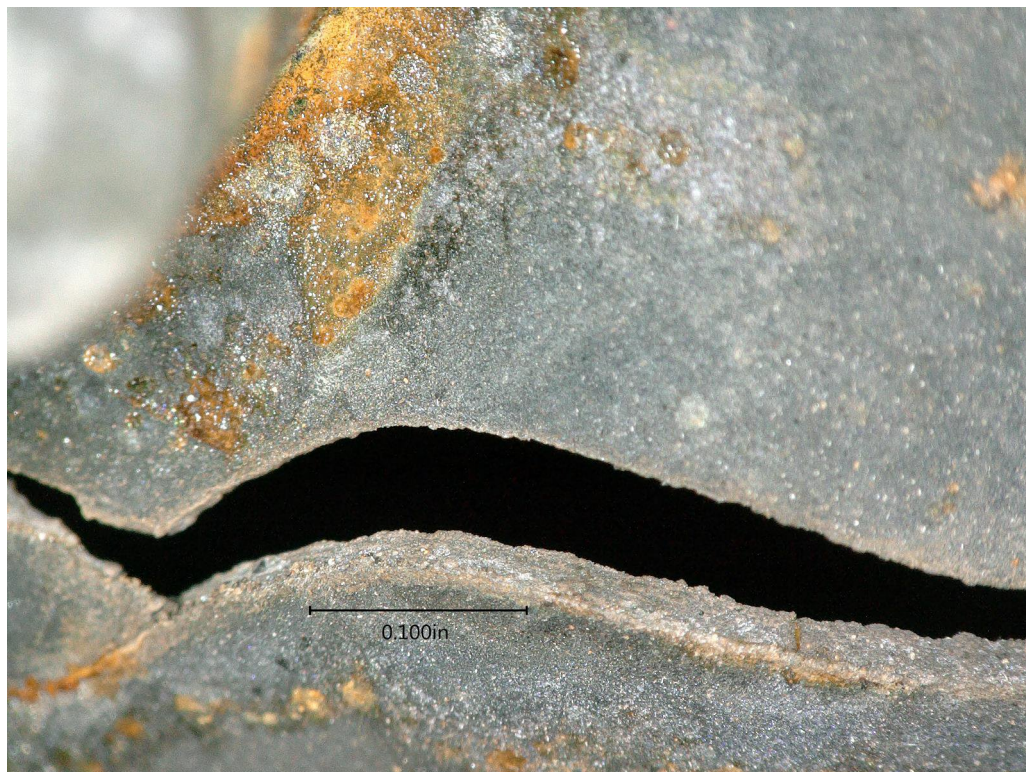
Figure 6: Crack fracture face exhibiting corrosion on the surface.
