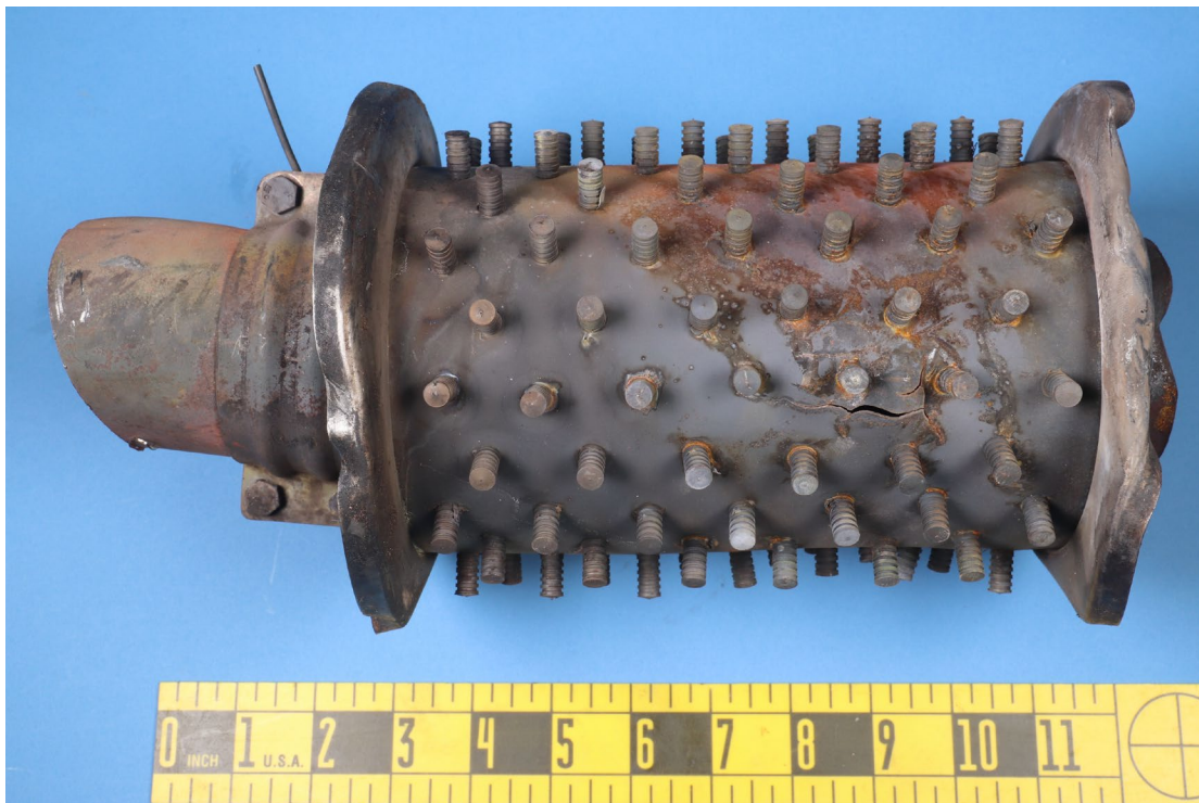
Figure 4: Heat exchanger with cover removed exposing the barrier between the exhaust gas and cabin air.
