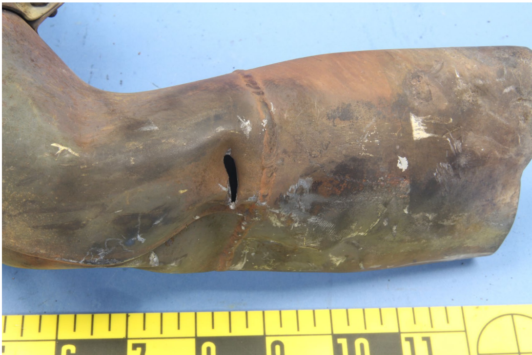
Figure 2: Crack on exhaust gas pipe
