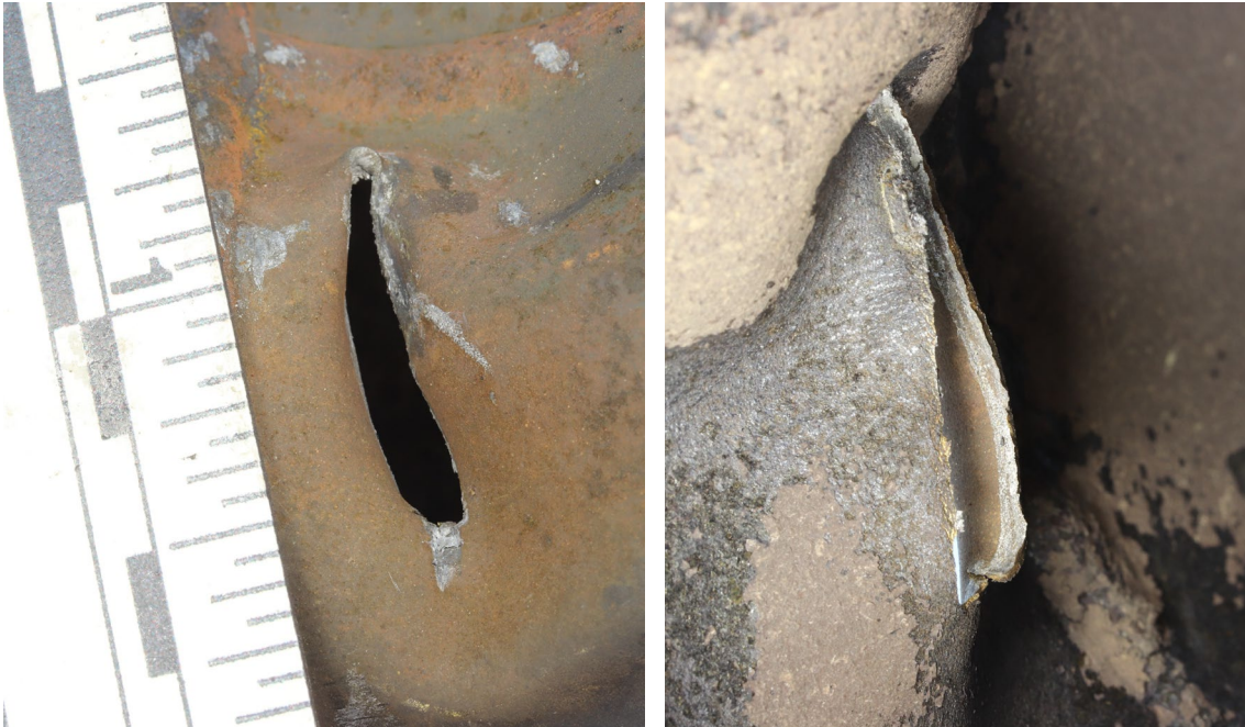
Figure 3: External and internal views of the crack on the exhaust gas pipe.
