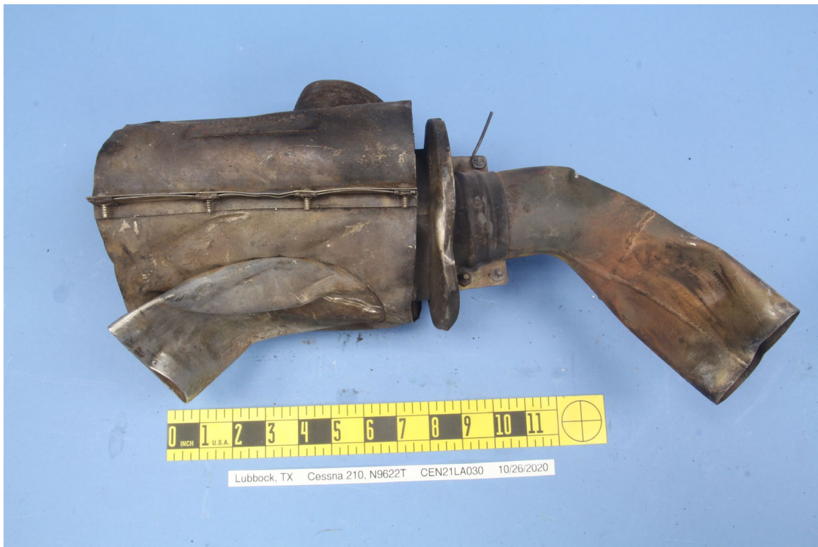
Figure 1: Portion of heat exchanger as received.
