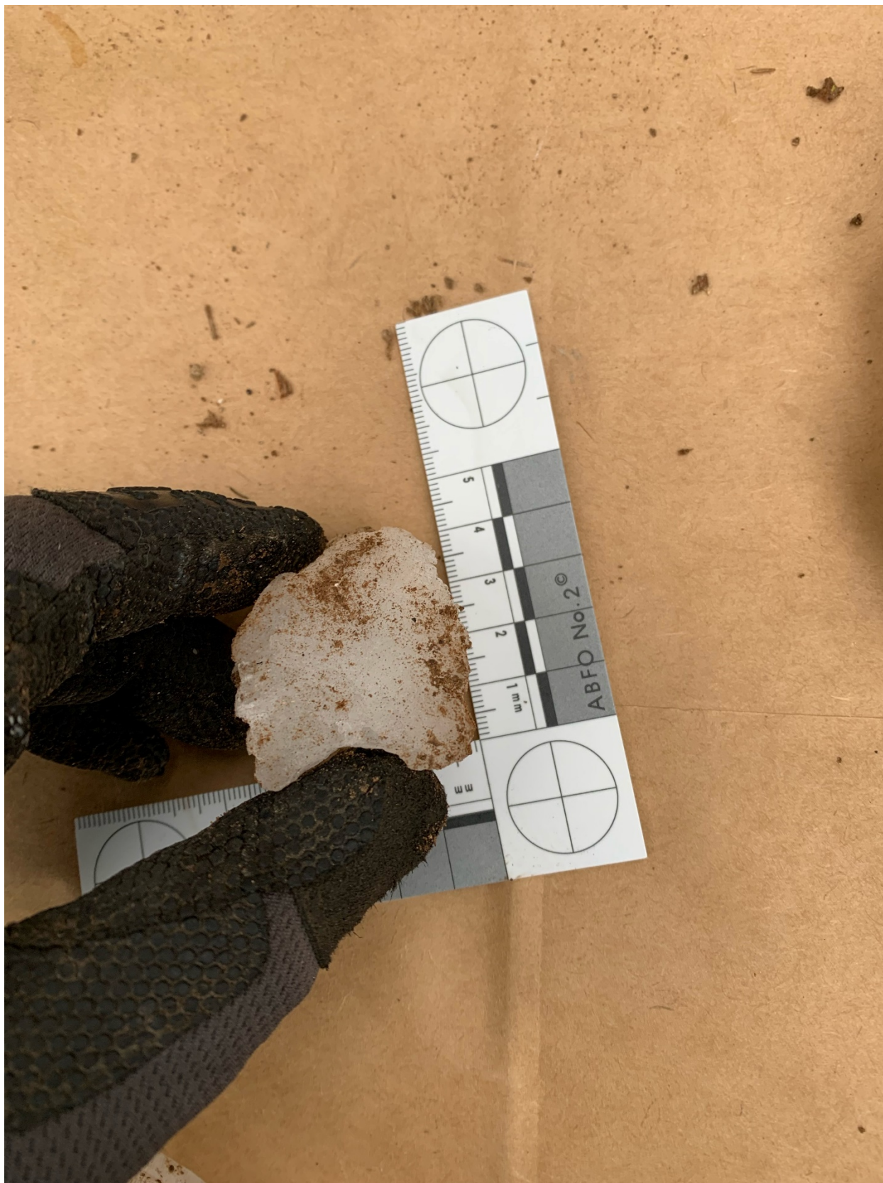
Figure 21 – Ice found near the accident aircraft
