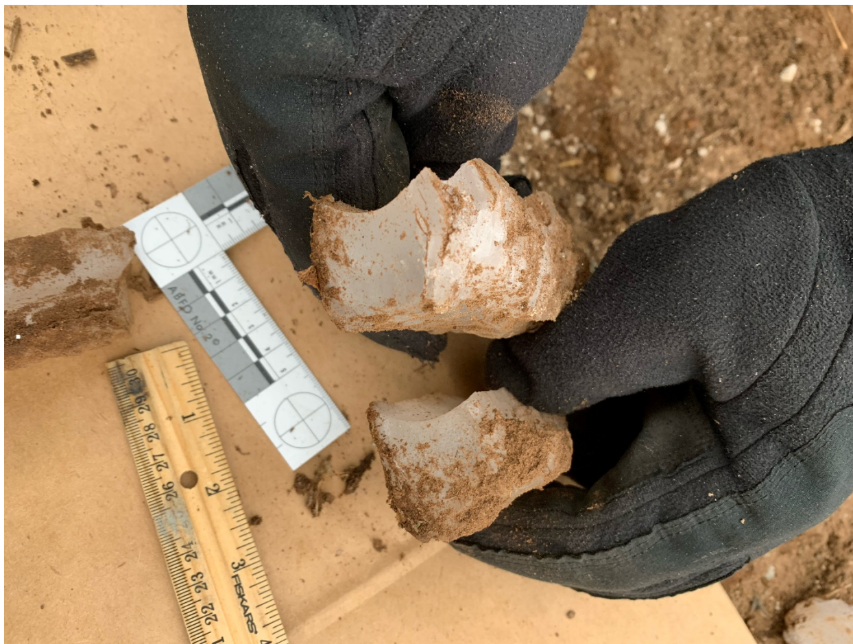
Figure 23 – Ice found near the accident aircraft
