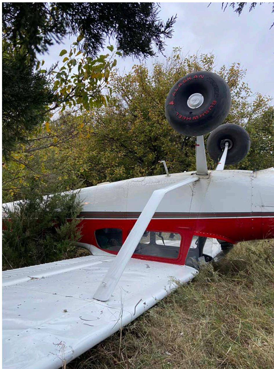
Photo 3 – Inverted N5910A. Note bent wing strut and buckled skin underneath left wing (Ian Alumbaugh photo)
