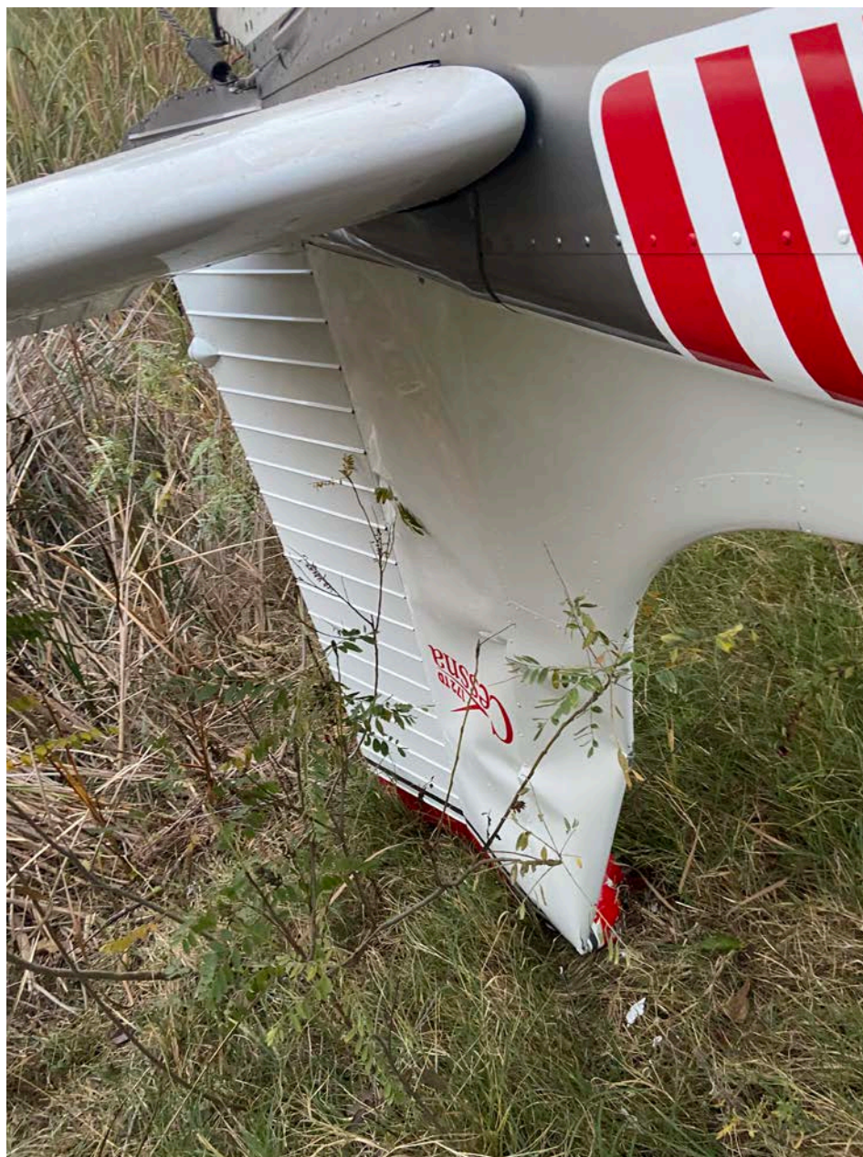
Photo 6 – Crushed and buckled vertical stabilizer (Ian Alumbaugh photo)
