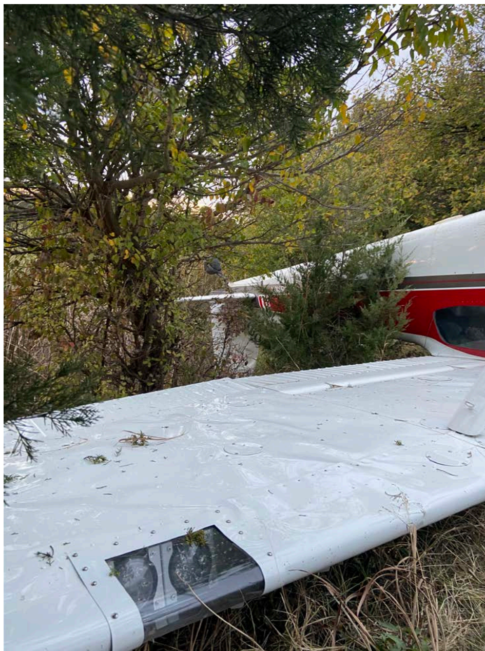
Photo 4 – Closer view of left wing's buckled skin (Ian Alumbaugh photo)
