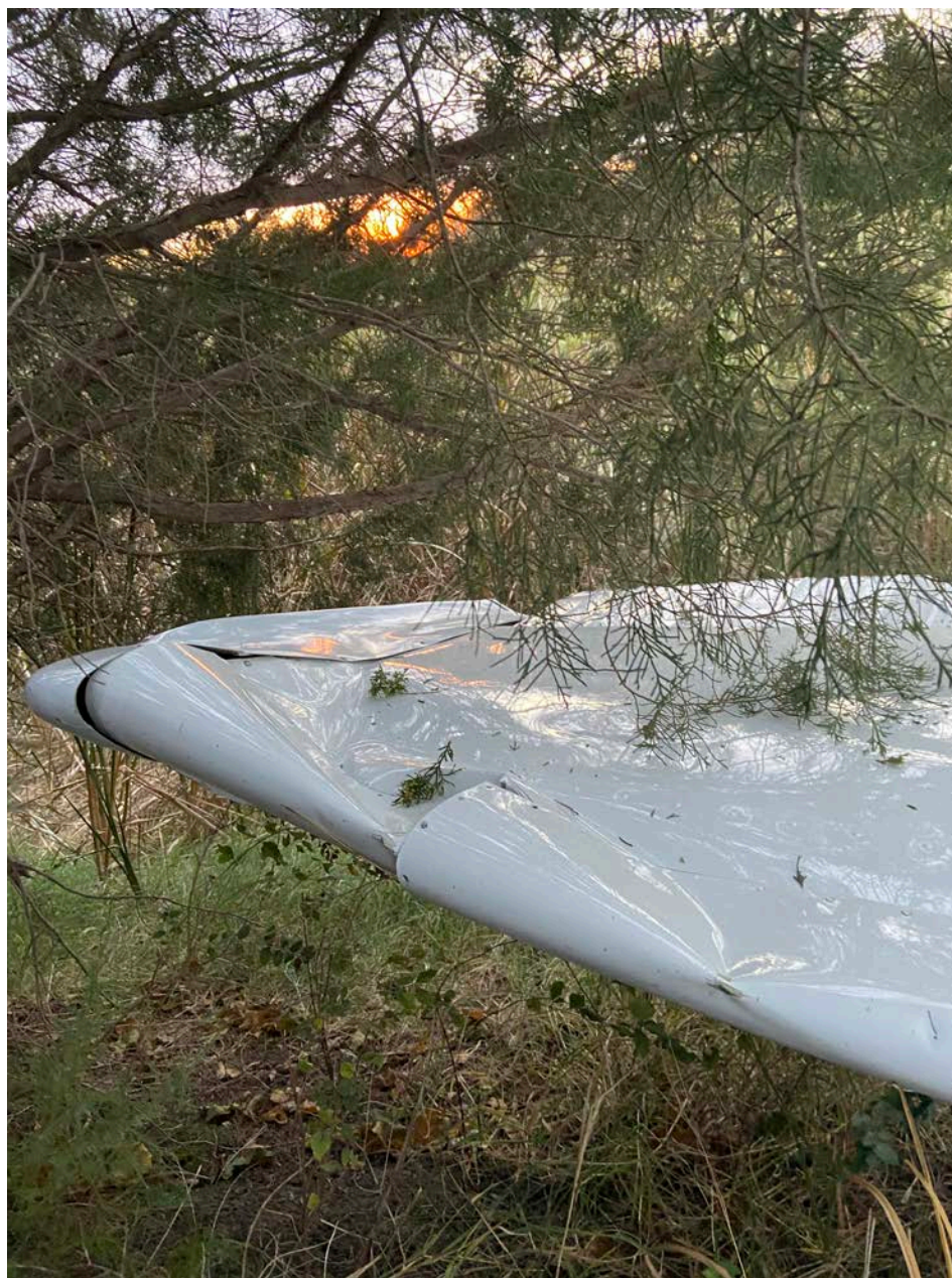
Photo 5 – Damage to left wing tip and leading edge (Ian Alumbaugh photo)
