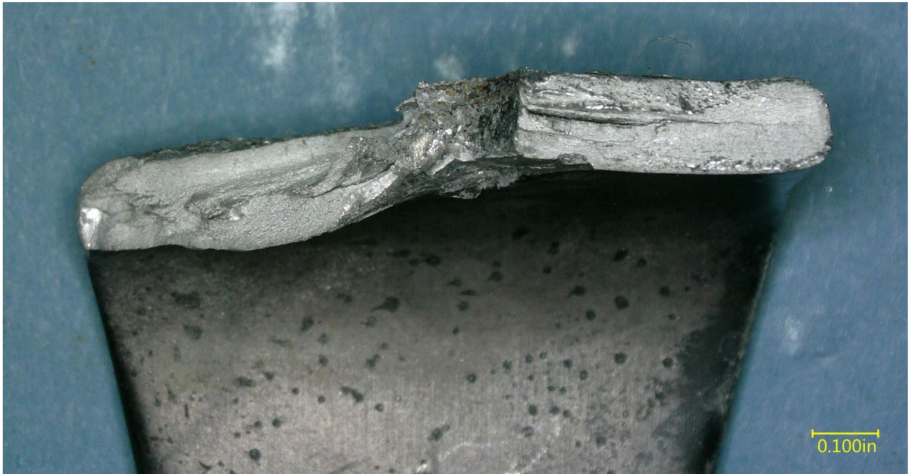
Figure 9 – View of one of the mating faces of the fractured bracket.
