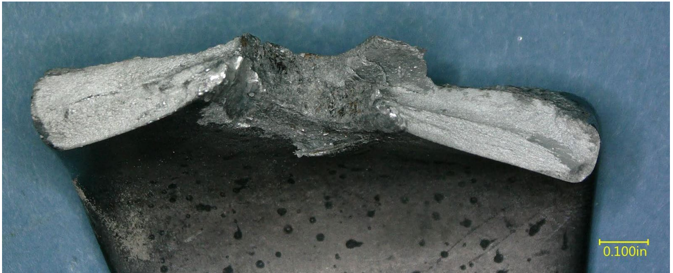
Figure 11 – View of the mating bracket fracture surface opposite that shown in Figure 9.
