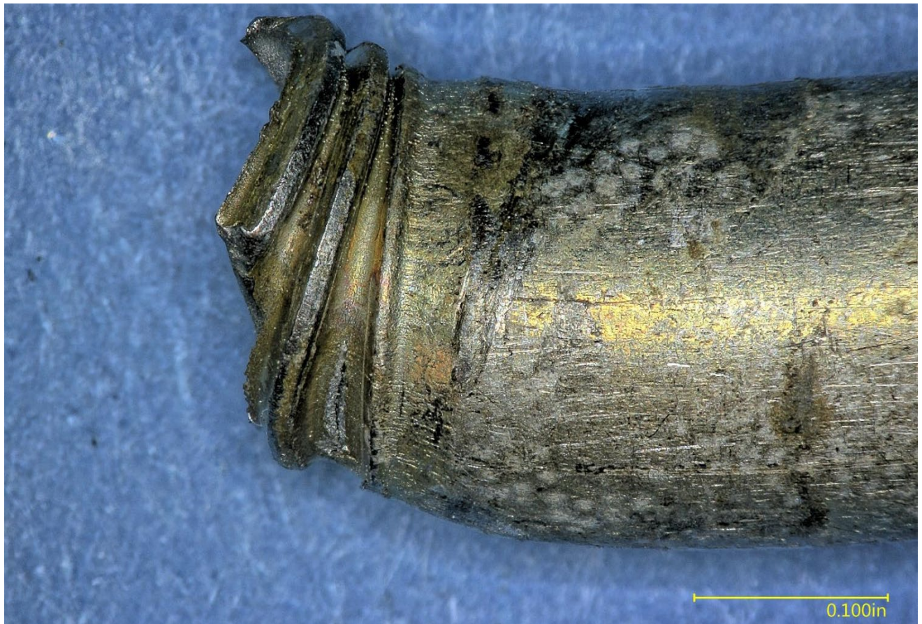
Figure 17 – View of the fractured bolt, from the side.
