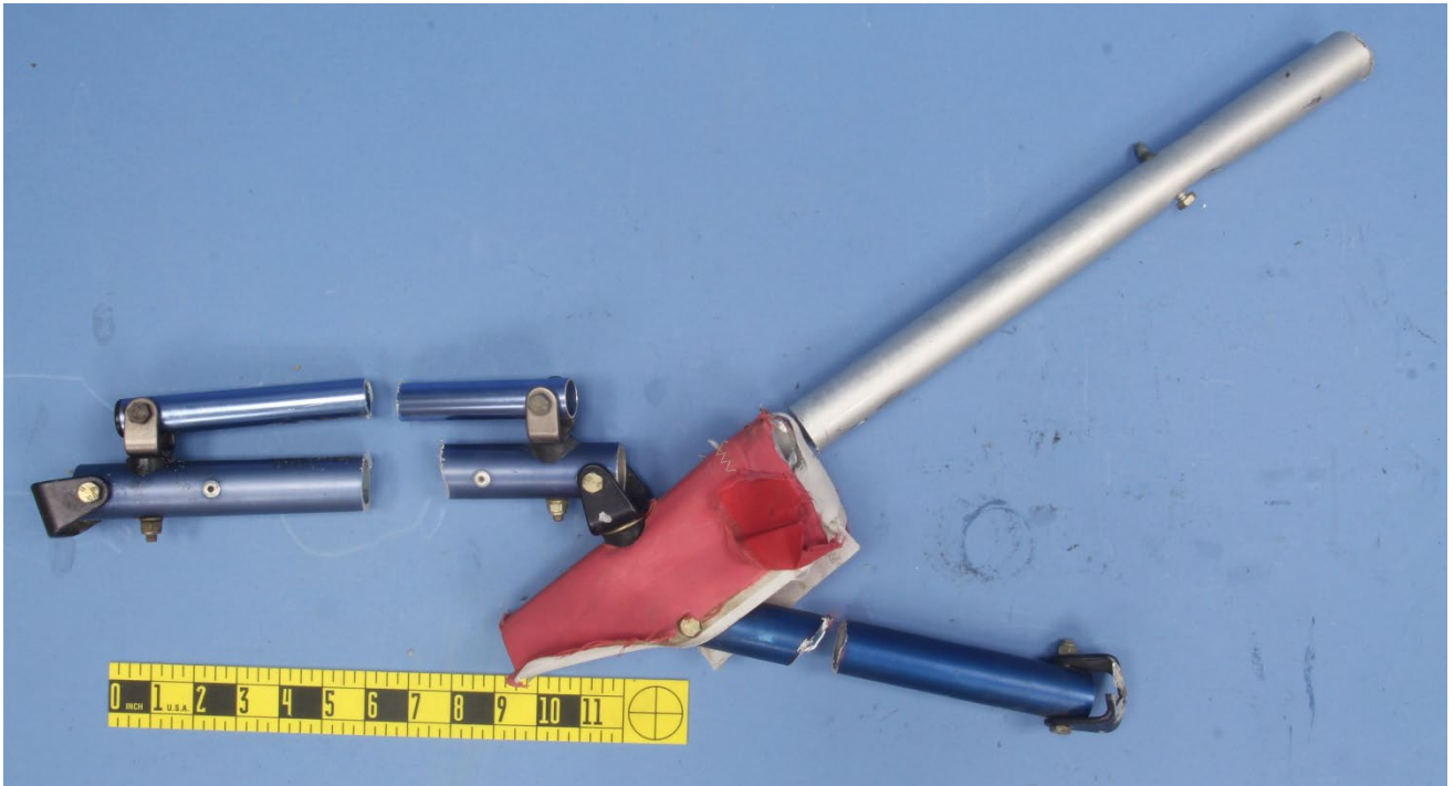
Figure 1 – The fractured structural support sectioned components, as received.
