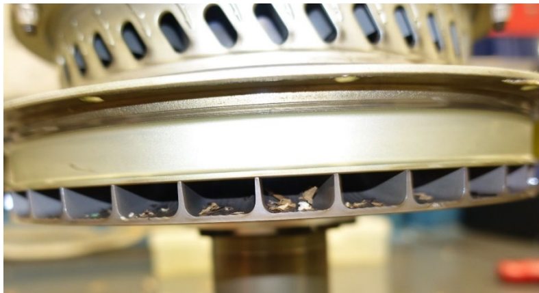
Photo 12- Centrifugal Compressor Exducer Debris Accumulation
