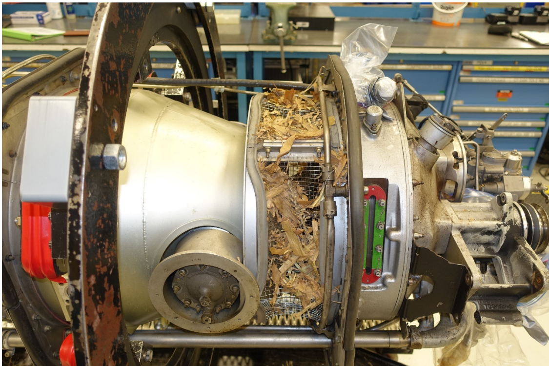
Photo 5- Corn Stalk Material Collected on the Inlet Screen
