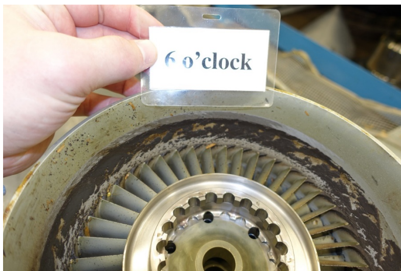
Photo 13- Axial Compressor Stator Case Debris Buildup and Rub Marks
