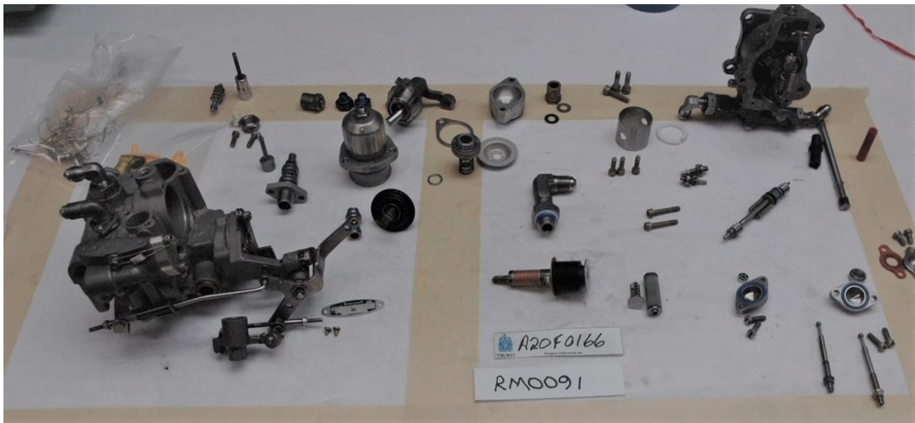
Photo 17- Fuel Control Unit, Partially Disassembled (Photo Courtesy of PWC)
