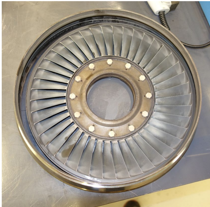
Photo 8- 2 nd Stage Power Turbine Nozzle
