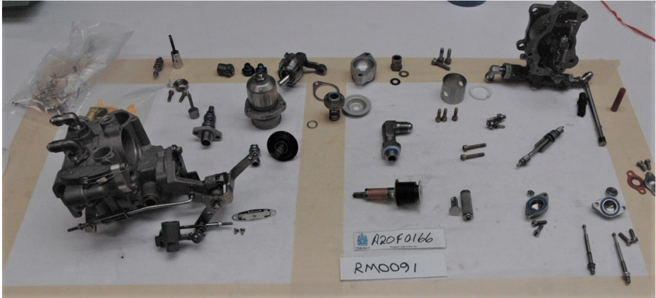
Figure 6 FCU partially disassembled
