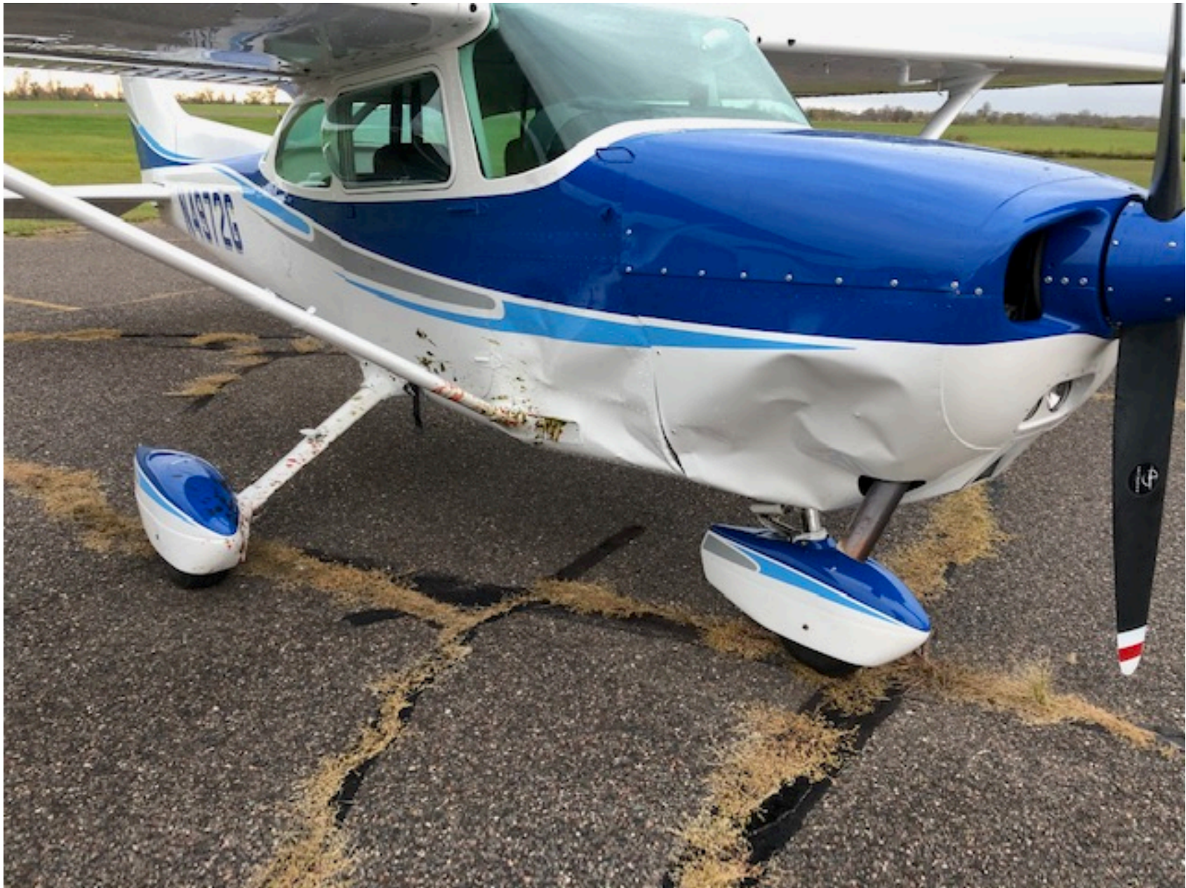
Photo 1 – Substantial Damage to Forward Fuselage
