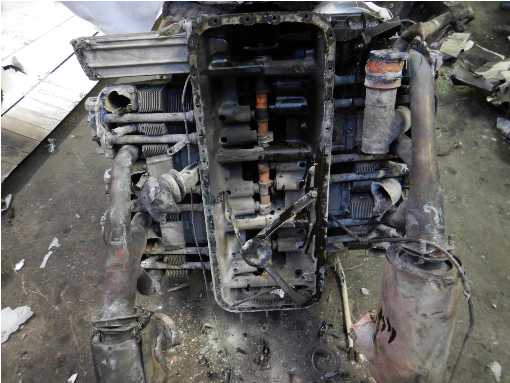
Photo 8 – Bottom of engine with oil sump pan removed
