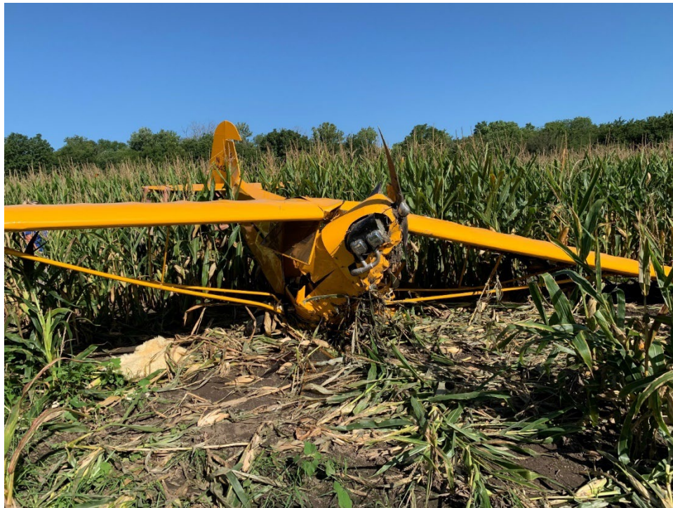
Figure 6: Overall Crush damage to Forward Fuselage and Engine
