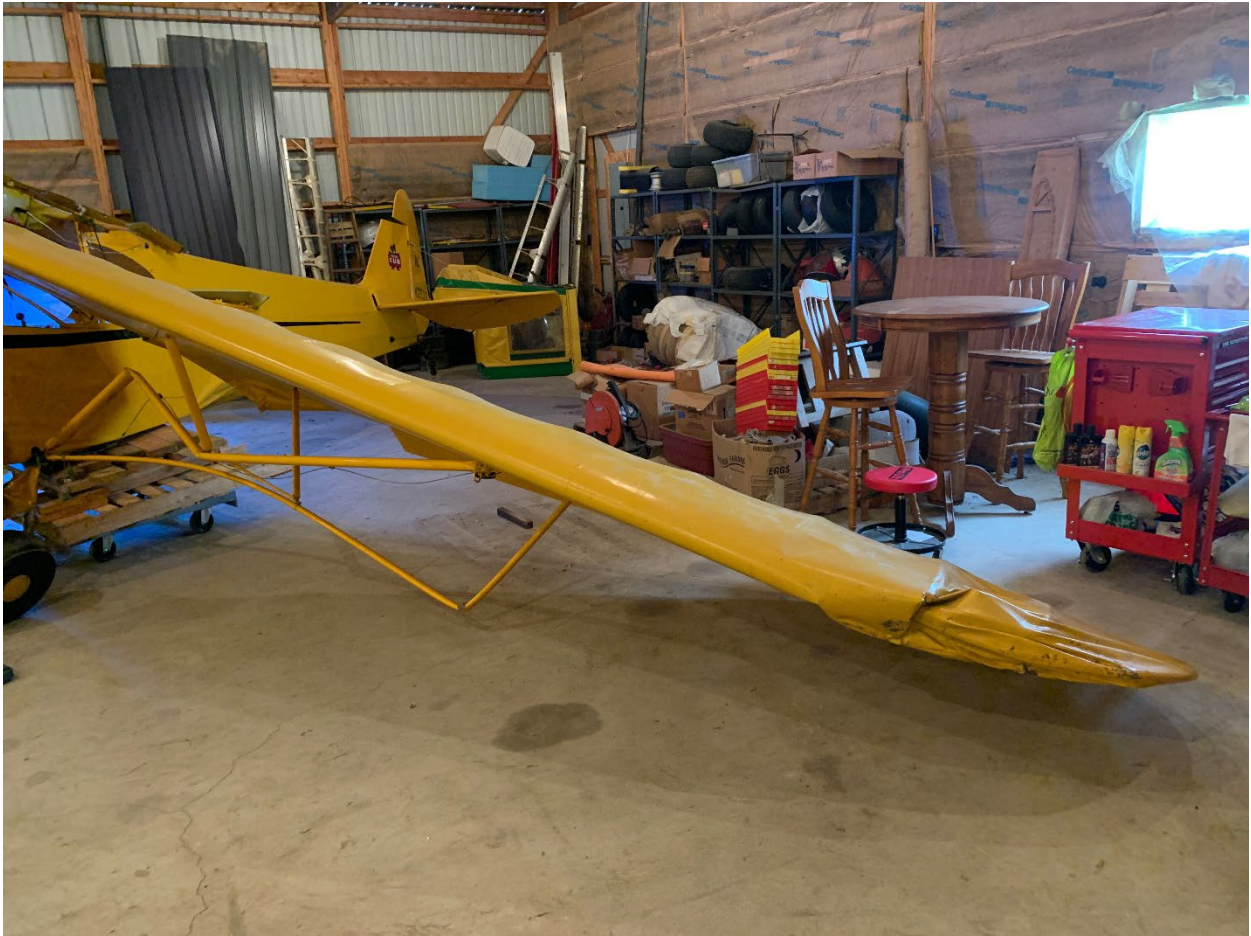
Figure 5. Left wing showing tip damage. (NTSB Photo)
