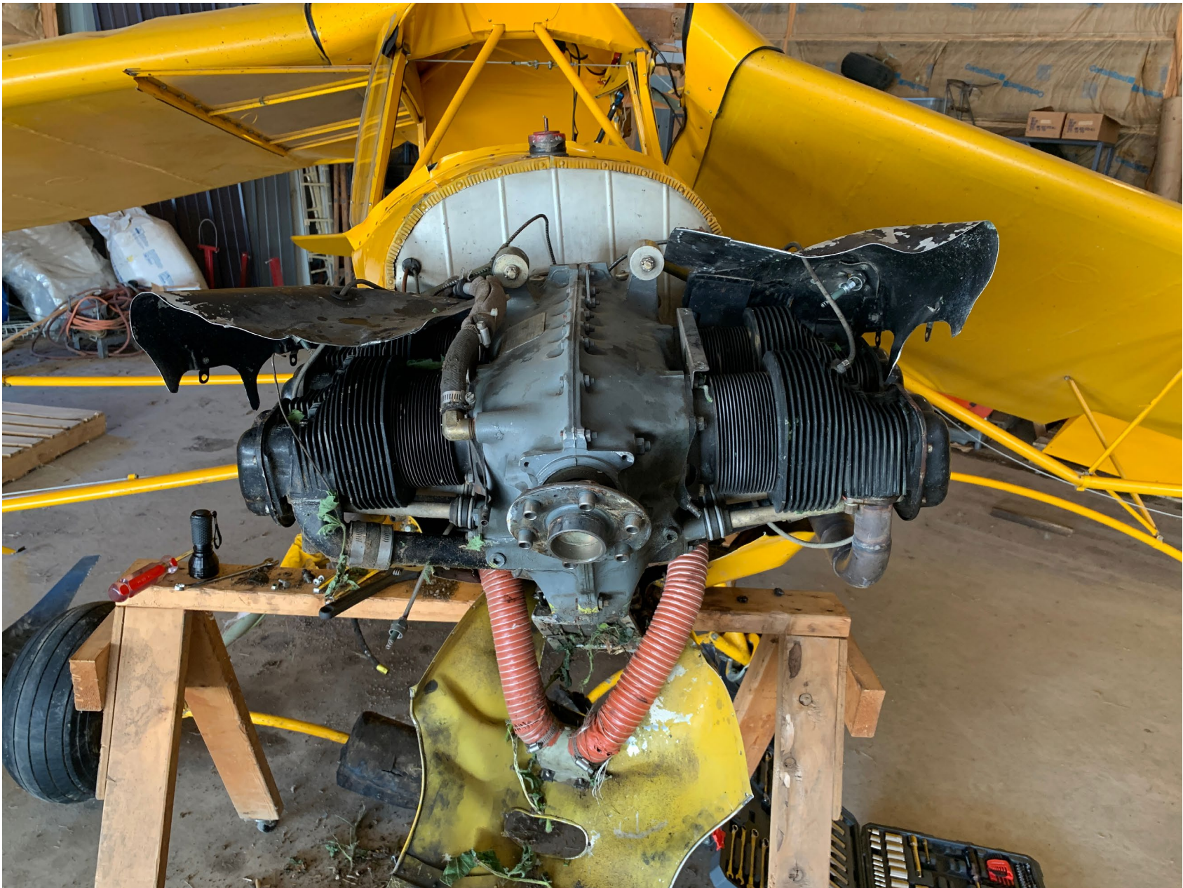
Photo 7 – Front view of engine during examination (NTSB Photo)
