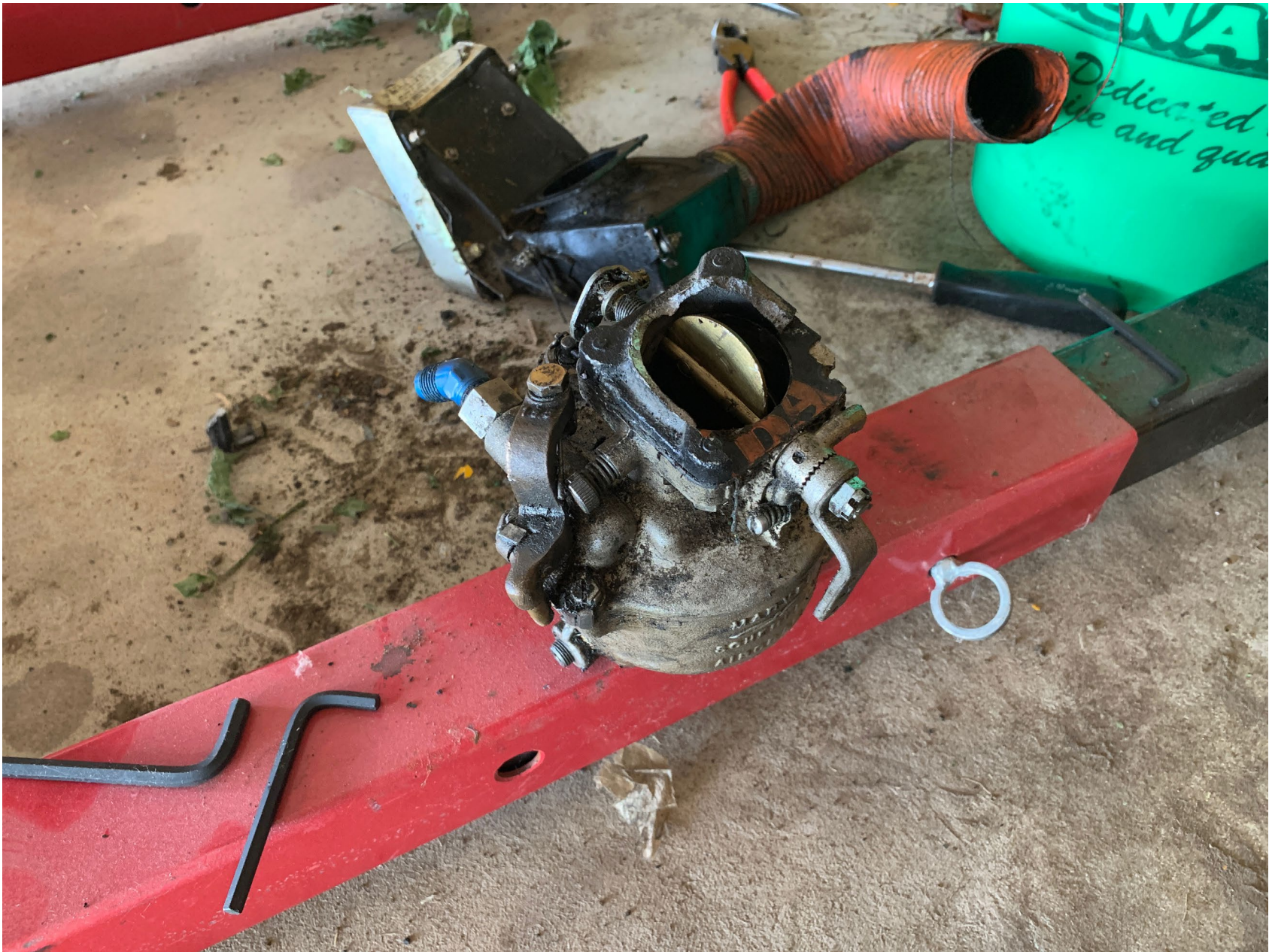
Photo 6 – View of carburetor after removal from airplane (NTSB Photo)
