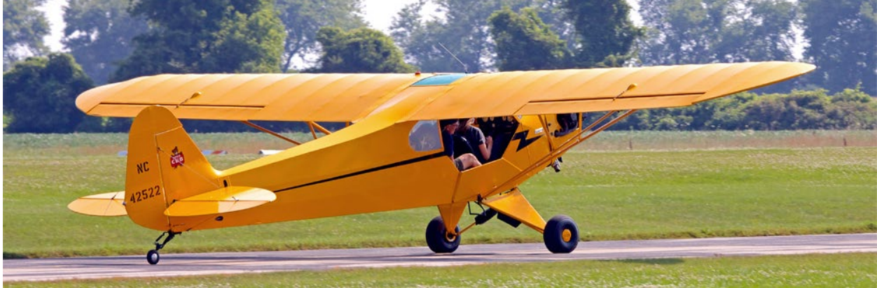
Figure 1. Pre-accident photo of N42522 found on airpigz.com 1 . In this photo the door is in a lowered and locked position, however that was not the configuration in the accident aircraft. Note that in the photo the side of the airplane is open, and the lower door can be seen in the down and secured position for flight.
