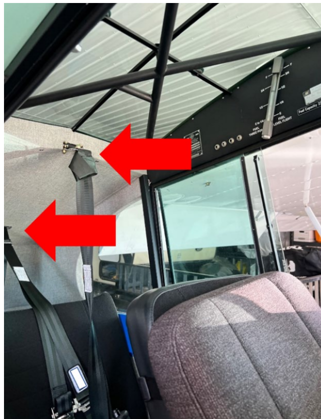
Figure 9. Mounting position for a set of upper torso restraints in an exemplar Piper Cub.
