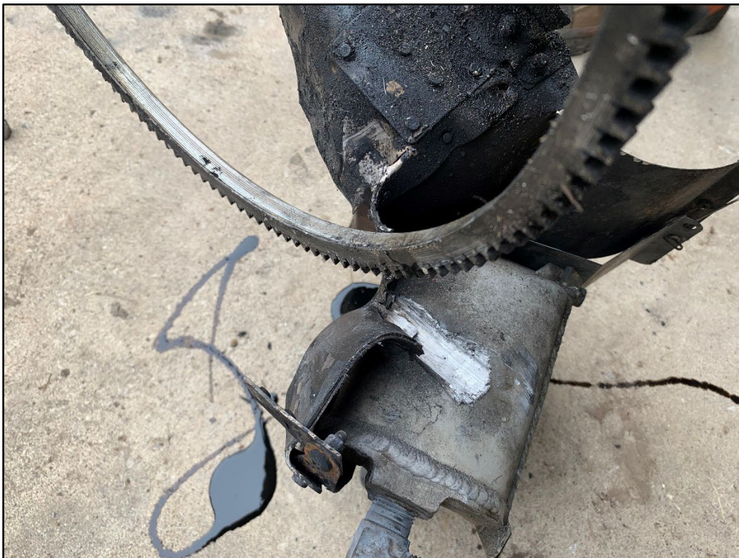
Figure 16. Starter ring gear gouge on the oil cooler body
