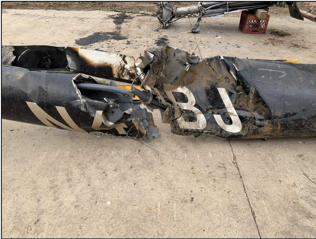
Figure 9. Tailboom boom separation about midspan
