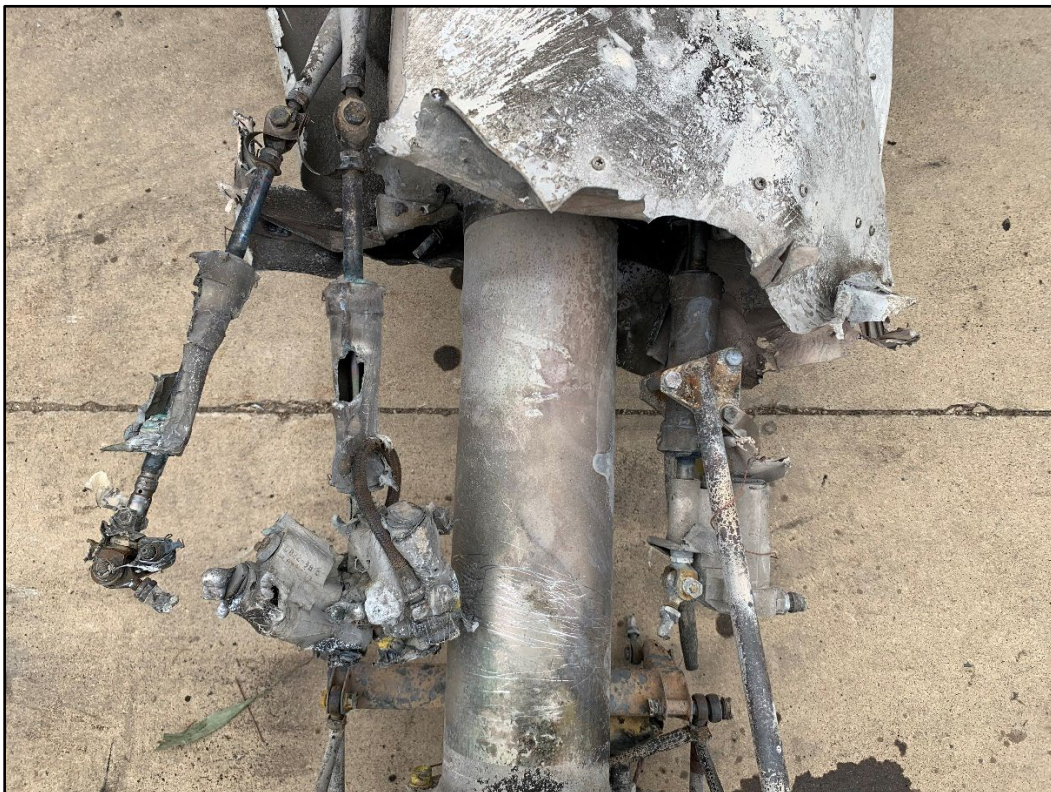
Figure 6. Hydraulic flight control actuators
