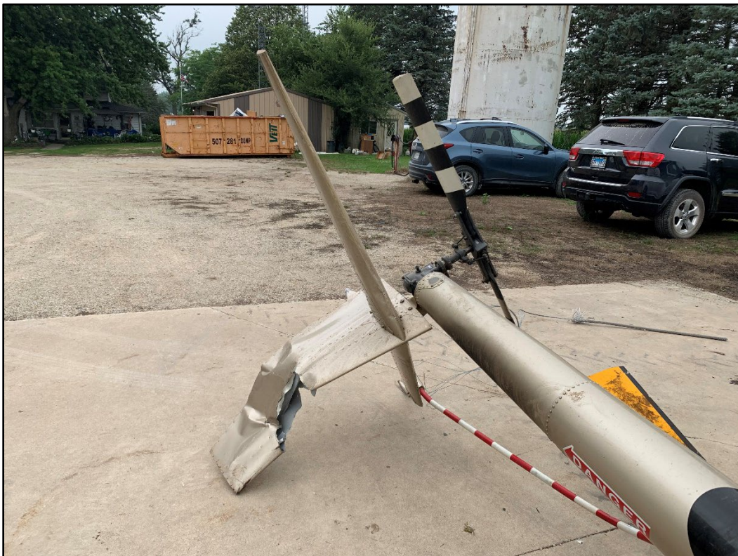
Figure 8. Aft section of tailboom
