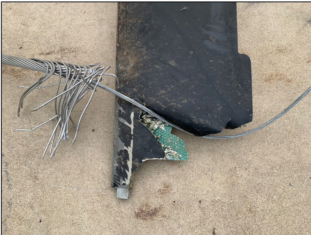
Figure 11. Main rotor blade fracture with the severed power transmission line
