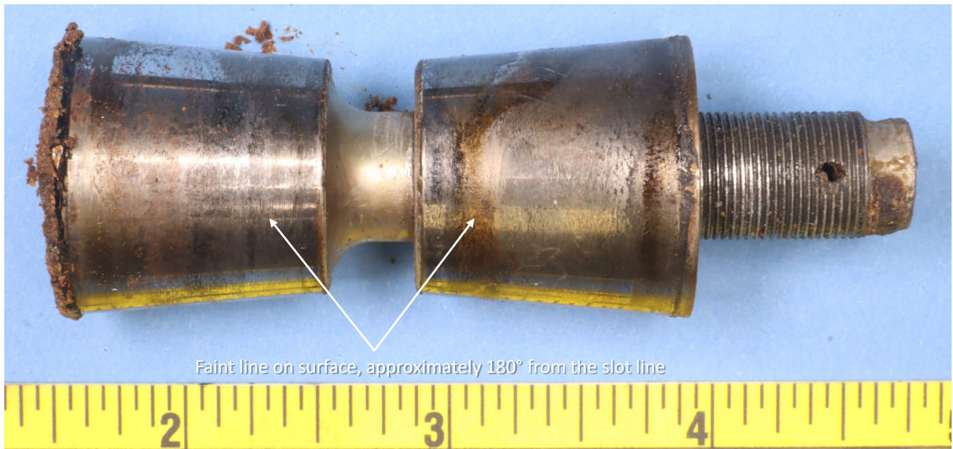
Figure 9 Image showing faint witness marks on the tapered portion of the retention bolt and the tapered plug.
