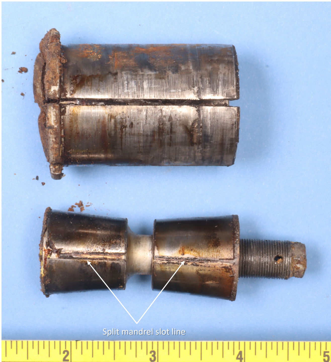
Figure 8 Image of the split mandrel, the retention bolt and tapered plug. A deposit of brittle coating is present on the ends of the parts. Witness marks on the tapered portion of the retention bolt and the tapered plug is from the slot in the split mandrel.
