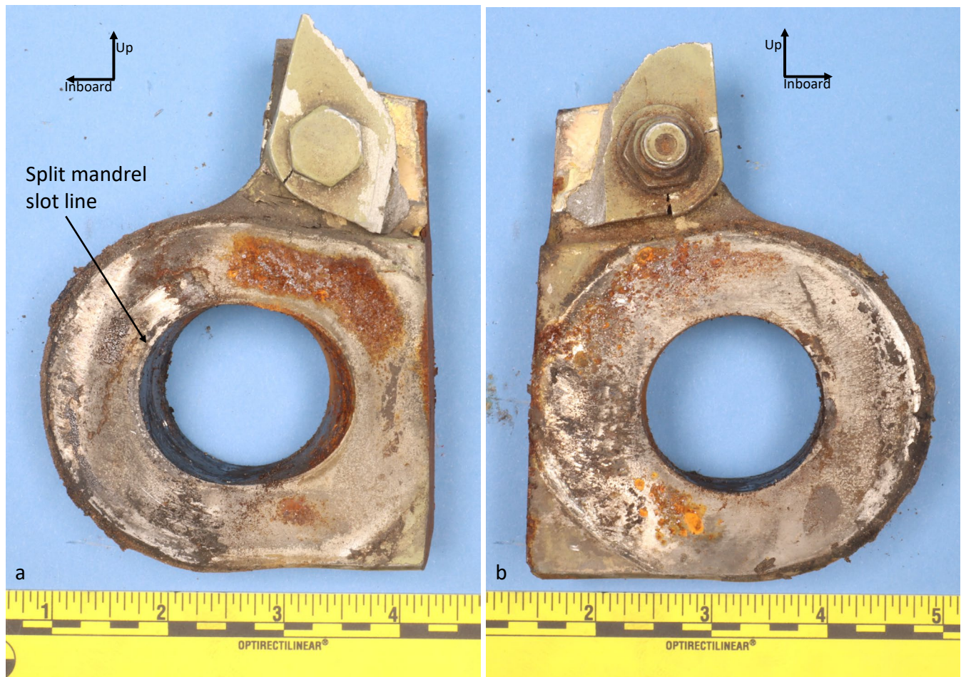
Figure 4 Images of the right outboard lower attachment fitting after disassembly from the lower yoke showing the aft (view a) and forward (view b) sides.
