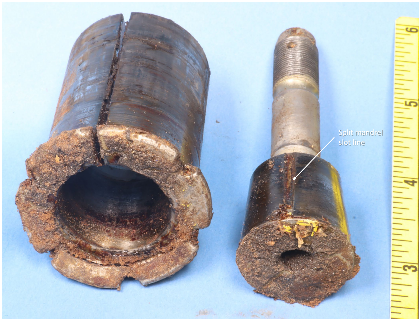
Figure 7 Image of the split mandrel and the retention bolt. A deposit of brittle coating is present on the ends of the parts. A witness mark on the tapered portion of the retention bolt is from the slot in the split mandrel.
