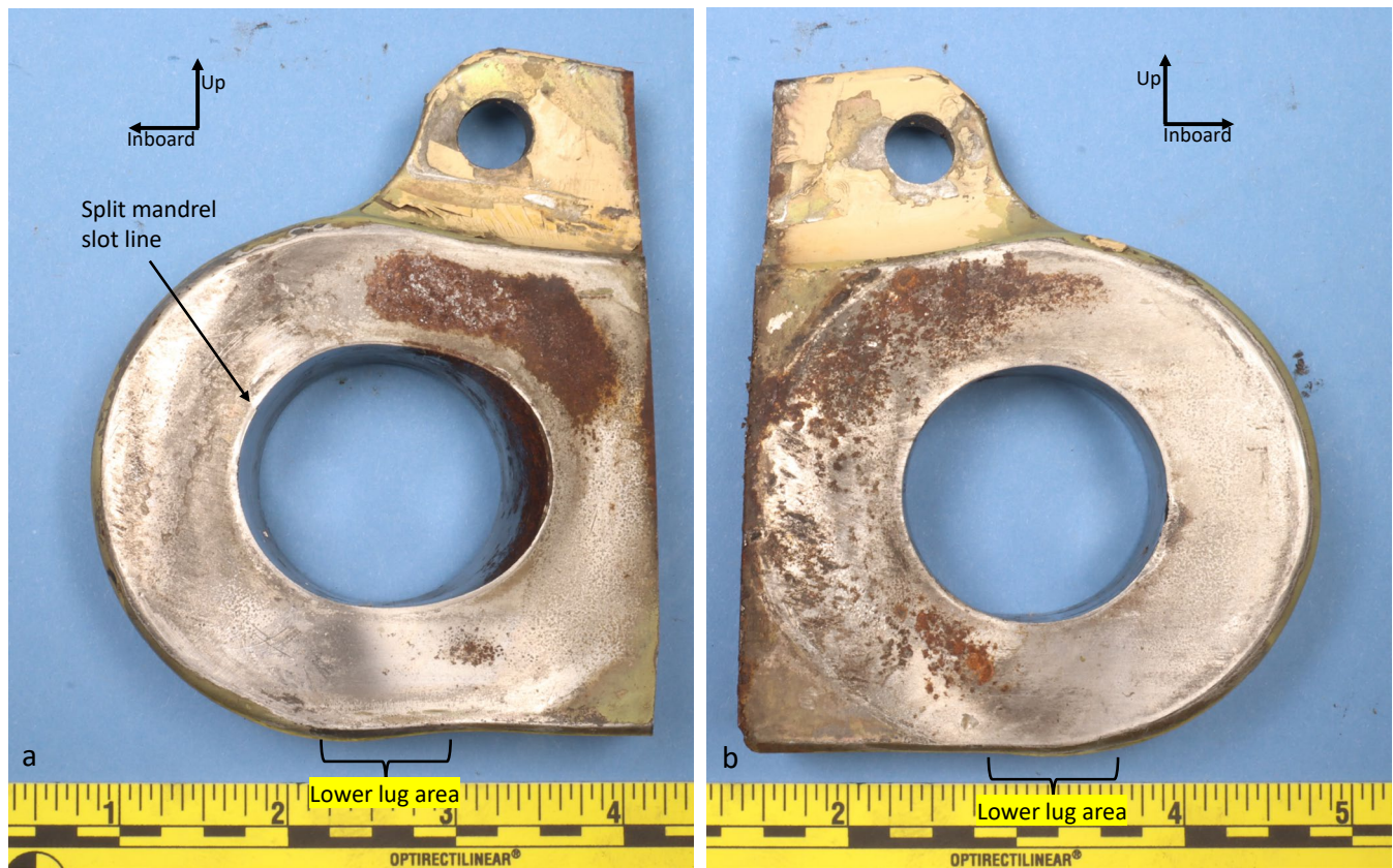
Figure 11 Images of the right outboard lower attachment fitting after cleaning in acetone showing the aft (view a) and forward (view b) sides.
