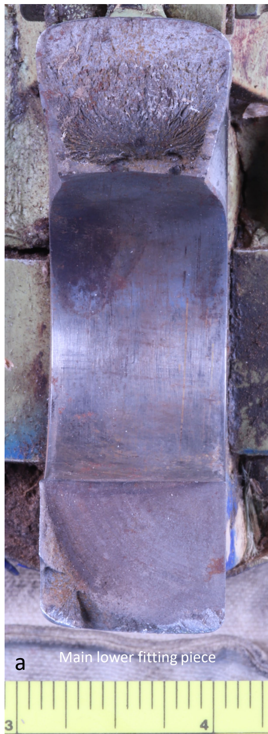
Figure 11 Close views of the as-received fracture faces and bore surfaces on the lower attachment fitting and the separated lug piece. Corrosion product deposits are evident on the bore surface of the separated lower fitting piece.
