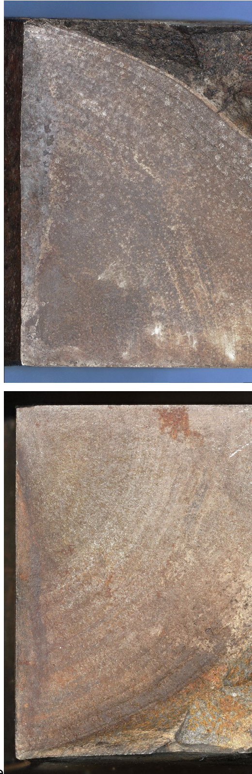
Figure 19 Digital microscope images of both halves of the lower lug fracture surfaces showing a stained region just below the bore (see Figure 20 for the same images with annotations). The images were acquired under normal imaging conditions with oblique lighting.
