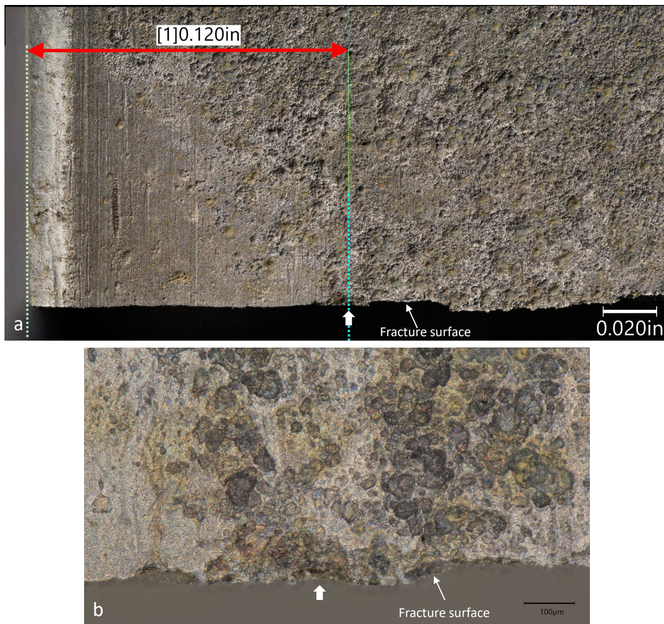
Figure 40 Closer digital microscope images (HDR) of the bore surface in Figure 39b after 240 minutes of Evapo-Rust immersion followed by brush cleaning to remove corrosion product deposits on the surface. Under the corrosion product layer, material loss by corrosion is evident and pits cover the surface. Pit 1 is marked with an unlabeled white arrow.
