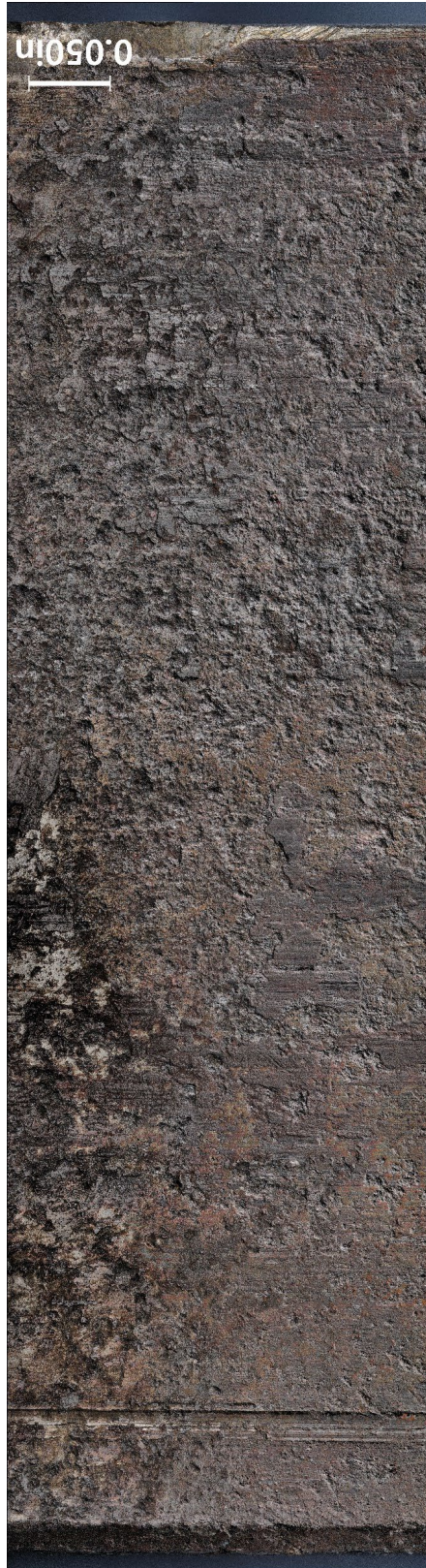
Figure 16 Digital microscope view across with width of the lug bore for the separated lower fitting piece (see Figure 15 for location) revealing corrosion product scale and pits. A circumferential score mark is also present.
