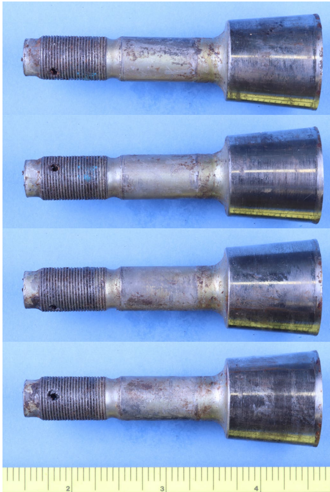
Figure 55 Views of the retention bolt from the expansion mandrel assembly in the as-received condition and after cleaning in acetone with ultrasonic agitation.
