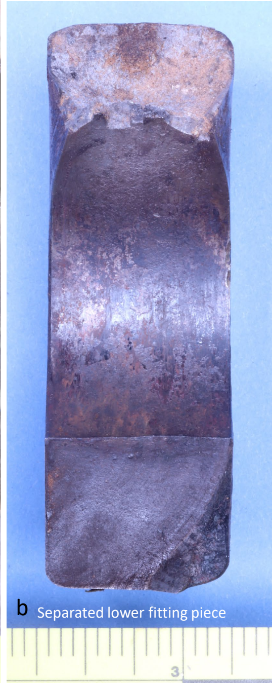
Figure 11 Close views of the as-received fracture faces and bore surfaces on the lower attachment fitting and the separated lug piece. Corrosion product deposits are evident on the bore surface of the separated lower fitting piece.
