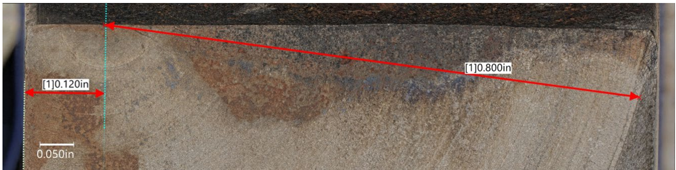
Figure 36 Digital microscope image (HDR) showing the location of the initiating pit feature relative to the edge of the lug. The overall length of the fatigue crack was also measured from the origin (Pit 1) to the approximate terminus. Image taken after 60 minutes immersion in Evapo-Rust.
