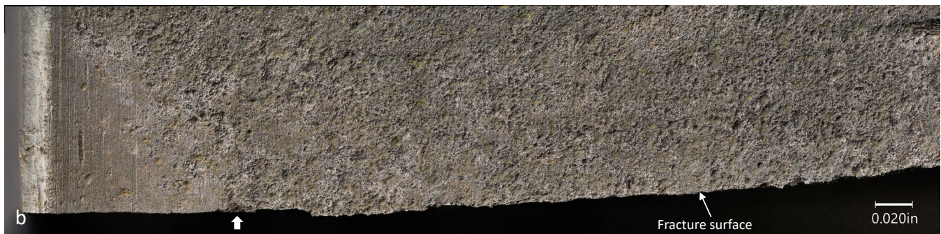
Figure 39 Closer digital microscope images (HDR) of those in Figure 38. View a is in the as-received acetone-cleaned condition. View b is the surface after 240 minutes of Evapo-Rust immersion followed by brush cleaning to remove corrosion product deposits on the surface. Under the corrosion product layer, material loss by corrosion is evident. Pit 1 is marked with an unlabeled white arrow.
