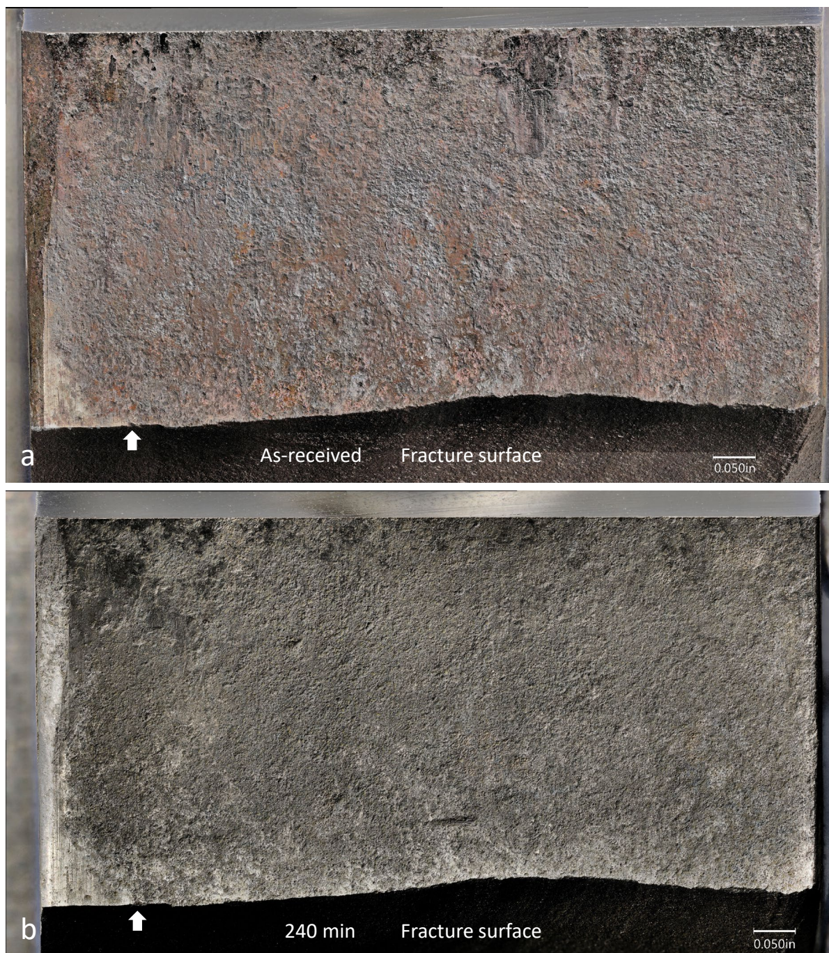
Figure 38 Top down digital microscope images (HDR) of the surface of the lug bore in the vicinity of the fracture face. The unmarked white arrow in the images is the location of Pit 1. View a is in the as-received acetone-cleaned condition. View b is the surface after 240 minutes of Evapo-Rust immersion followed by brush cleaning to remove corrosion product deposits on the surface.
