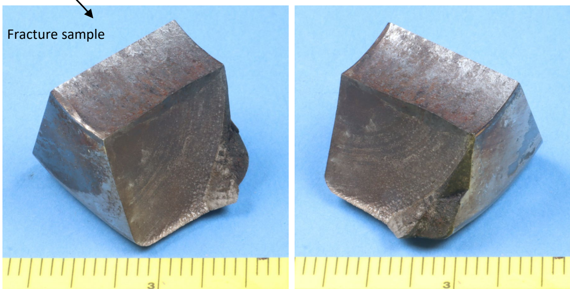
Sample with fracture to be progressively cleaned in Evapo-Rust®
