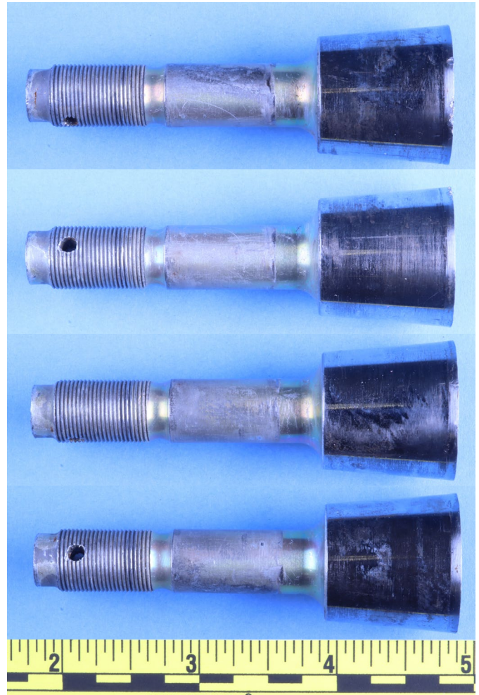
Figure 55 Views of the retention bolt from the expansion mandrel assembly in the as-received condition and after cleaning in acetone with ultrasonic agitation.
