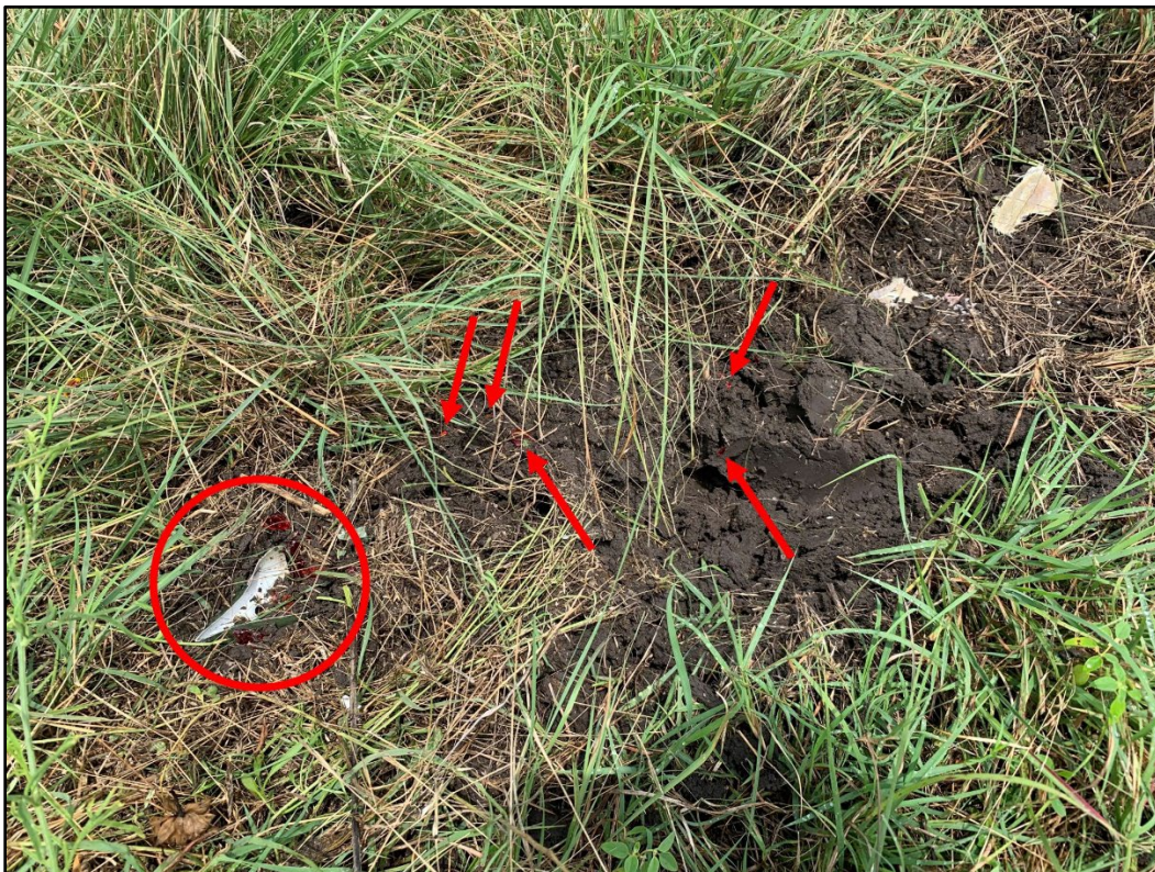
Figure 5 - Initial impact point with red navigation lens material from left wingtip
