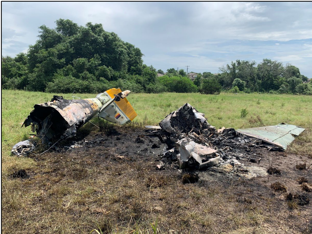
Figure 8 - Main wreckage, aft fuselage, and empennage
