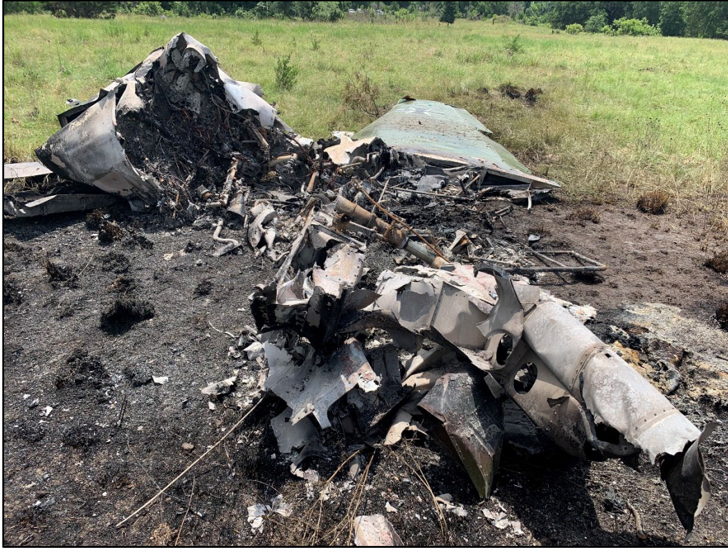
Figure 11 - Left wing and cabin
