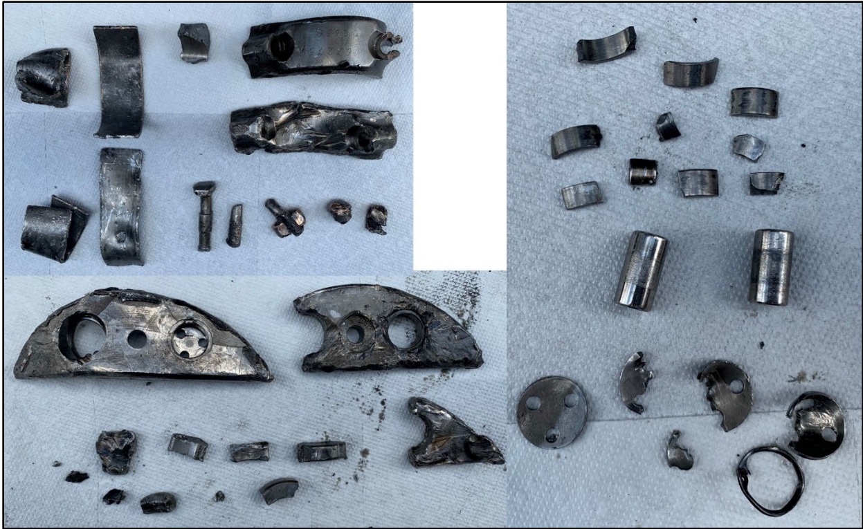
Figure 24 - Metal items recovered from inside engine during the examination
