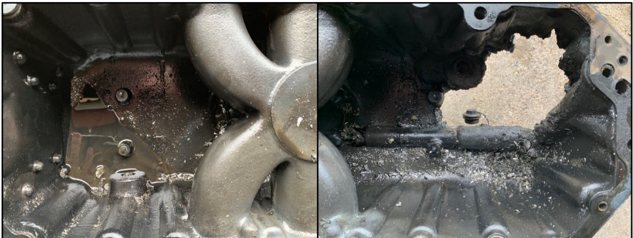
Figure 21 - Metal contamination found in the engine oil sump
