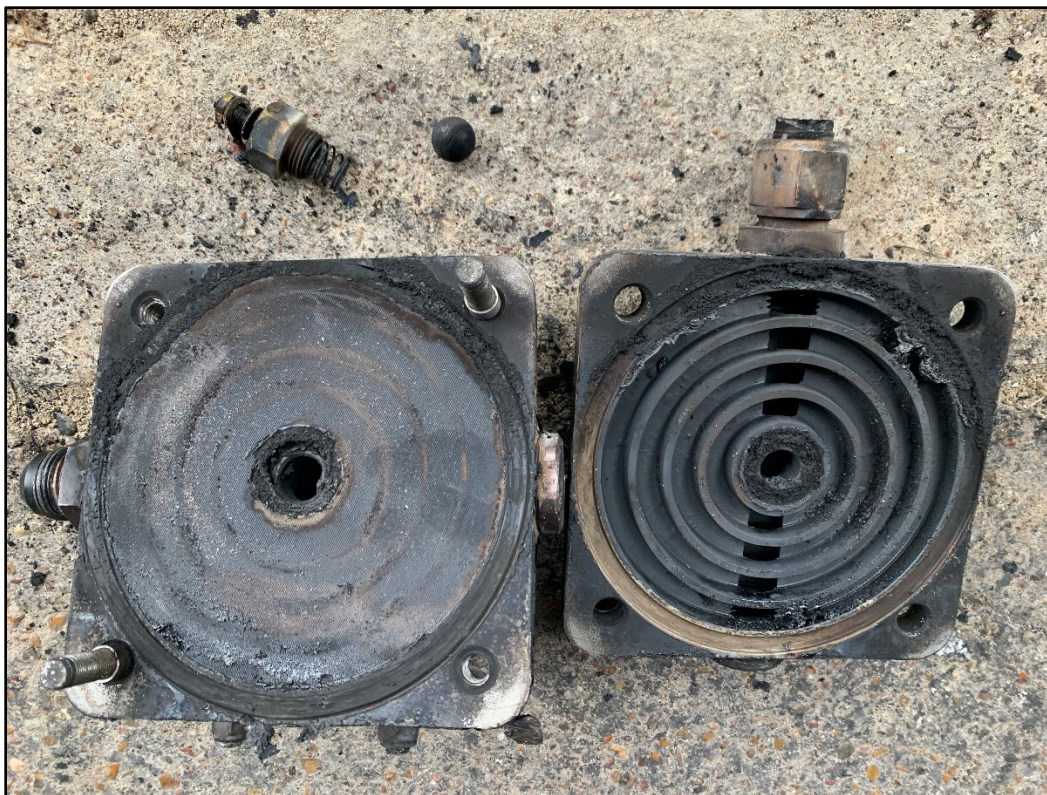
Figure 28 - Engine oil filtration assembly disassembled
