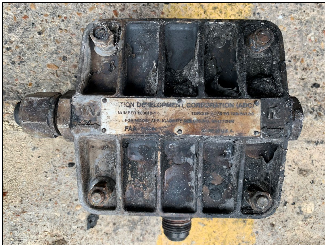
Figure 27 - Engine oil filtration assembly, p/n 600010-1
