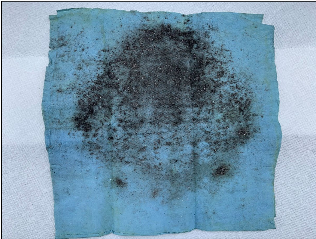
Figure 30 - Contamination collected from oil filtration screen 2 days before accident
