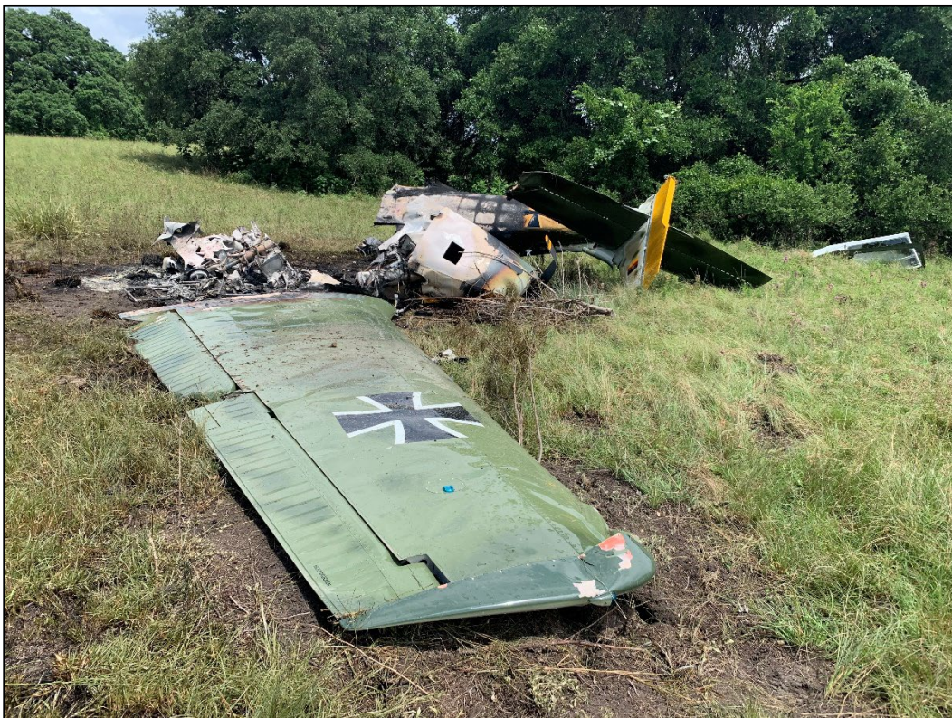
Figure 10 - Right wing, right aileron, and right flap
