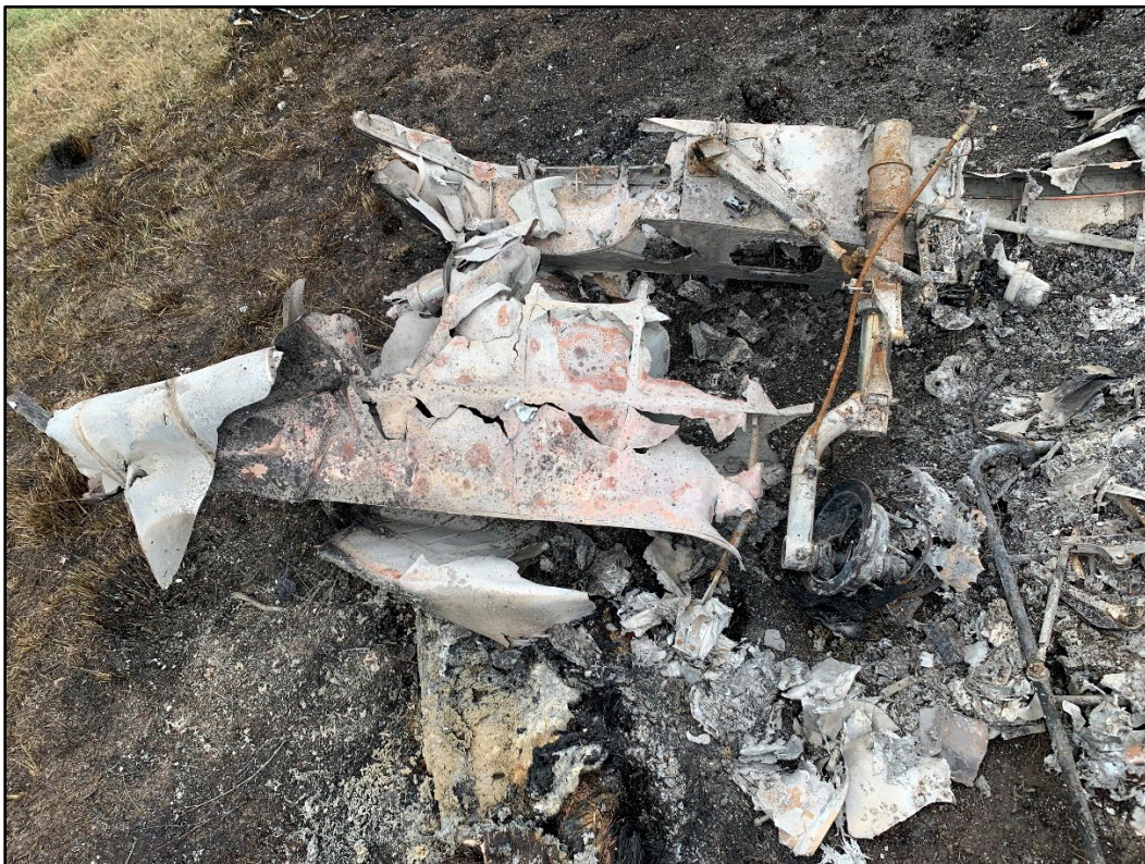
Figure 12 - Left wing spar, left flap, and left main landing gear
