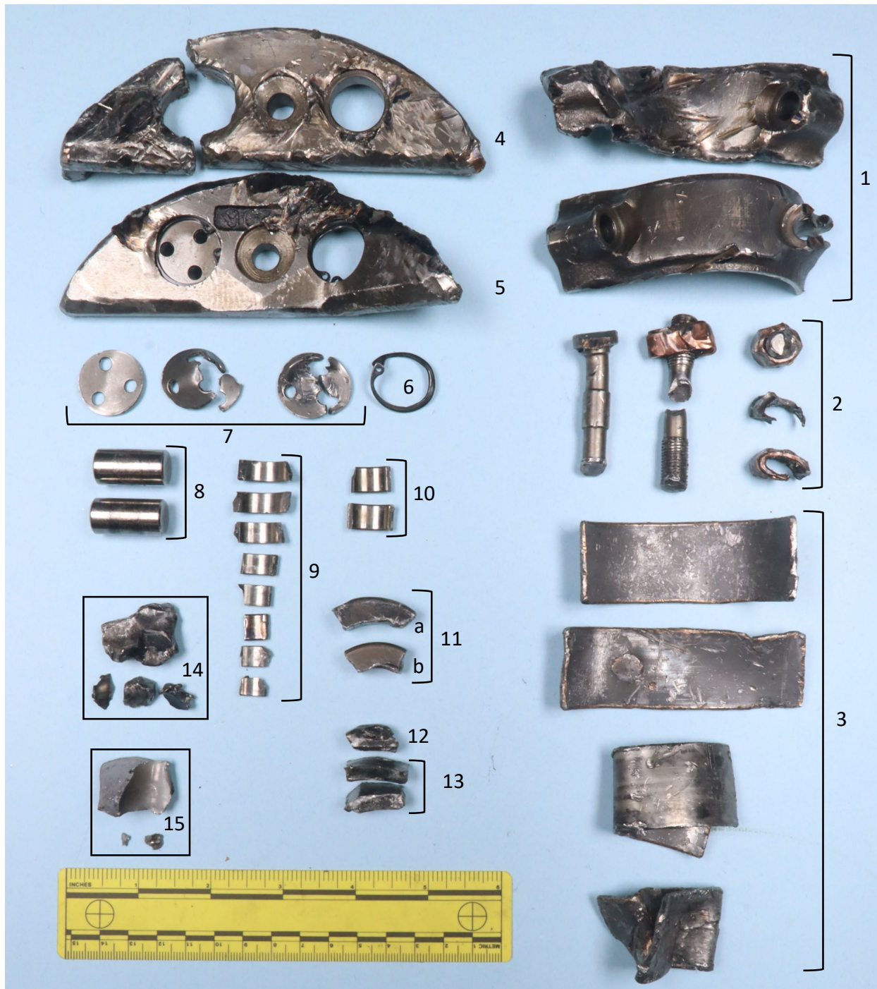
Figure 12. Image showing the pieces recovered from the engine after teardown. The pieces are approximately grouped according to their function. Table 1 provides a description of the pieces.
