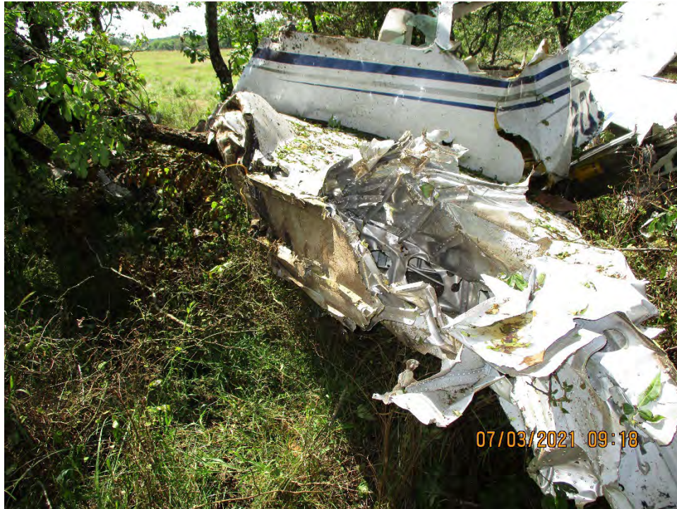
Figure 9: Left wing midspan fracture surface
