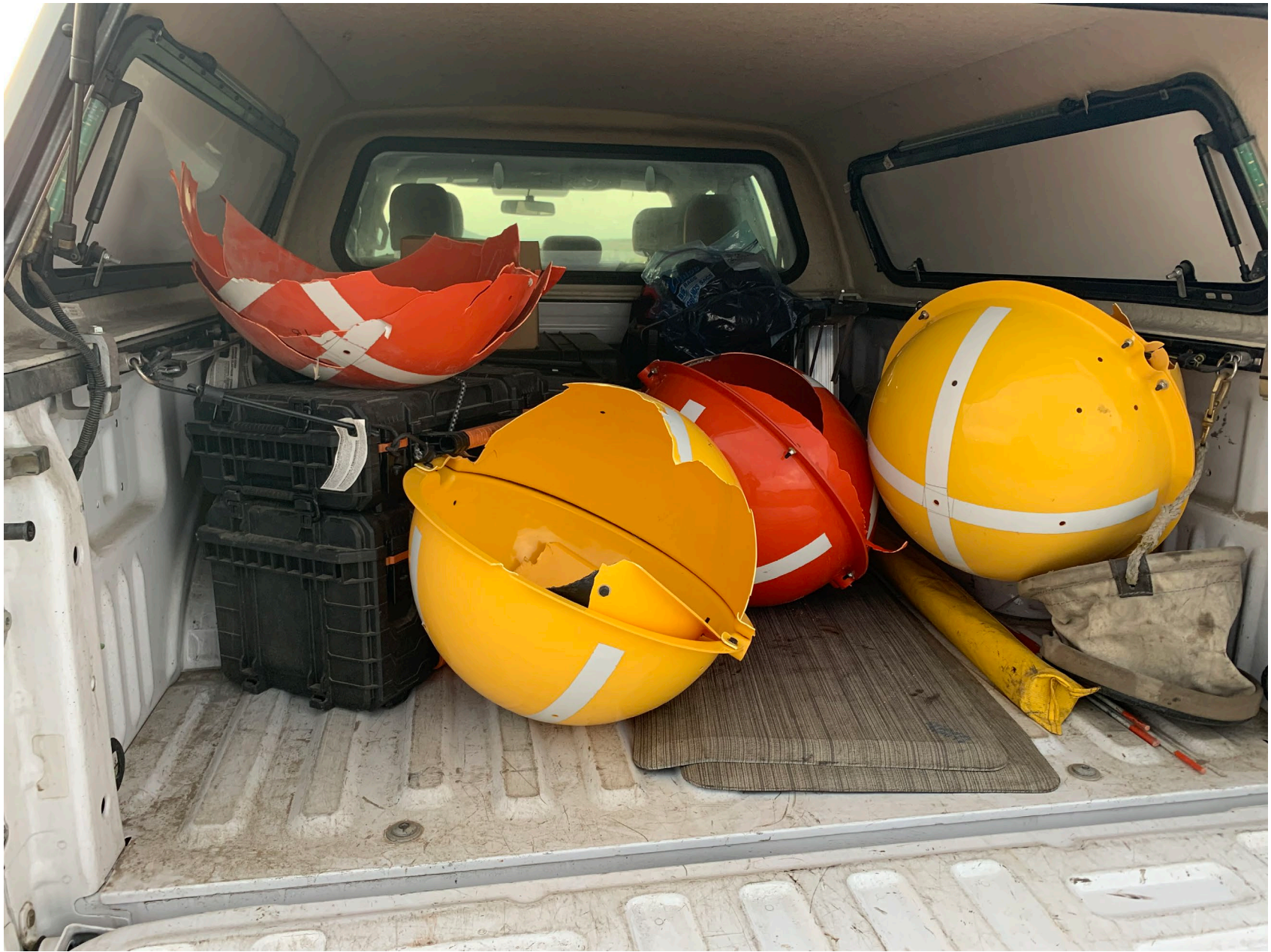
Photo 12 – View of the various recovered marker balls that were installed on the transmission static lines.
