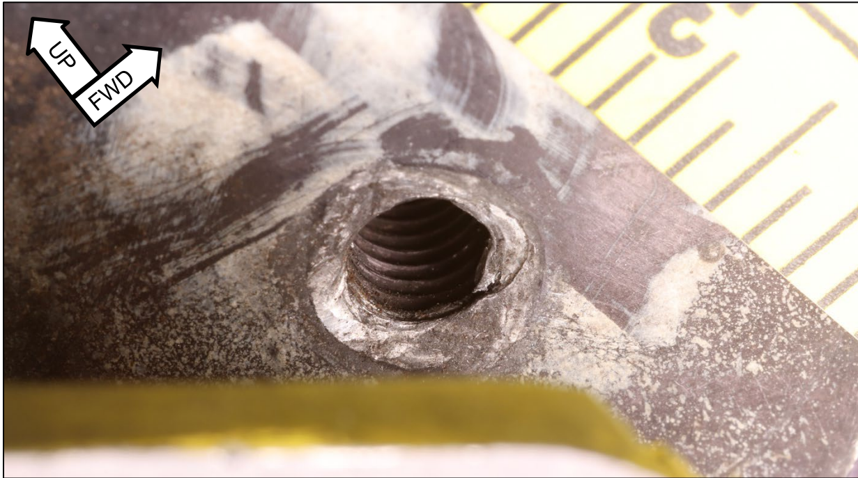
Figure 3. Intact threads in the left flap control attachment bracket associated with the missing flap control attachment bolt.
