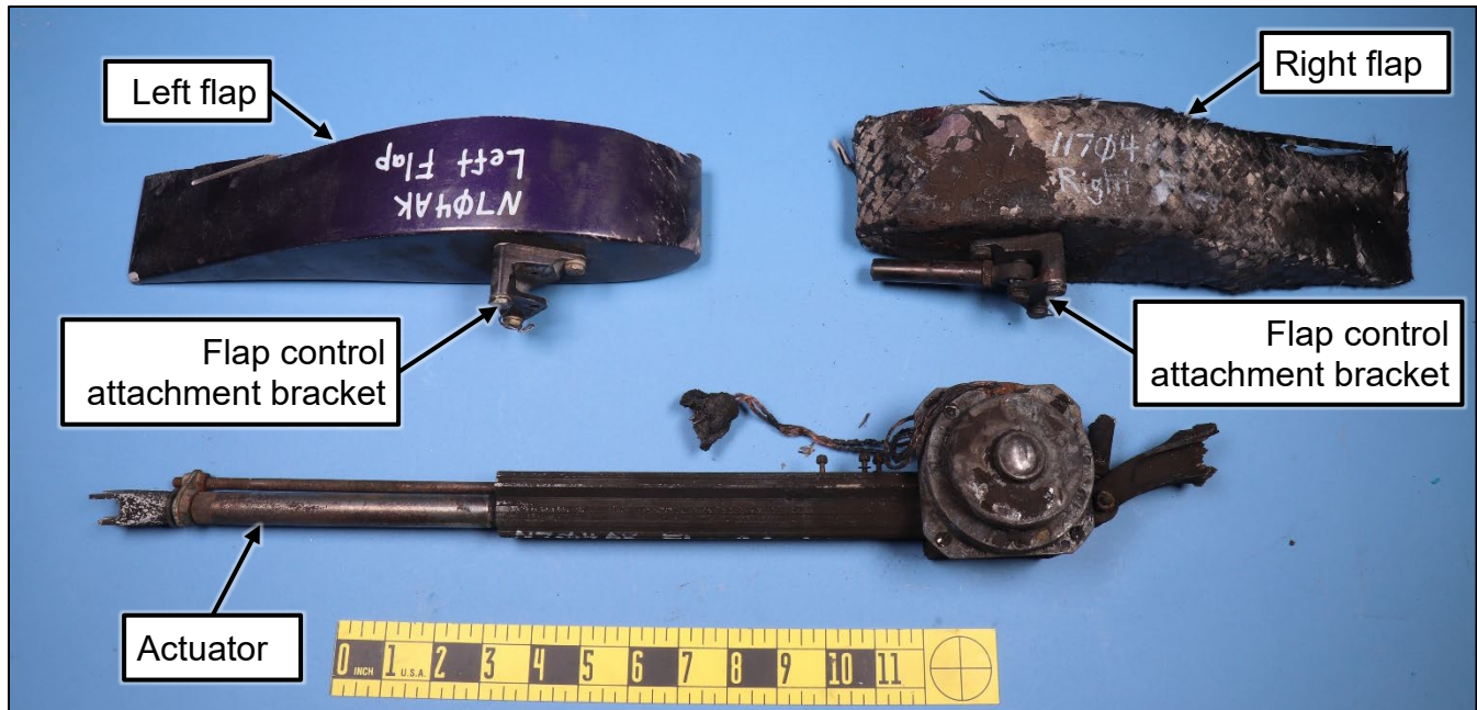
Figure 1. Overall view of the submitted flap pieces and the flap actuator.
