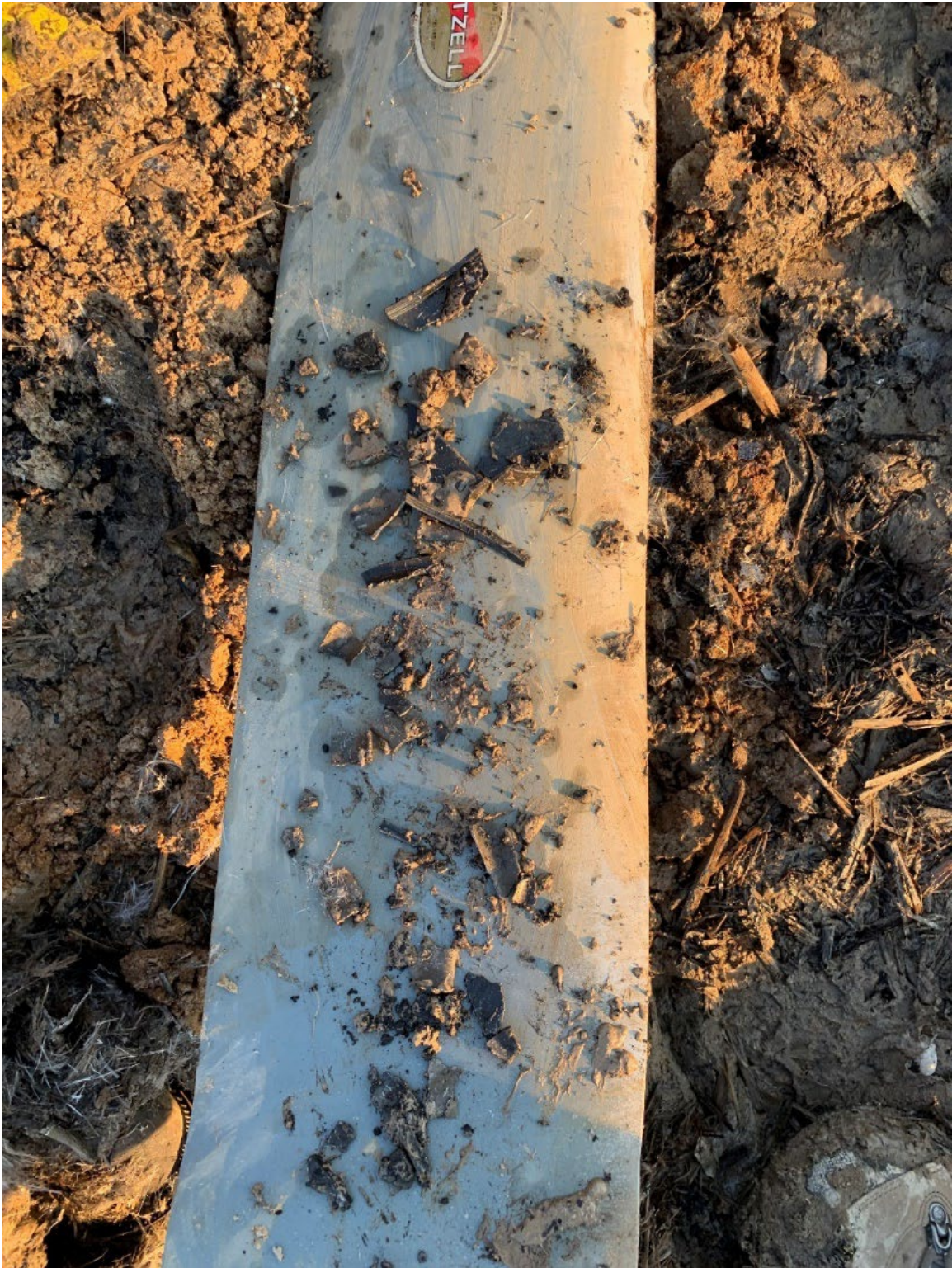
Figure 19: Power Turbine Blade Fragments removed from Exhaust.
