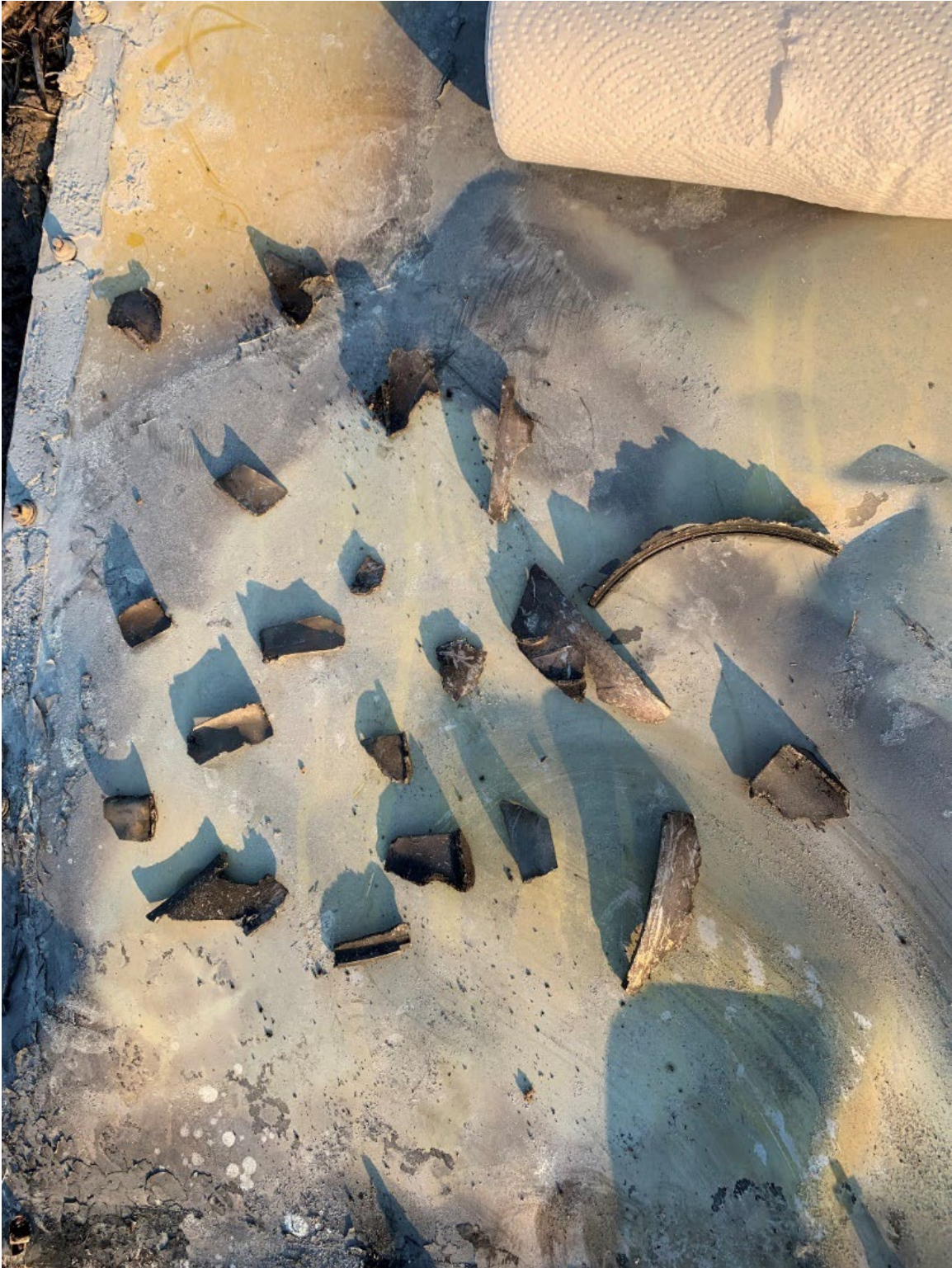
Figure 20: Fragments of Power Turbine Blades, Vane Ring, and Shroud.
