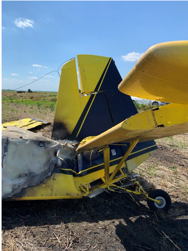
Figure 9: Bend in Empennage
