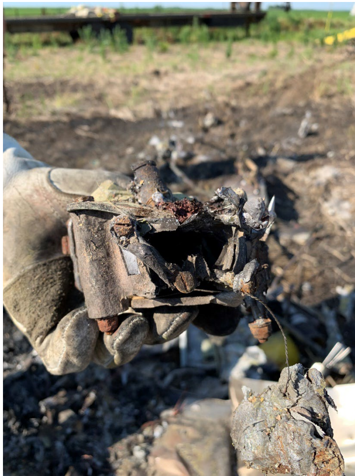
Figure 12: Fuel Control Valve
