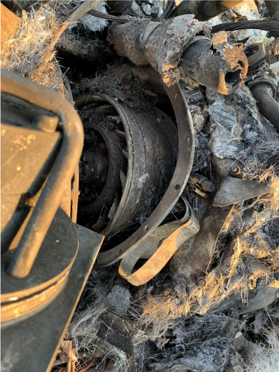
Figure 23: Housing Fracture at the Axial Compressor.
