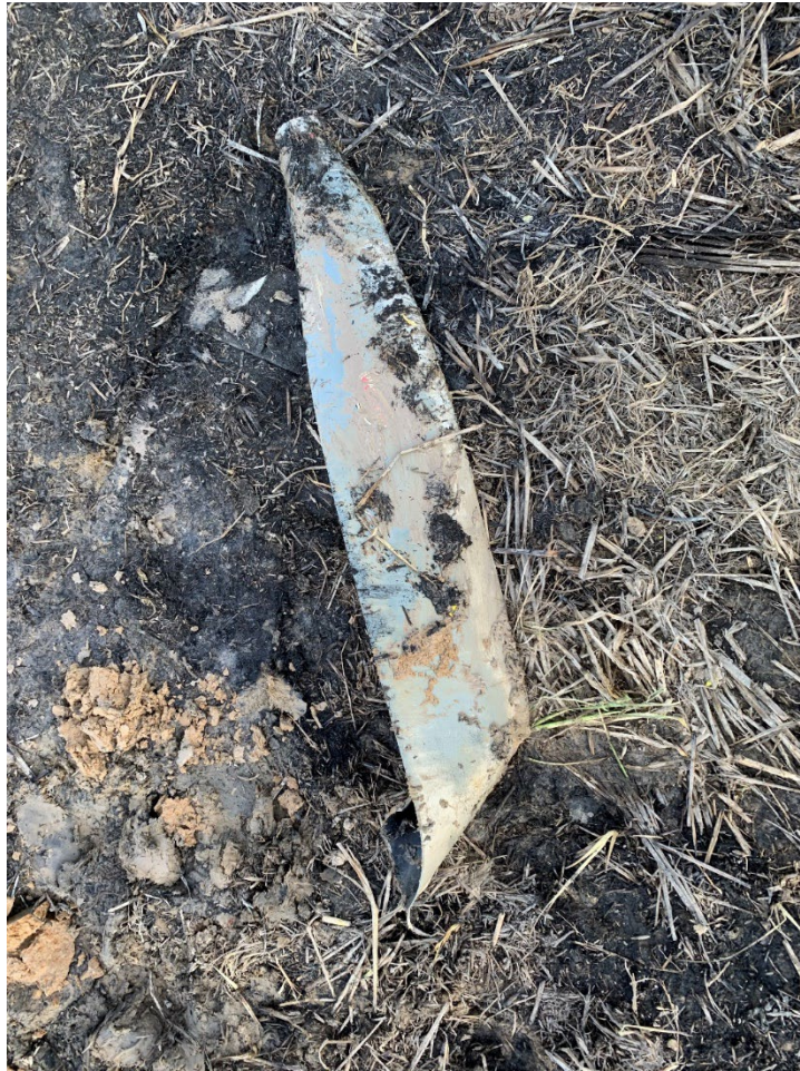
Figure 17: Fractured Propeller Blade
