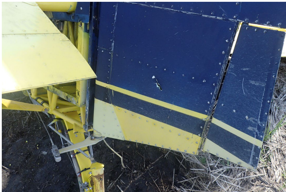
Figure 10: Puncture on Lower Left side of Rudder
