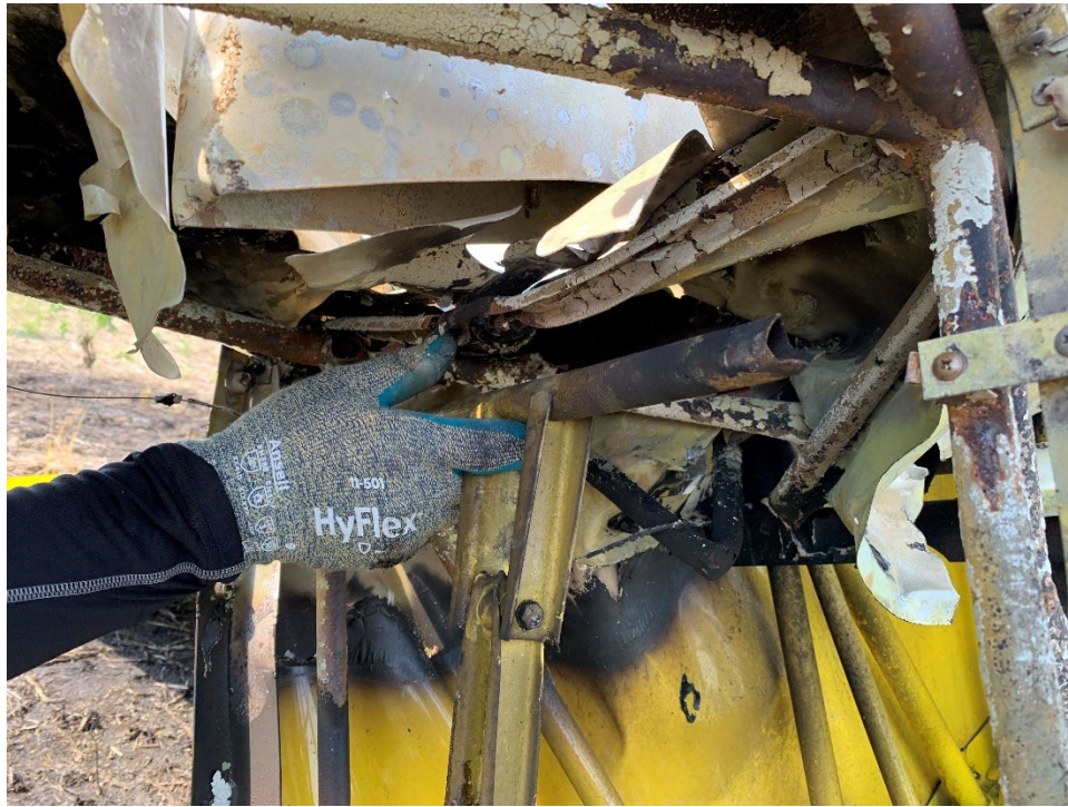
Figure 11: Crossbar for Elevator Control aft Idler.
