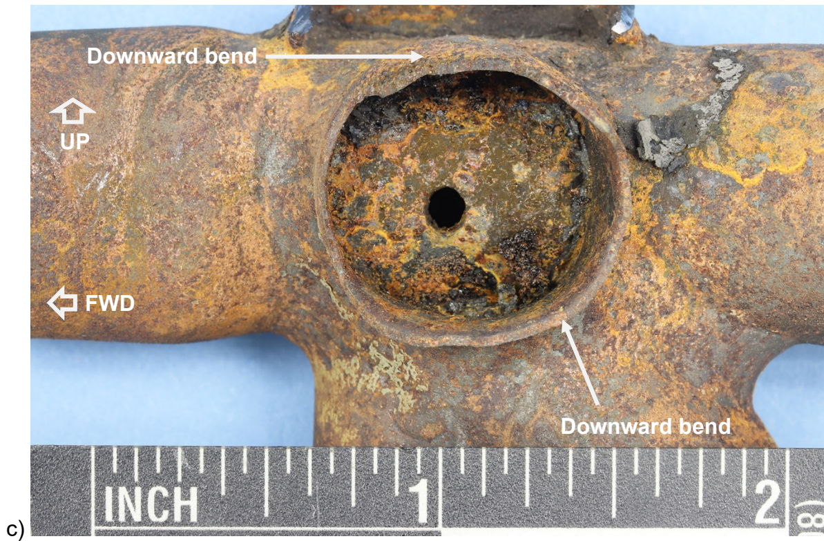
Figure 2 (cont.): and c) image of the mating fracture at the right-side node, showing downward bending of the tube wall along the top and bottom.
