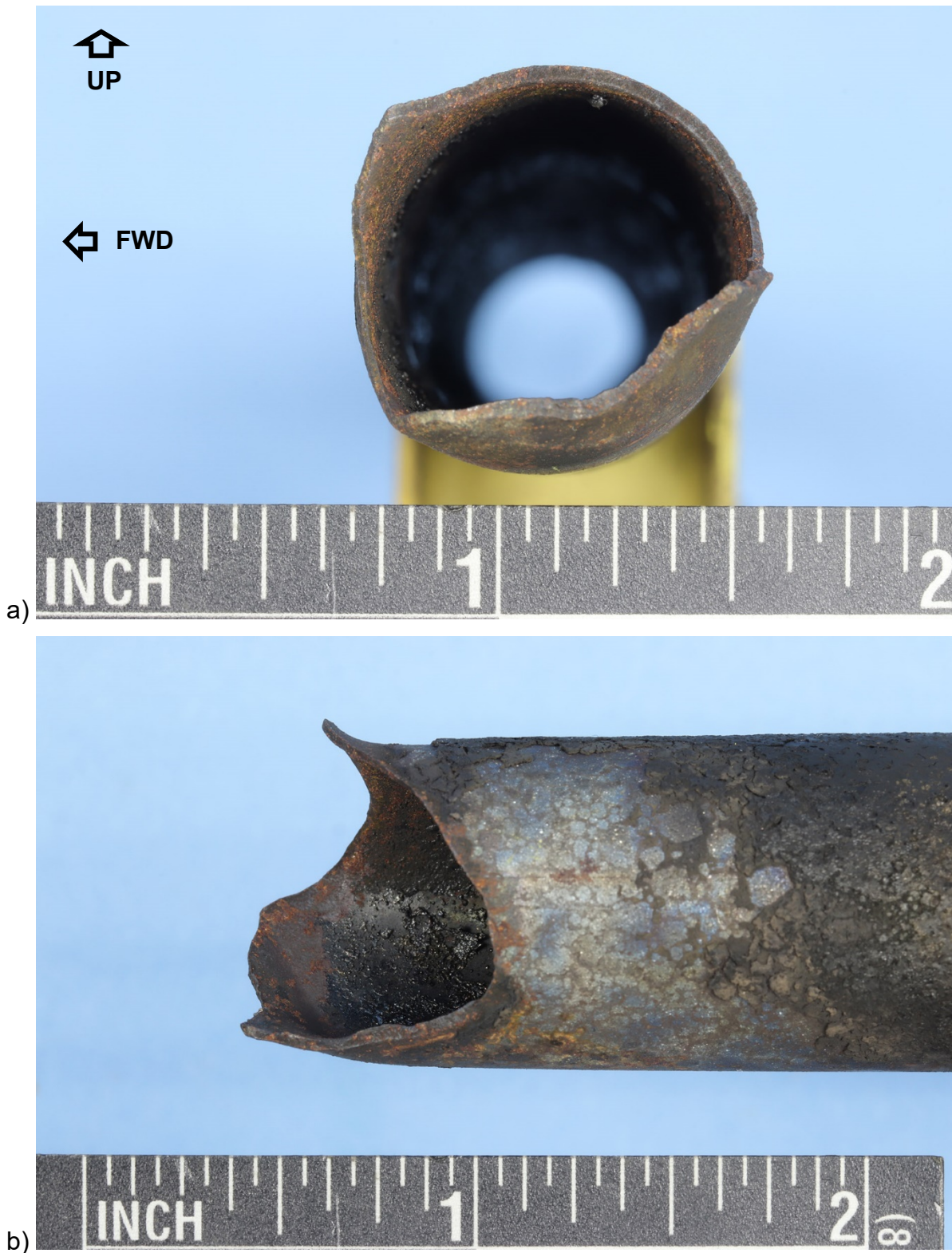
Figure 3: The left-side fracture of the cross-brace tube; a) longitudinal view of the fracture; b) side view showing deformation at the tube end near the fracture. The tube is viewed looking down and forward.
