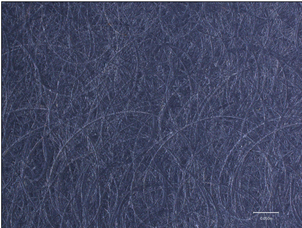
Figure 4. Typical scratch pattern on the bond surface on the exterior of the piece shown in figure 2.
