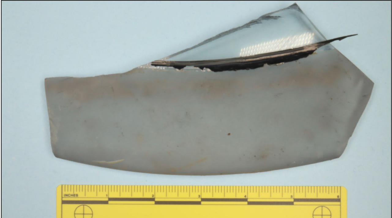
Figure 2. View of a piece from the windshield perimeter after cleaning with a solution of Alconox and water and light brushing.
