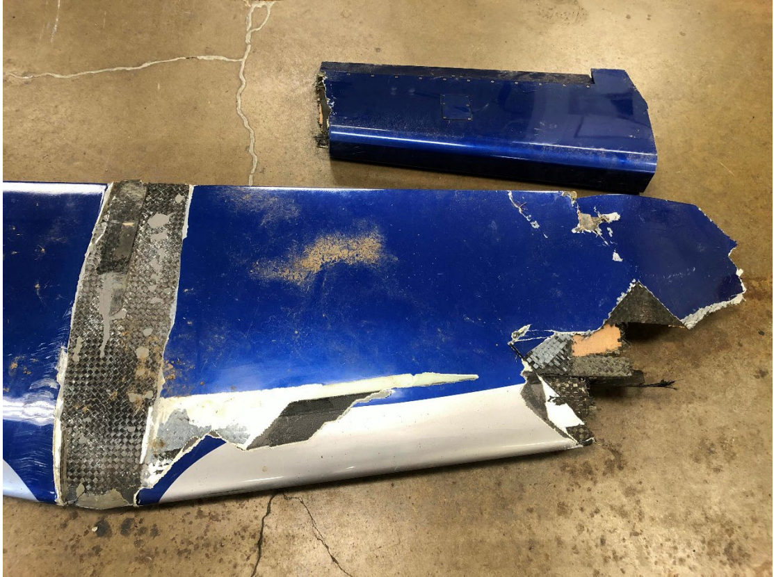
Photo 5 – Horizontal stabilizer and left elevator that separated inflight
