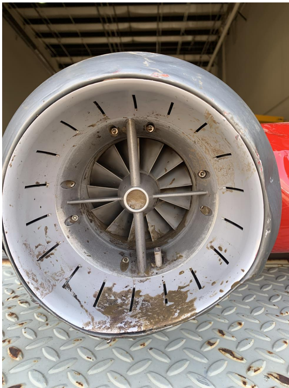
Photo 9 – Engine Inlet and Compressor Disc
