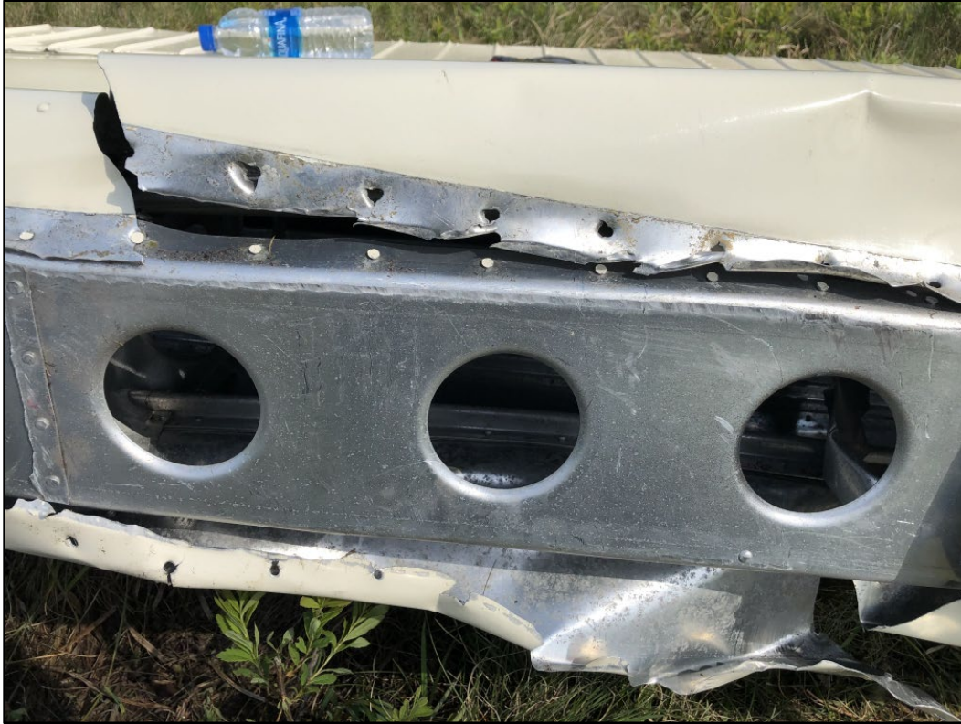
Figure 9 - Left Wing Leading Edge and Forward Spar Damage
