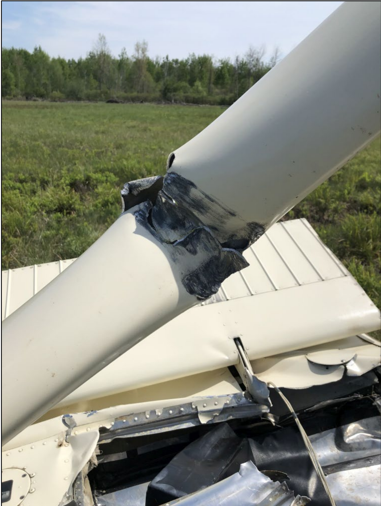
Figure 8 - Left Wing Lift Strut Damage
