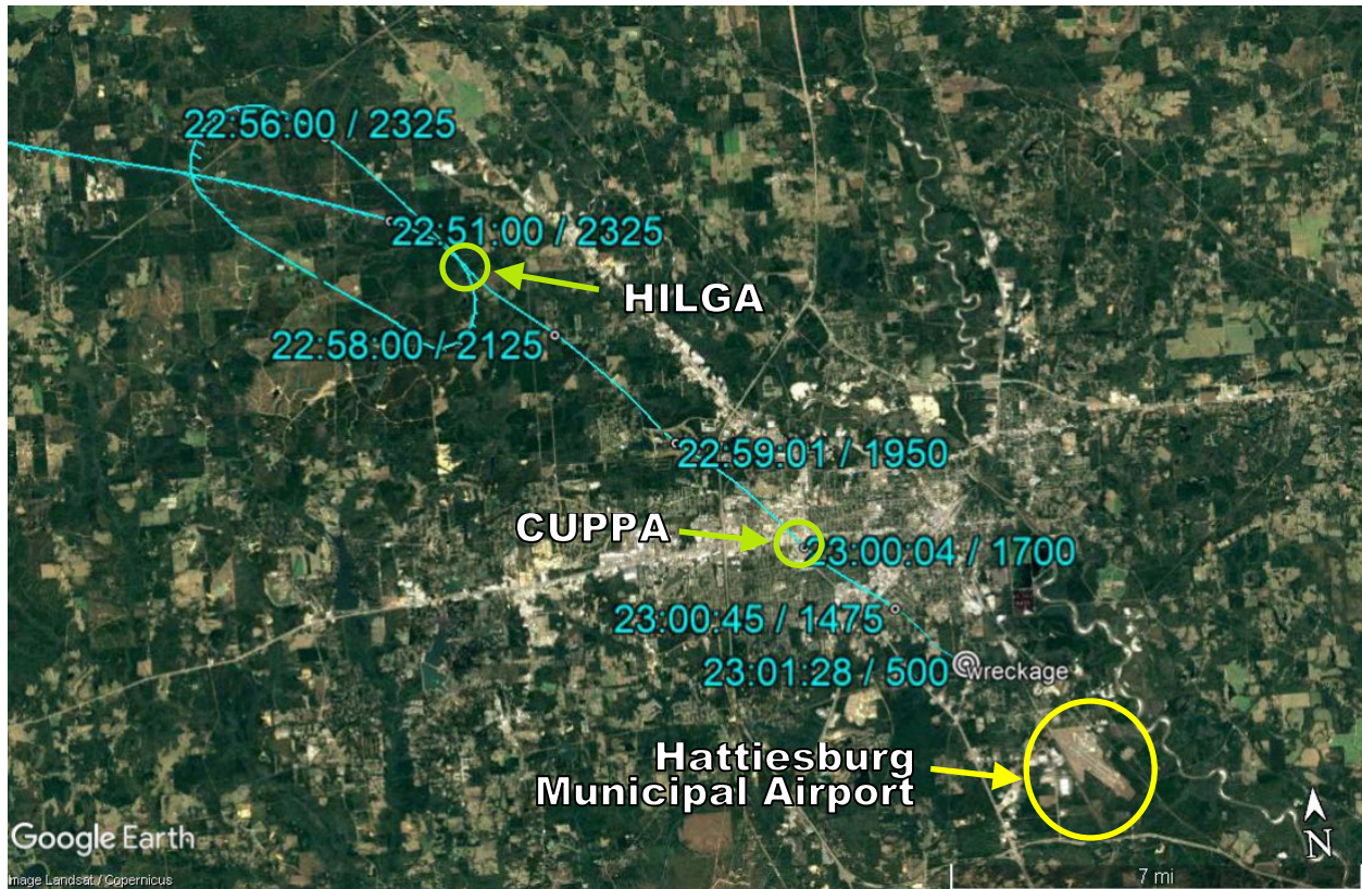
Figure 3. Approach flight path and impact location, selected times and altitudes (msl) annotated in blue. Waypoints HILGA and CUPPA and the airport are also indicated; see the approach chart in the Appendix.
