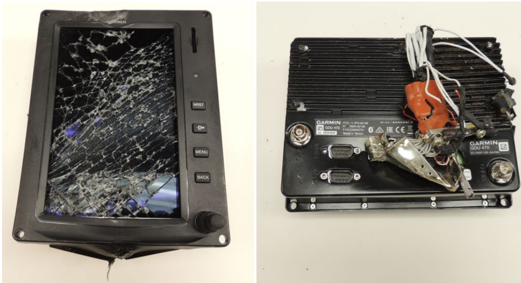
Figure 1: The front and back of the Garmin GDU 470, as received.
