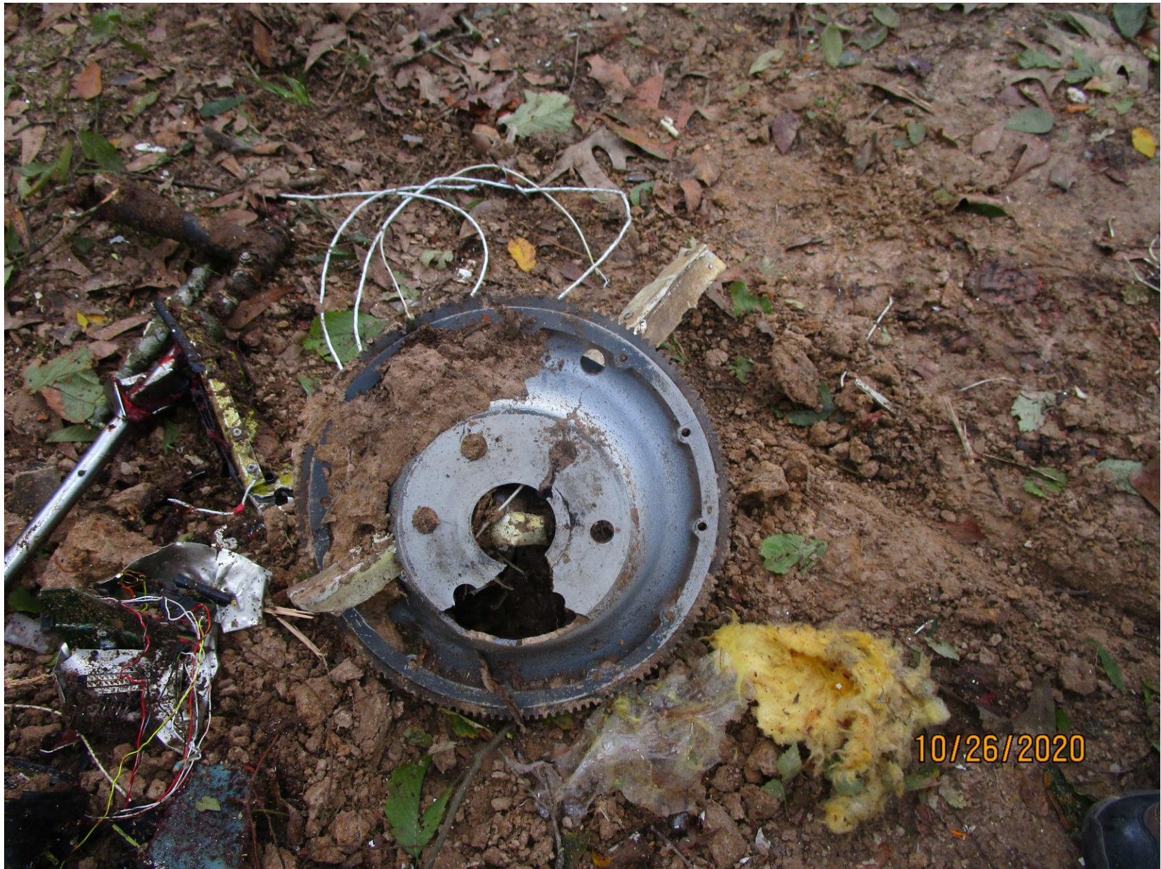
Photo 7 – Engine Starter Ring Gear with Embedded Debris
