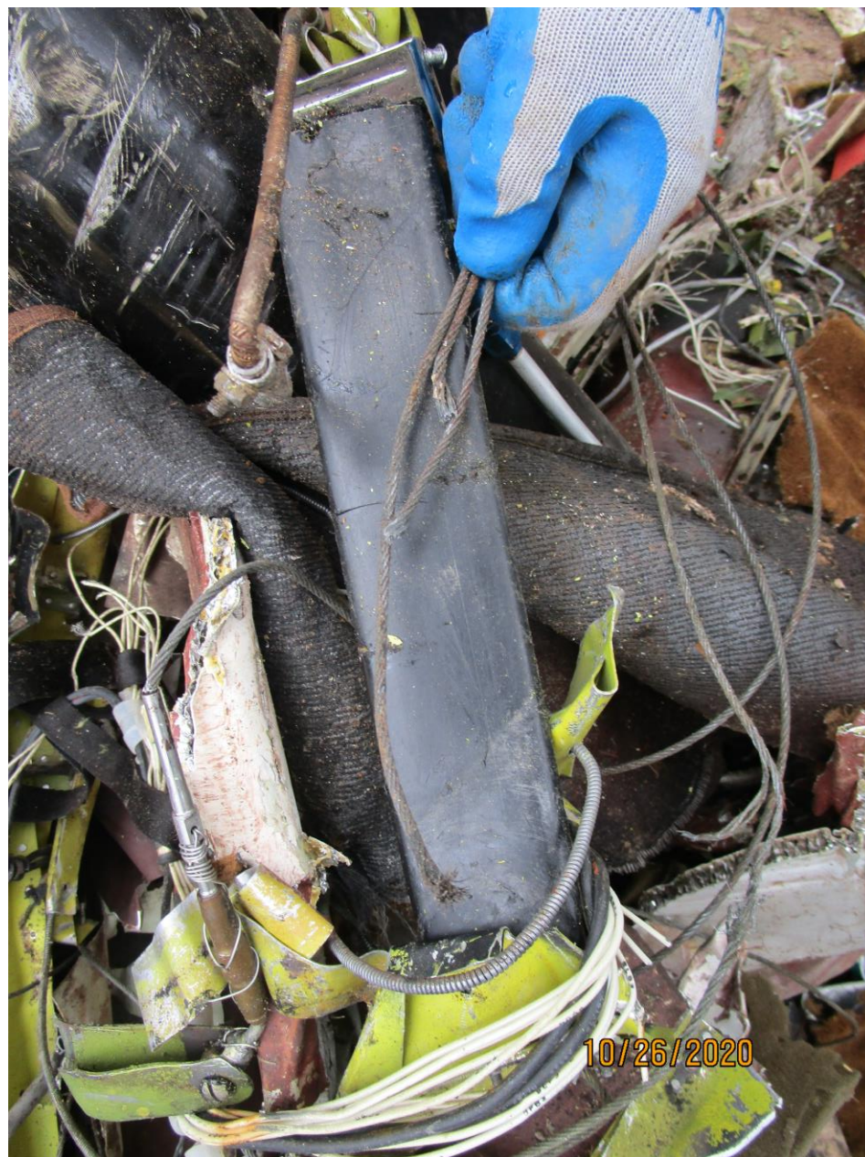
Photo 11 – Flight Controls Cable Separations
