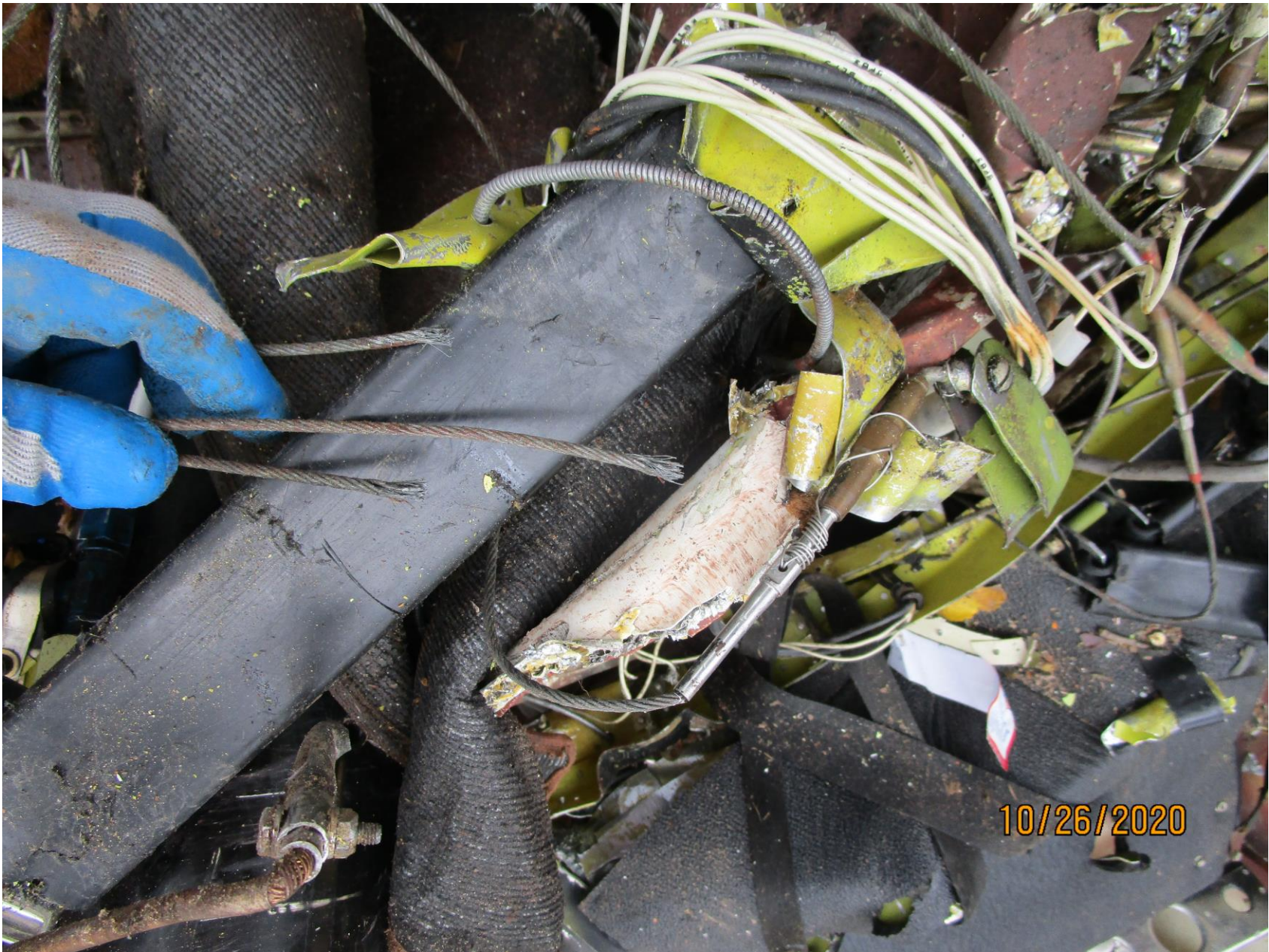
Photo 12 – Detail View of Broken Flight Control Cables
