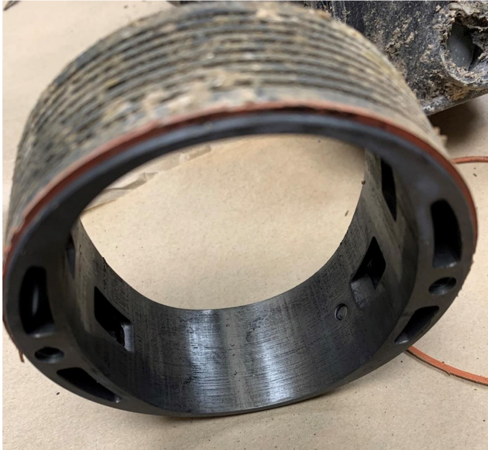
Figure 8. Pump Stator Housing, Inside View
