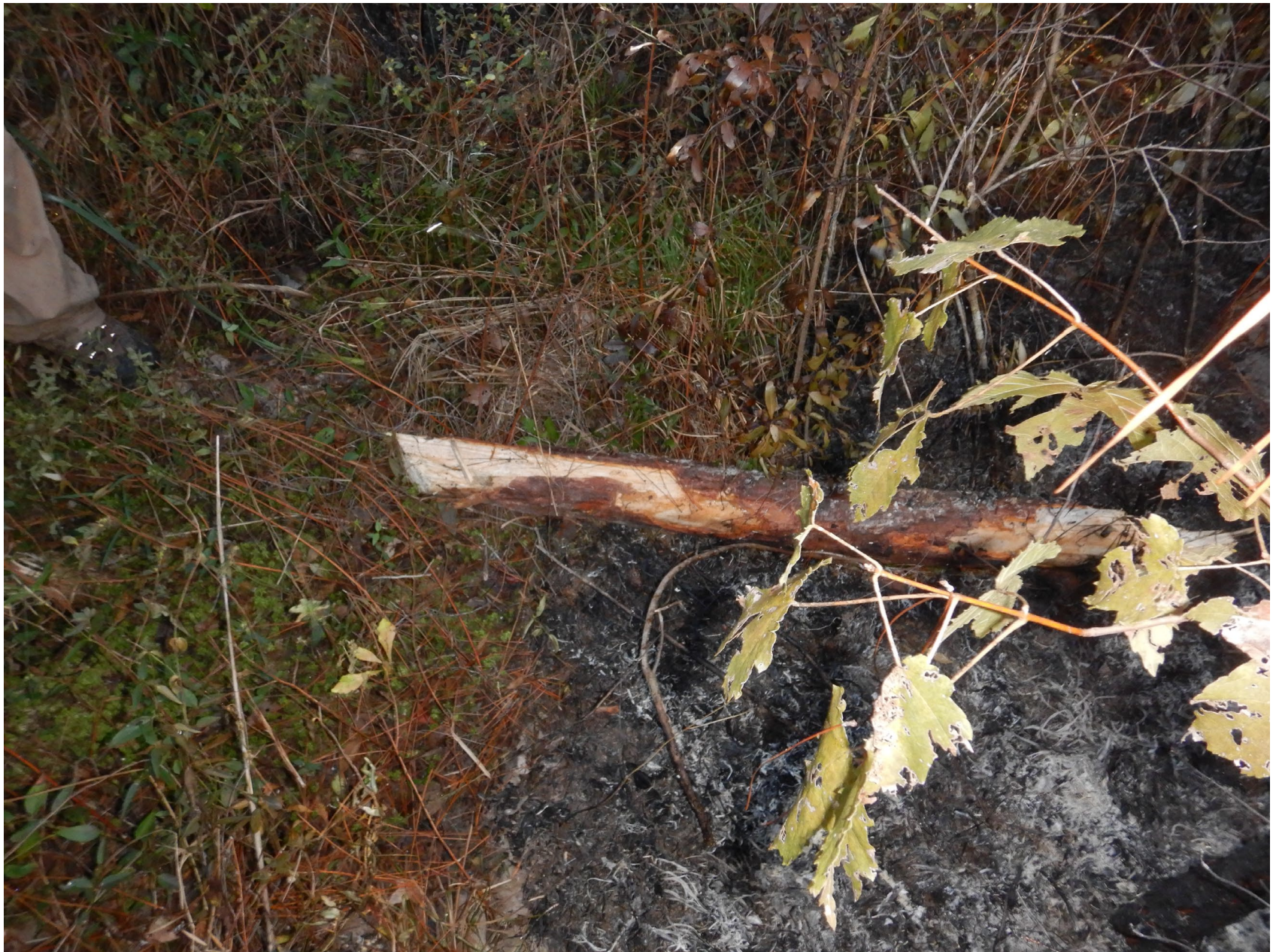
Photo 11 – Tree with propeller cut
