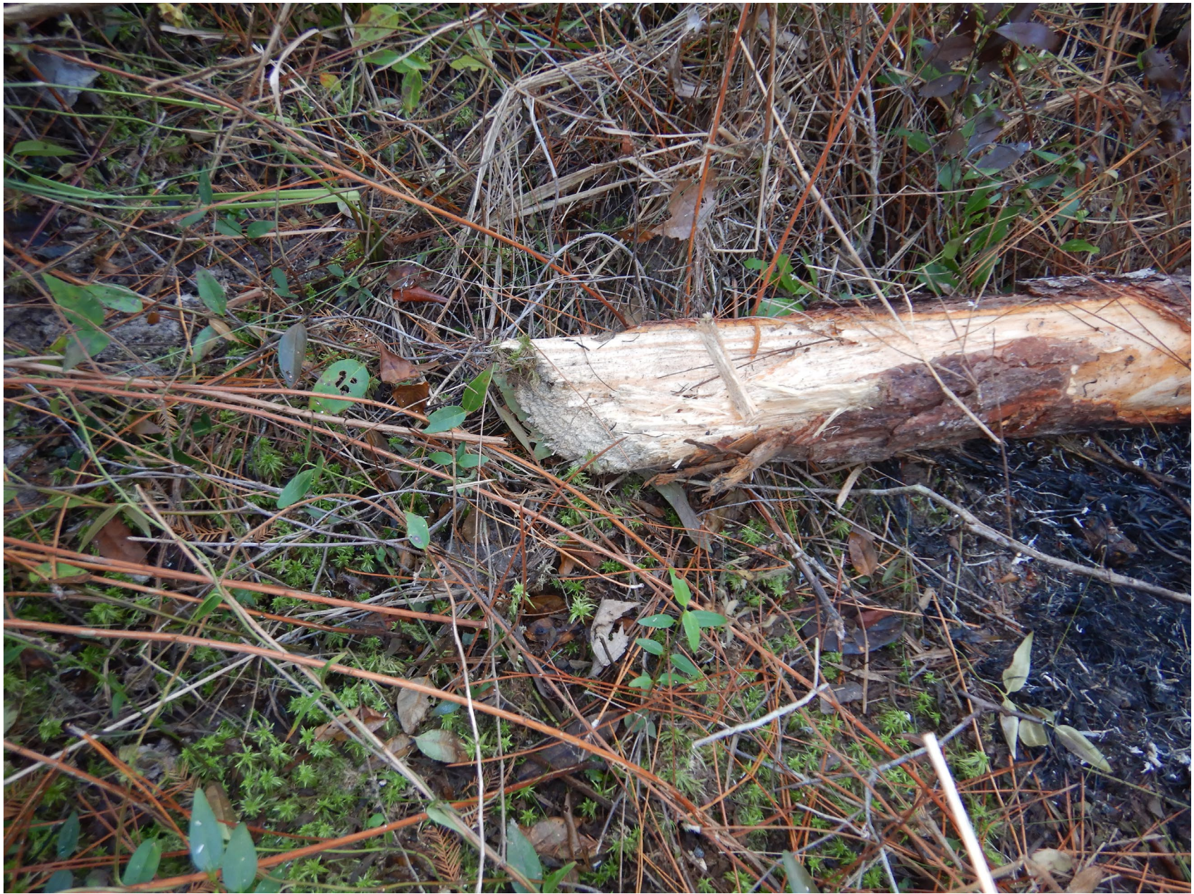
Photo 12 - Tree with propeller cut
