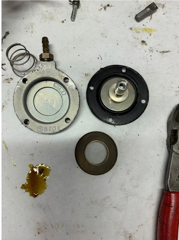
Figure 18. Disassembled Fuel Distribution Manifold
