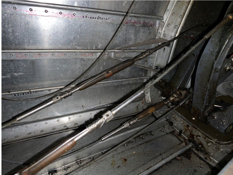
Figure 6. Control Cables to the Elevator and Rudders
