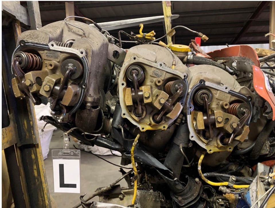
Figure 14. Engine, Left Side, Valves, Springs, and Rockers
