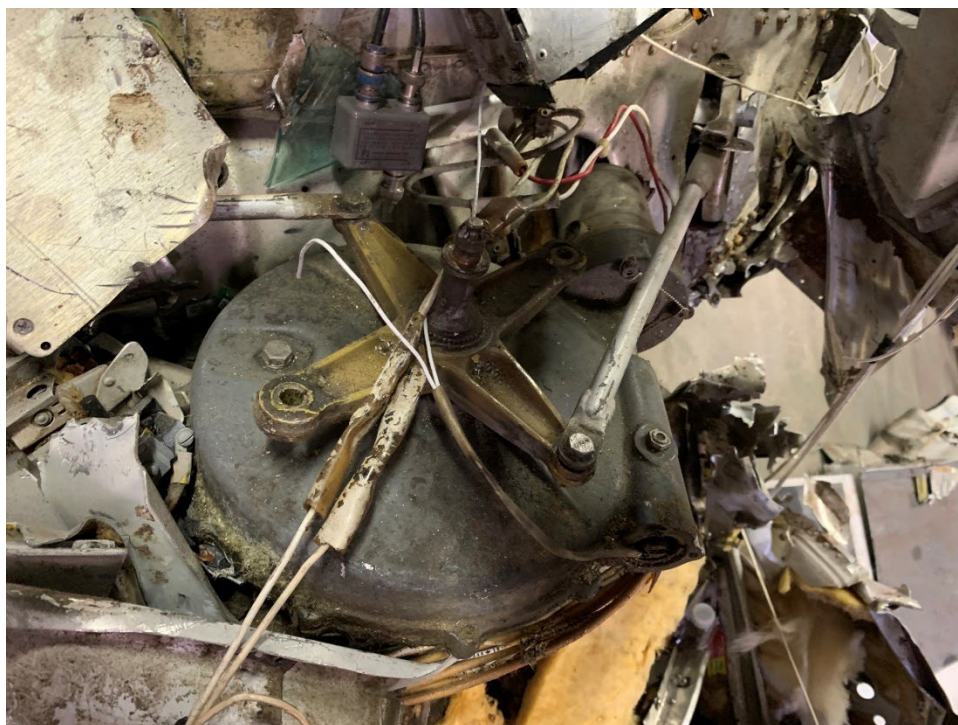
Figure 5. Landing Gear Gearbox
