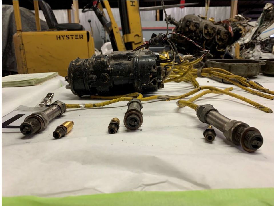
Figure 17. Right Magneto, Top Spark Plugs & Fuel Injectors, Cylinders 1, 3 & 5 (Left to Right)
