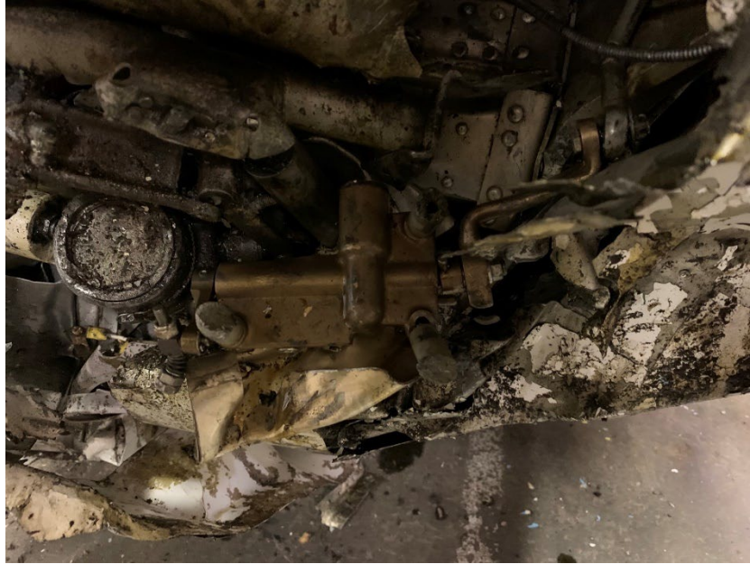
Figure 19. Throttle Body Housing
