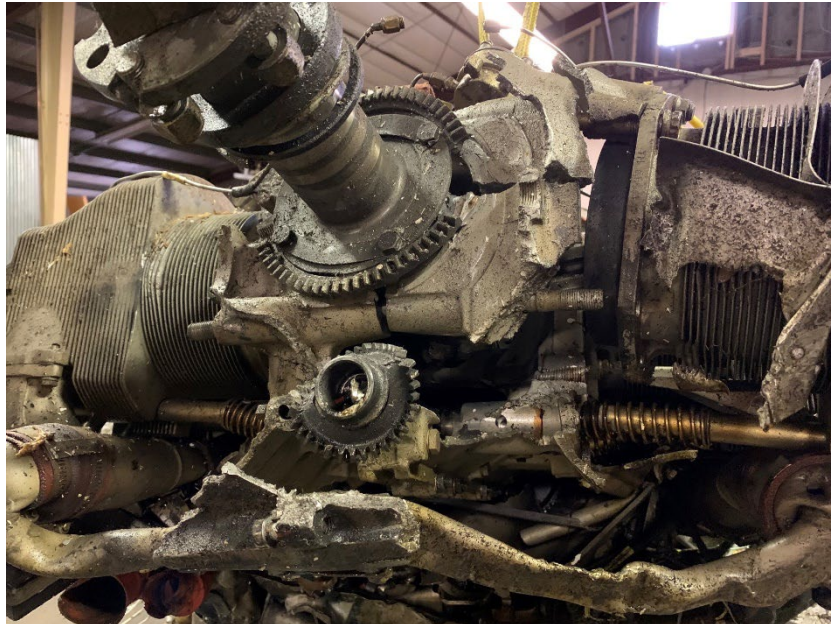
Figure 12. Engine, Front Side, Crankshaft, Camshaft, Number 5 and 6 Cylinders
