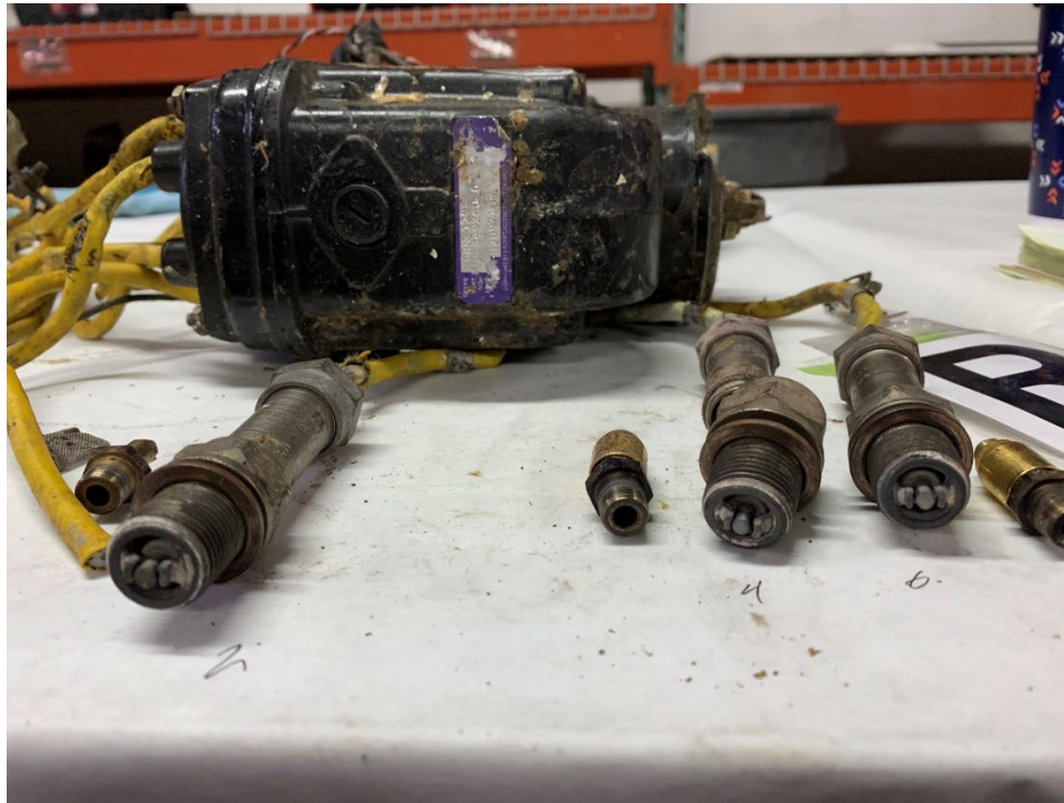
Figure 16. Left Magneto, Top Spark Plugs & Fuel Injectors, Cylinders 1, 3 & 5 (Left to Right)
