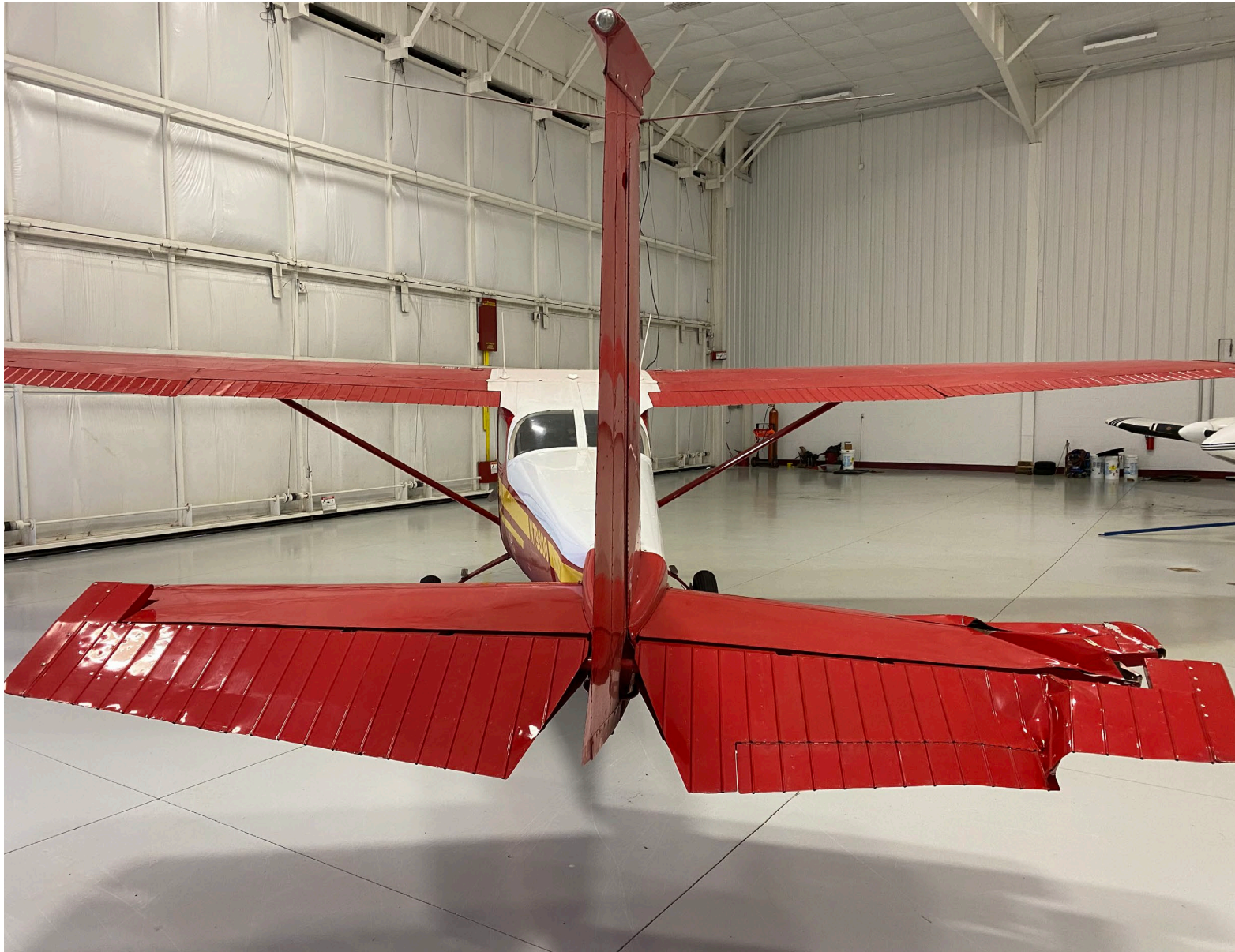
Photo 1 – Damage to Right Horizontal Stabilizer
