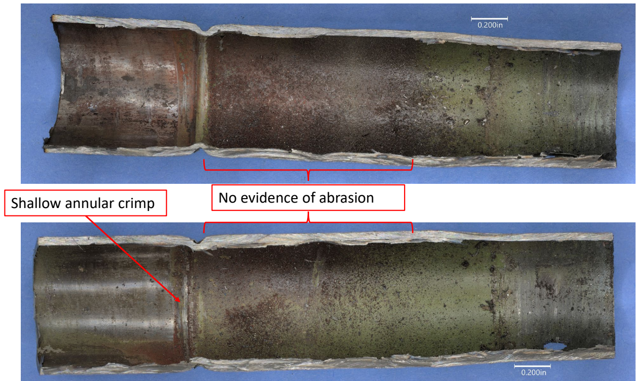
Figure 7: Inner surface of the left-hand steering tube around the annular crimp.
