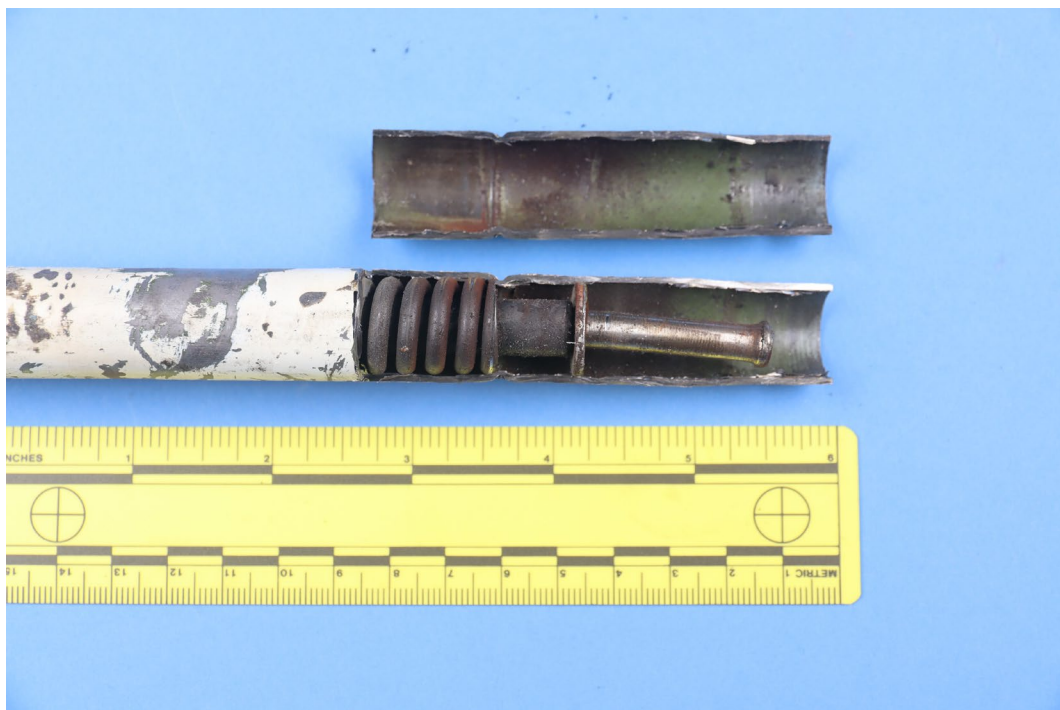
Figure 6: Left-hand steering tube sectioned around the annular crimp.
