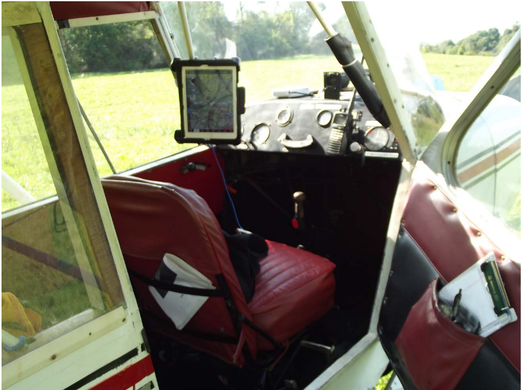
Photo 7 – The cockpit of N81624. Notice hand-held communications radio and moving map display
