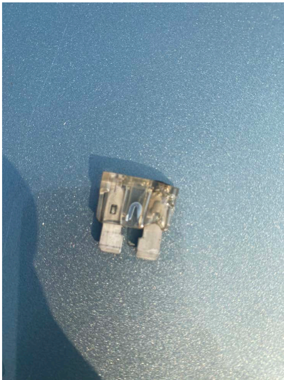
Photo 3 – Failed Fuse (photo provided by Viking Aircraft Engines)
