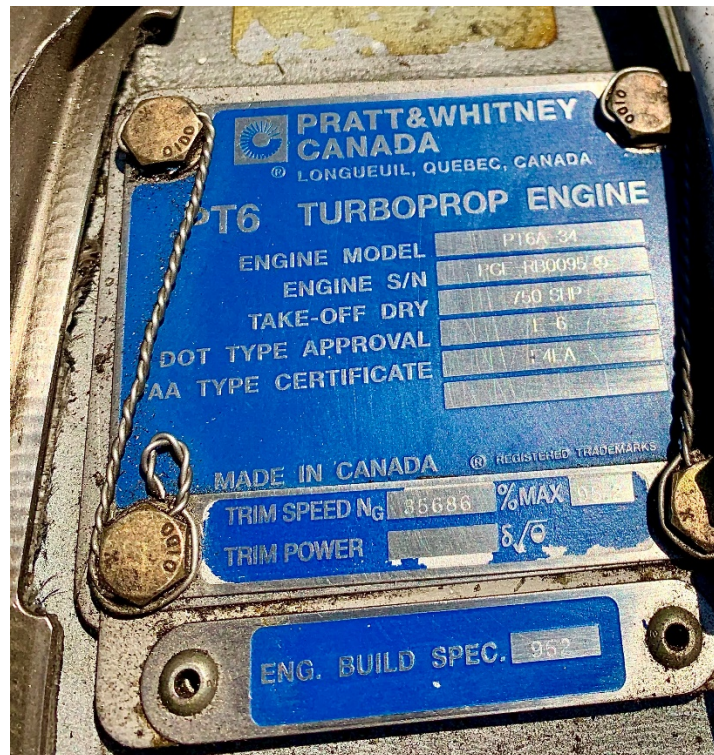
Photo 4- Engine Data Plate
