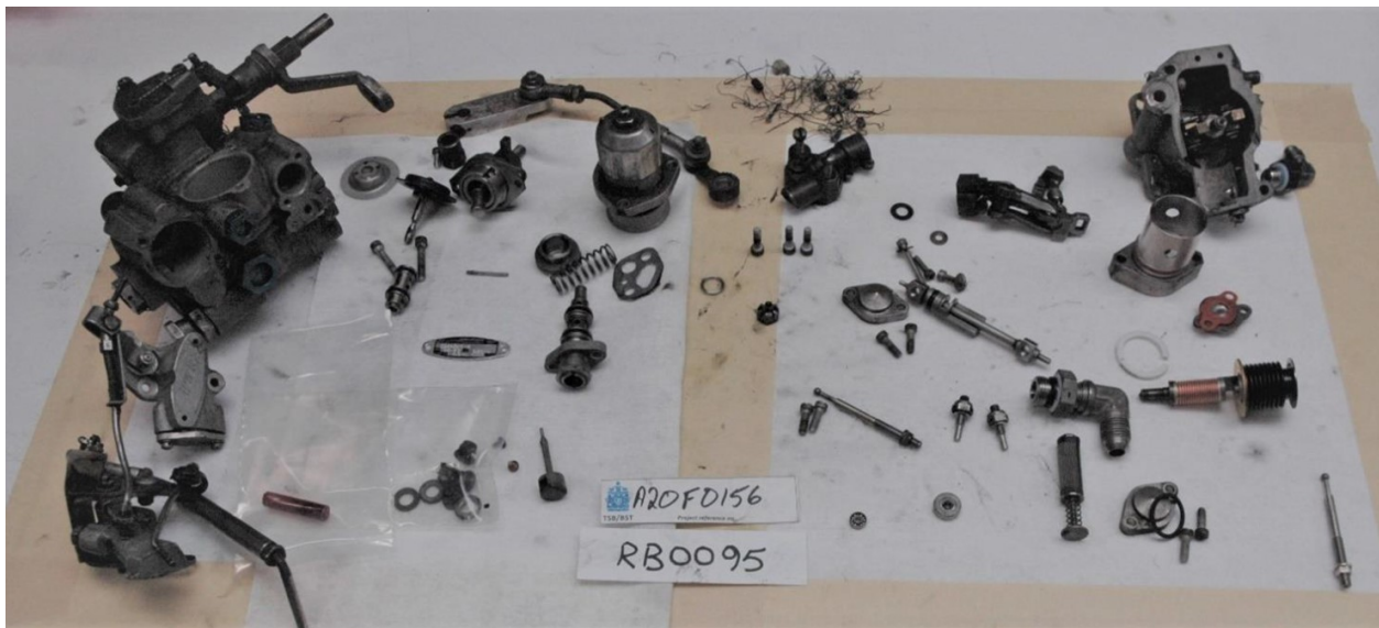
Photo 20- Fuel Control Unit Disassembled (Photo Courtesy of PWC)
