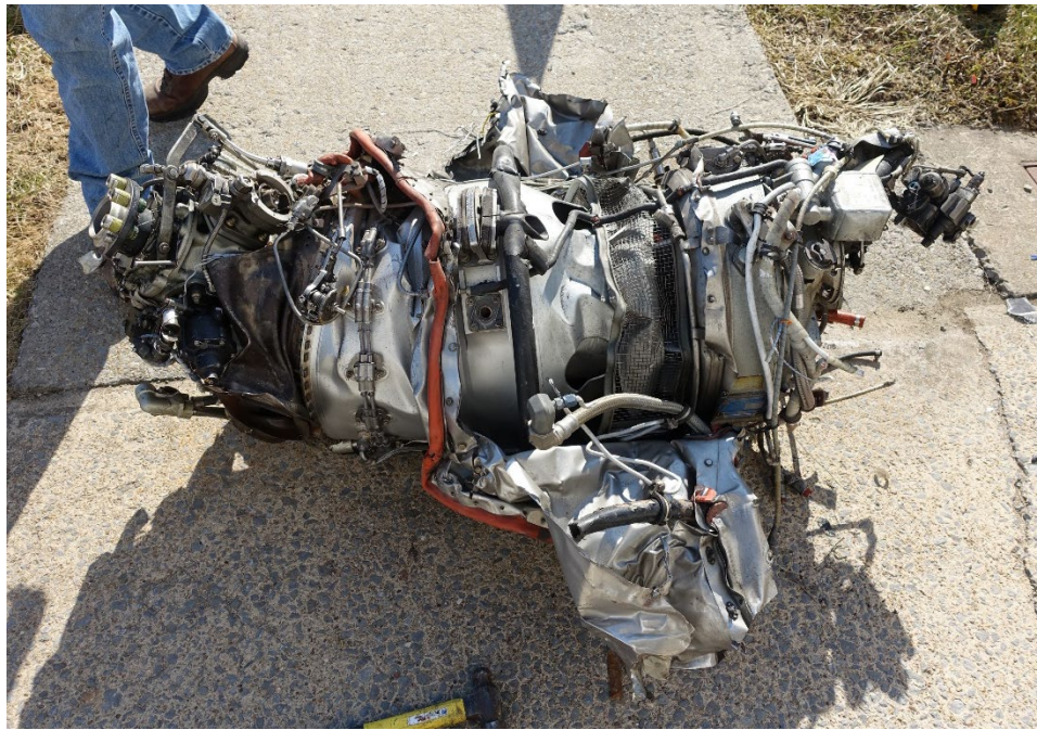
Photo 5- Left Side of the Engine After Airframe Parts Removal
