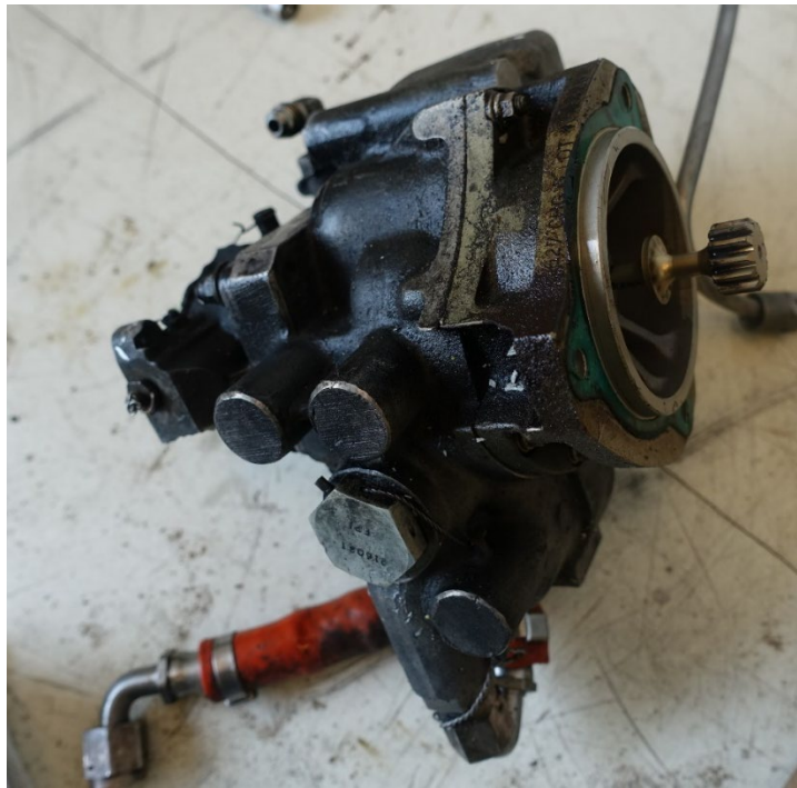
Photo 18- Fuel Pump Spline
