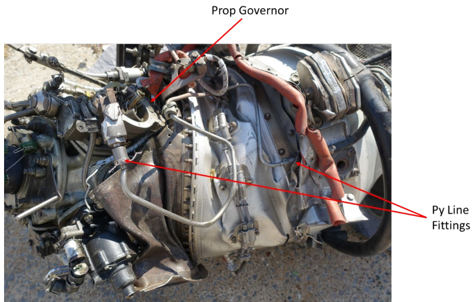
Photo 6- Turboprop Governor and Py Line Fittings
