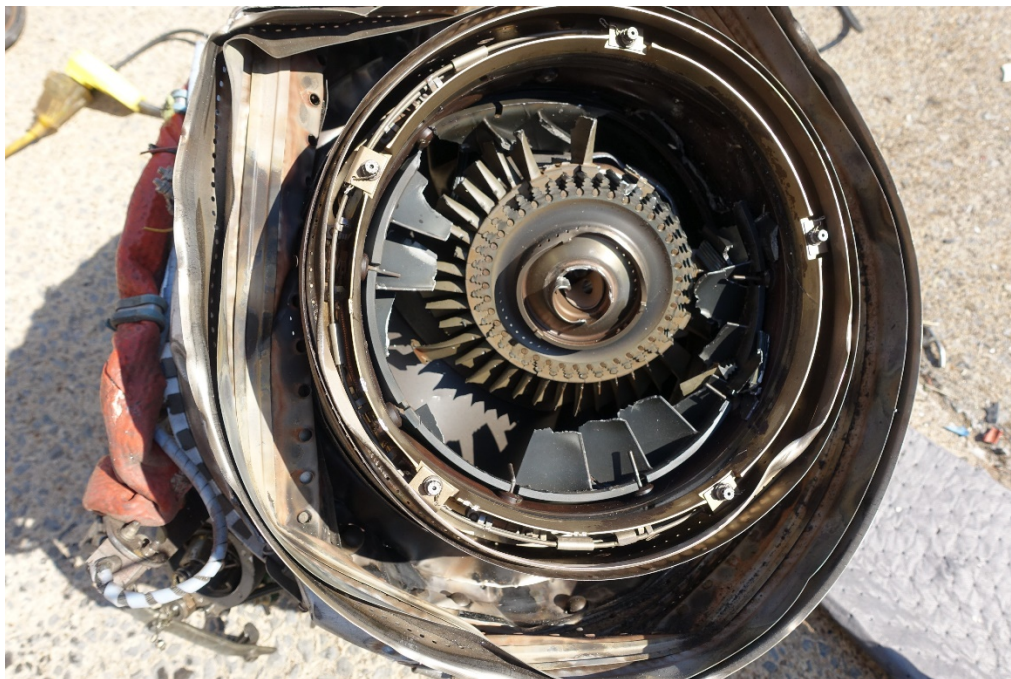
Photo 9- Power Turbine Rotor and Nozzle Impact Damage
