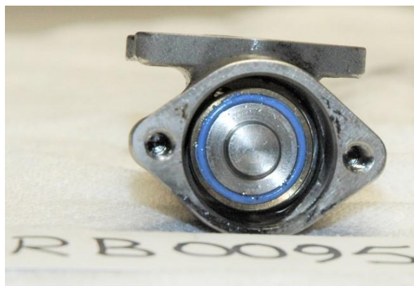
Figure 12 FDV primary valve in the housing
