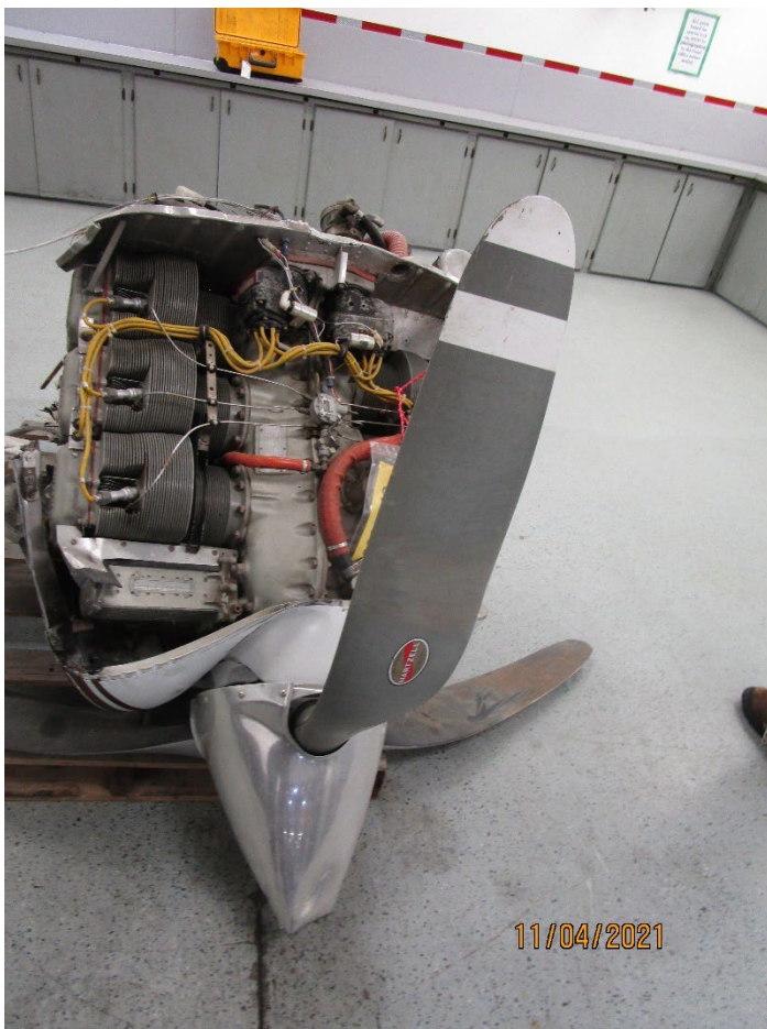
Engine, separated from fuselage and ready for examination
