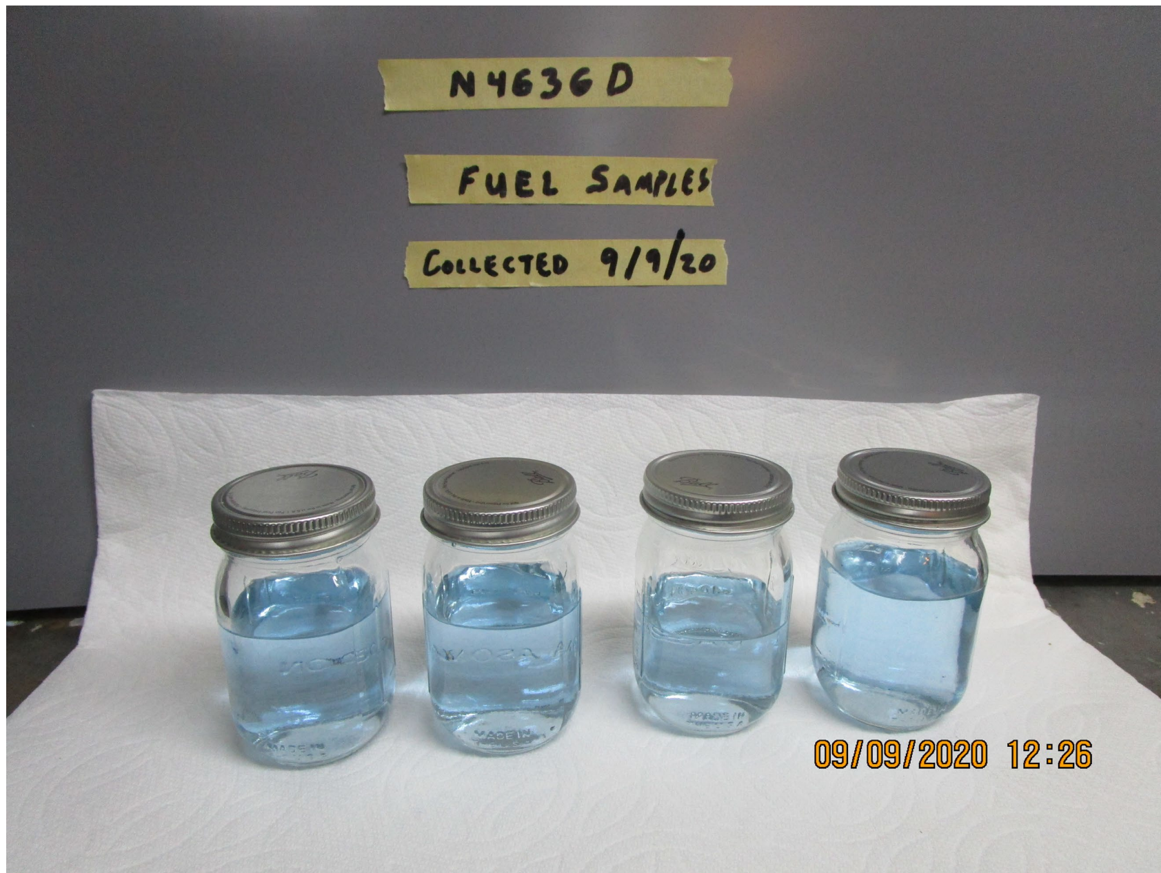
Photo 3 – Fuel Samples taken from each tank 2 days after the accident (Photo courtesy of FAA)
