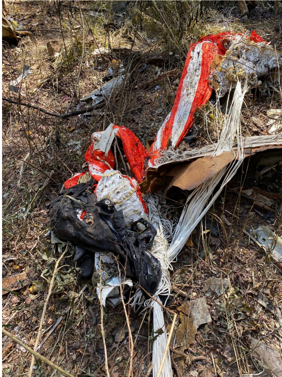
Photo 7 - Supplied view of the CAPS parachute in the debris field.
