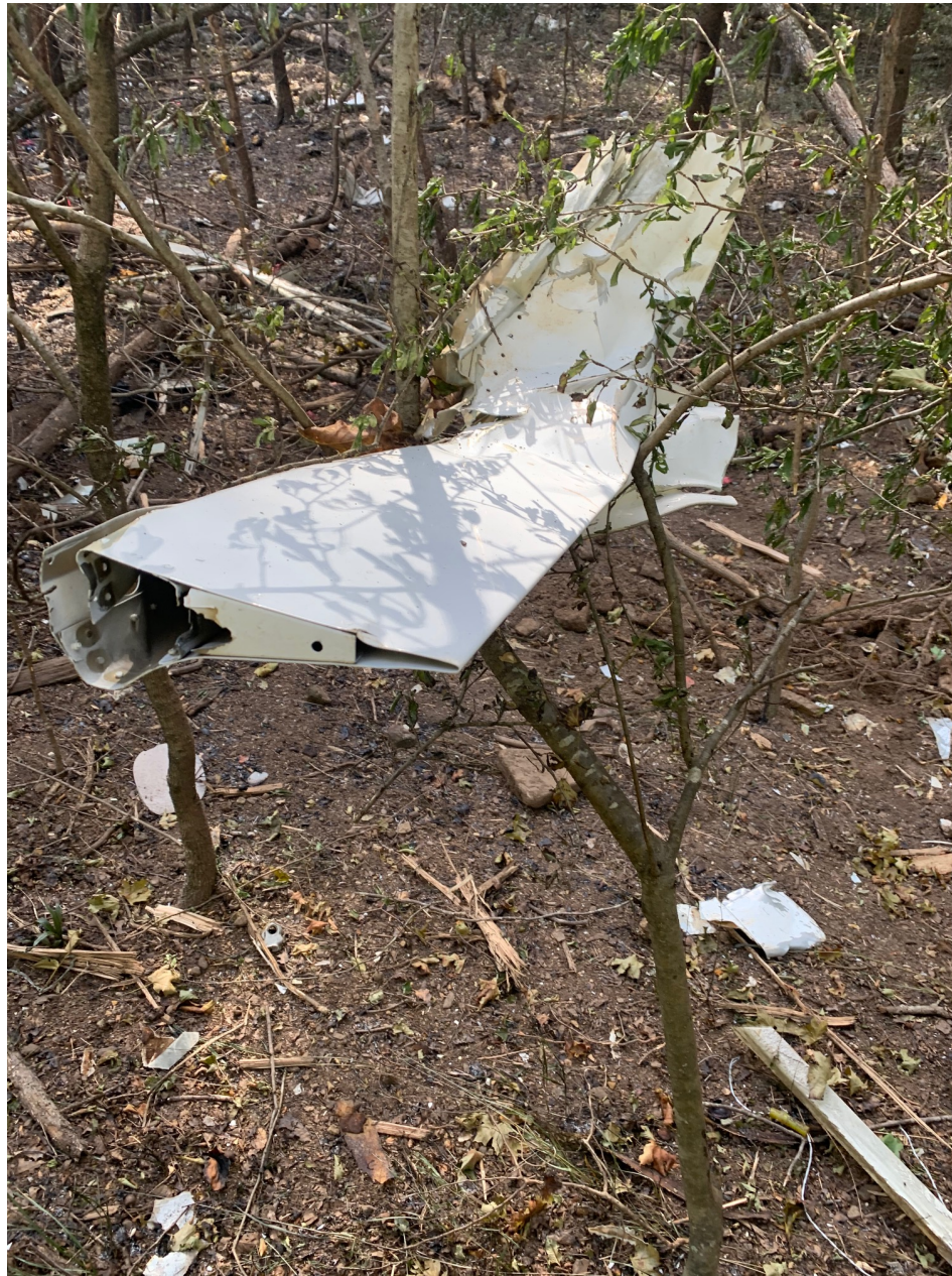
Photo 3 - Supplied view of a separated control surface in the debris path.
