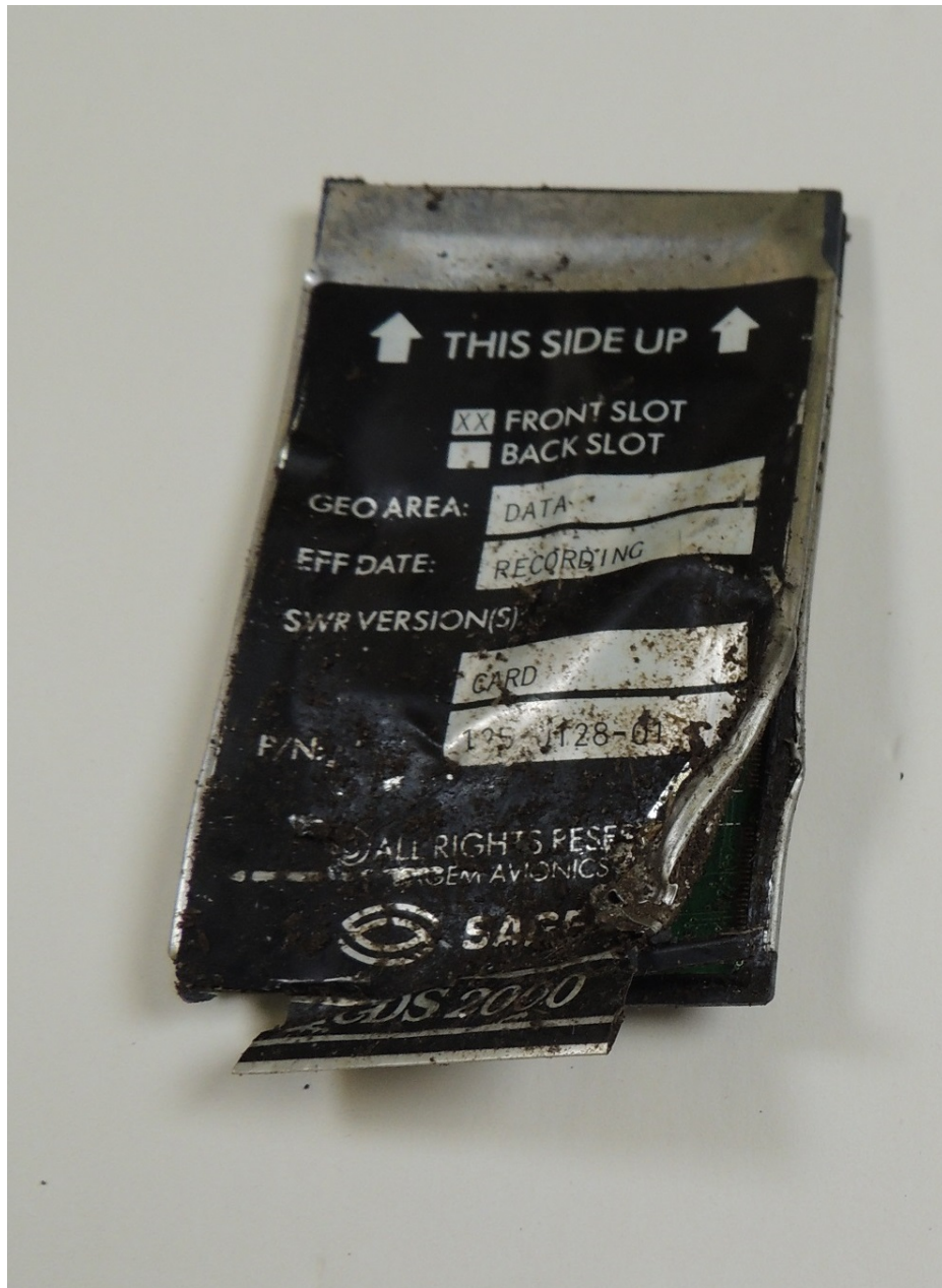
Photo 1 – The CF card arrived exhibiting signs of impact damage.
