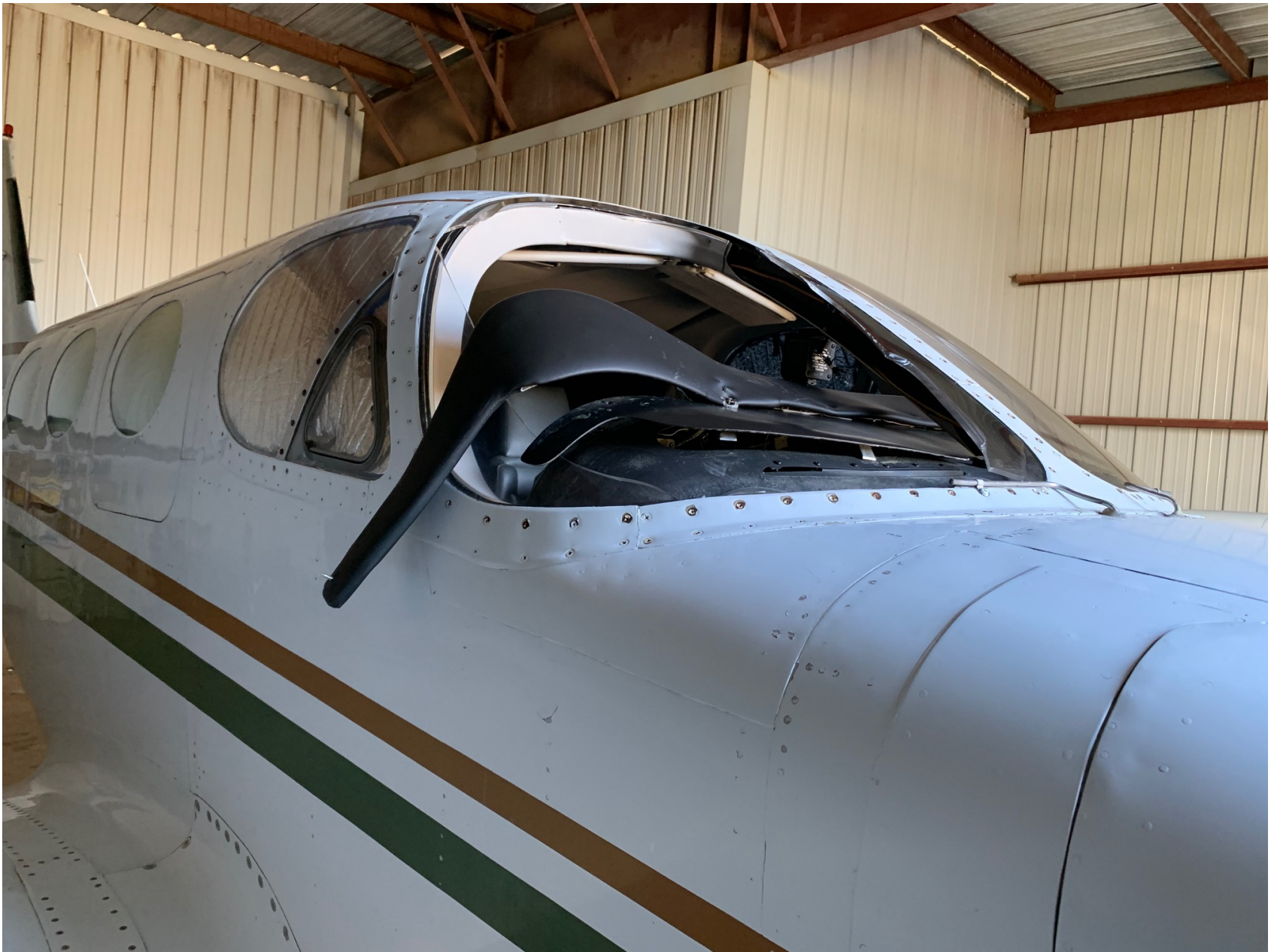
Photo 1 – Damaged Windshield (Pilot Photo)
