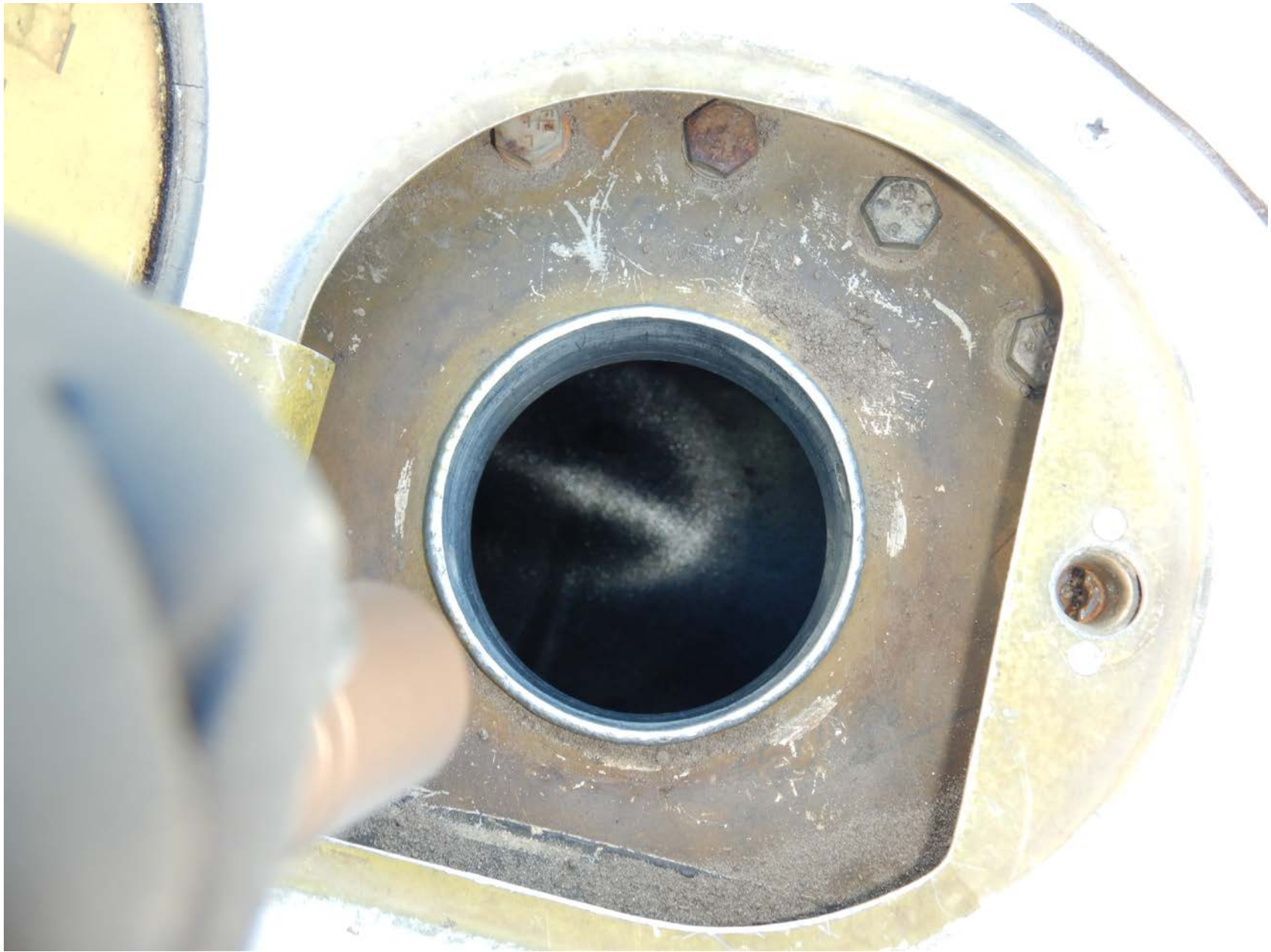
Photo 4 - Inside the left fuel tank. Note the left fuel tank bladder was breached. During recovery of the aircraft, fuel was seen streaming from the left wing root, and there was a fuel blight underneath the left wing
