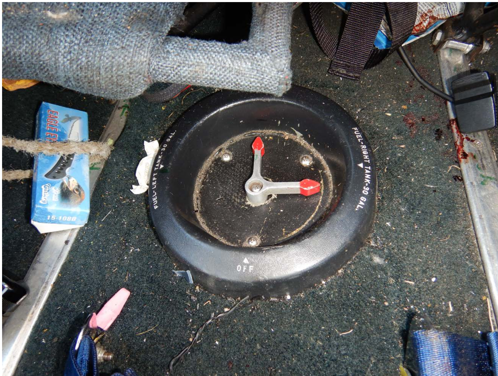
Photo 6 - The fuel selector, positioned on the right fuel tank. During removal of the fuel selector for testing, fuel came from the left fuel line but not the right fuel line
