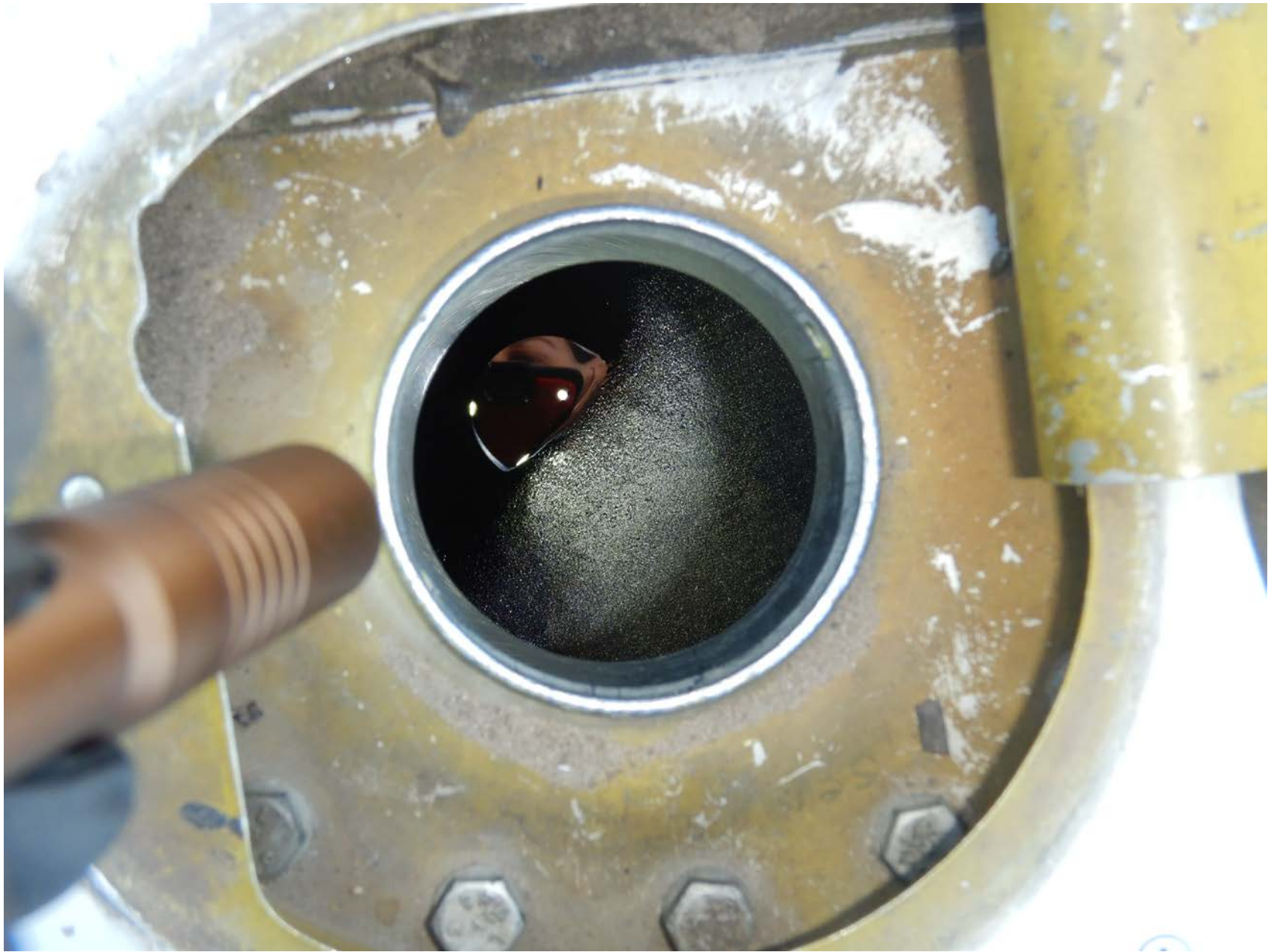
Photo 5 - Inside the right fuel tank. Fuel tank bladder was not breached but contained no fuel
