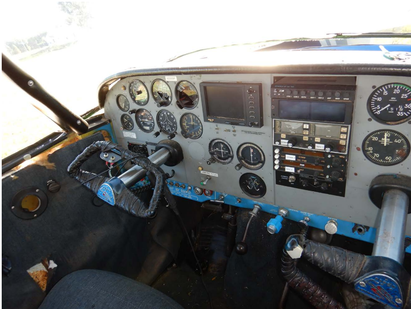
Photo 7 - The instrument panel. Note propeller control is full forward, the throttle is aft and bent down, the carburetor heat is closed, the primer is in and locked, and the mixture control is broken off
