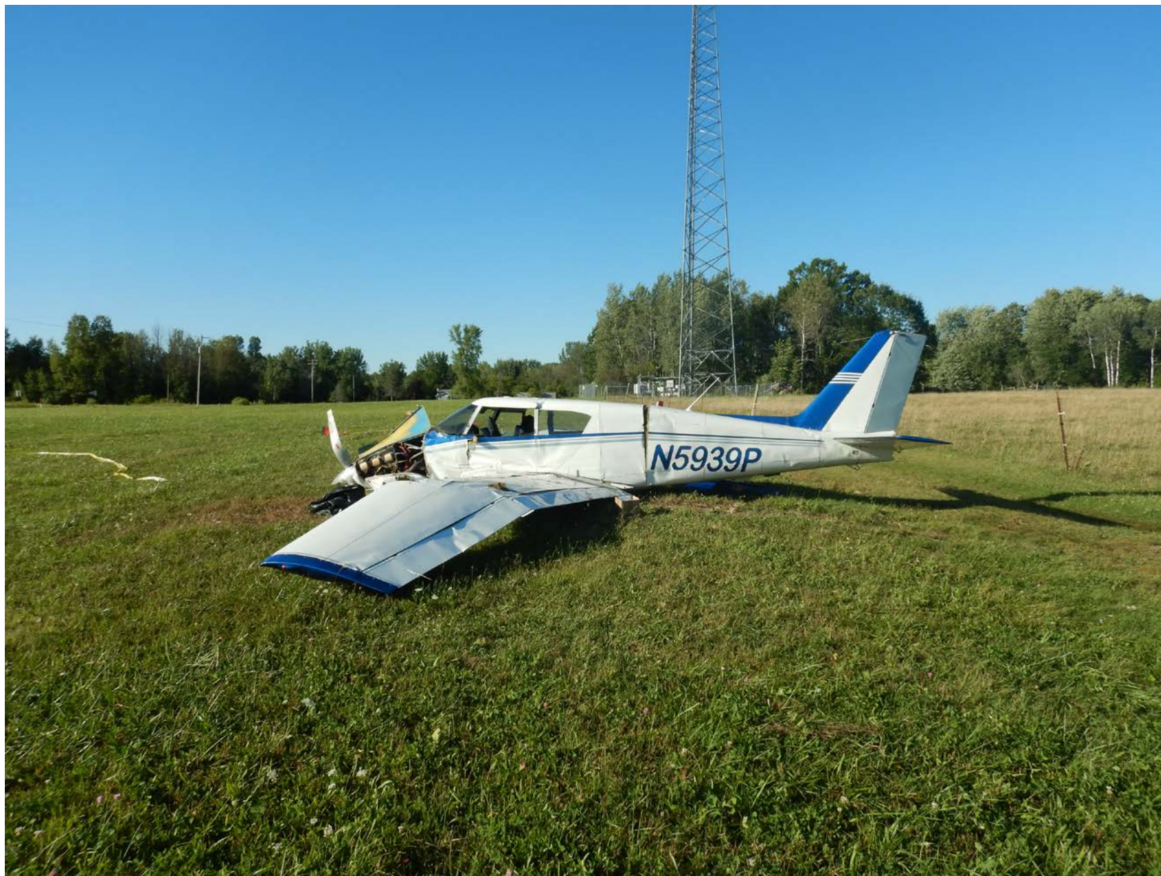
Photo 3 - Left side of airplane with circumferential break in the fuselage and buckled left wing
