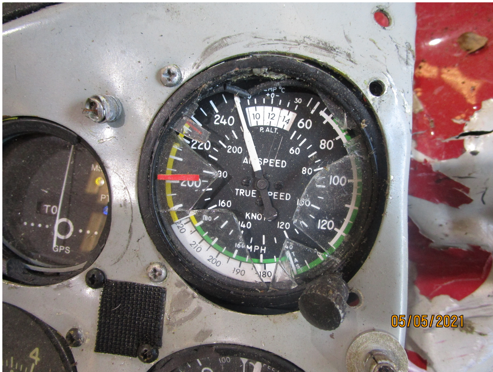
Photo 16 – Image of the damaged airspeed indicator, showing a needle slap marking (courtesy of the National Transportation Safety Board).
