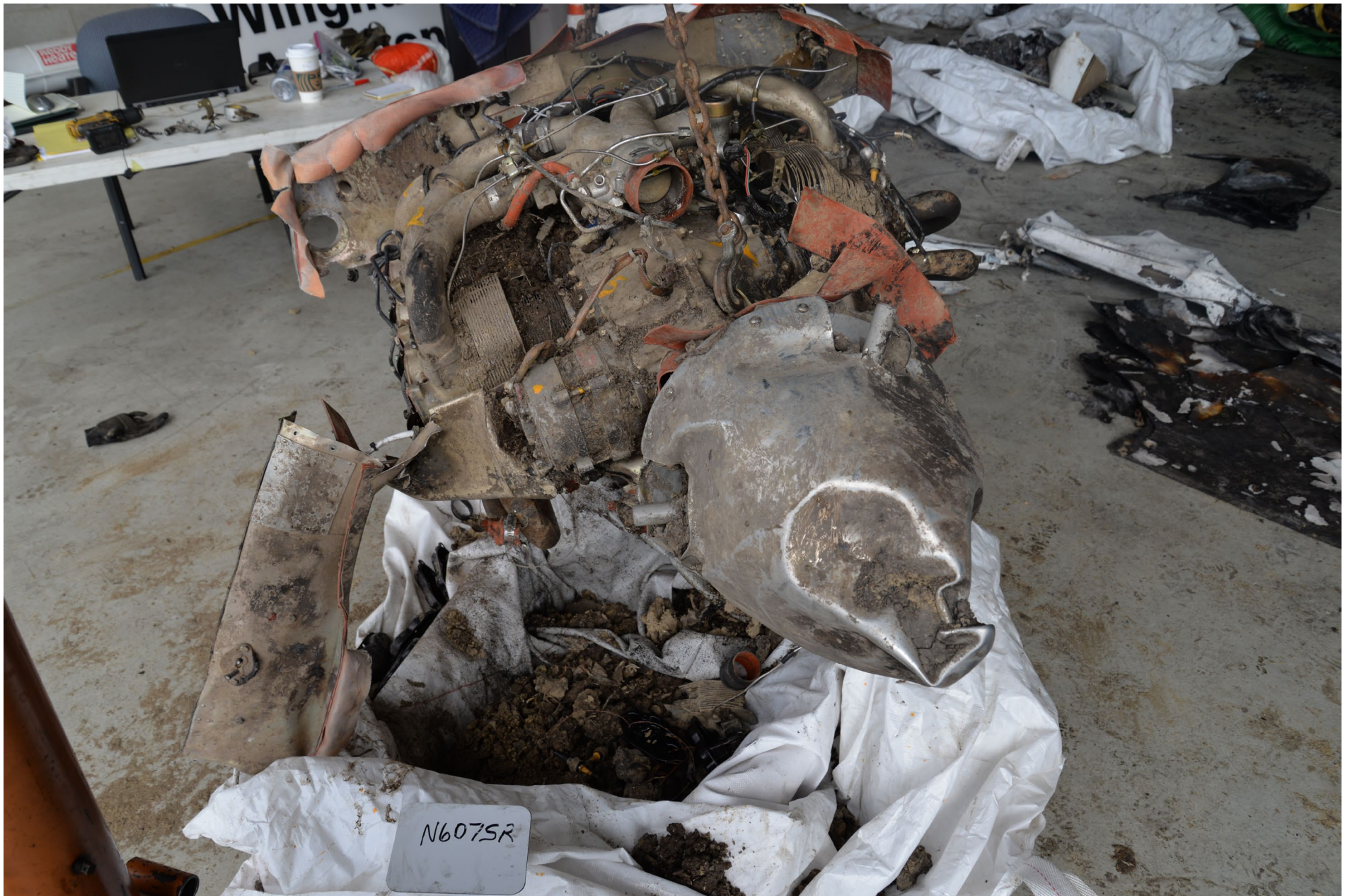
Photo 6 – Engine and Propeller Assembly (photograph provided by Cirrus Aircraft)
