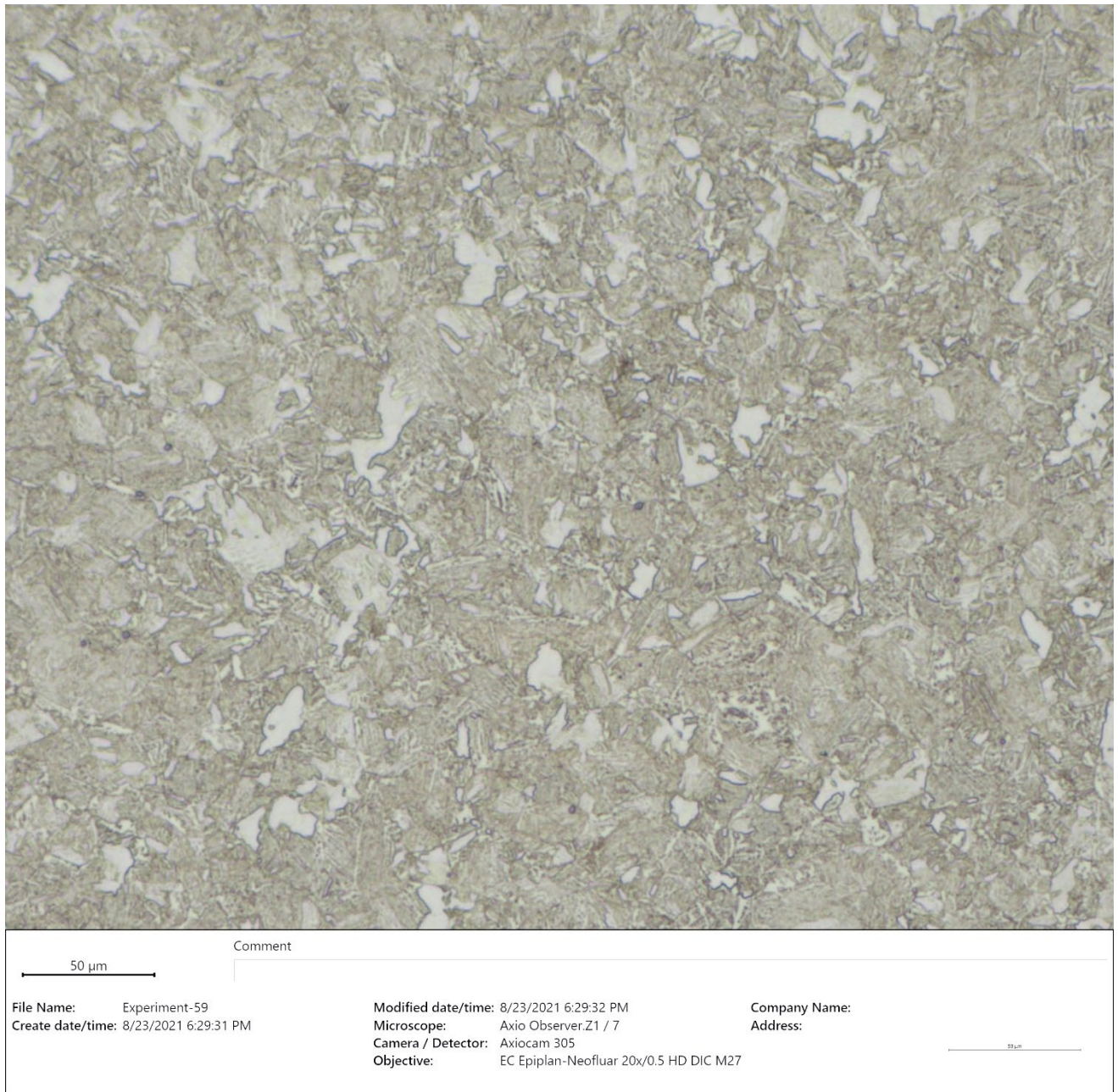
Figure 19 – BF optical micrograph of a typical area of the rod microstructure adjacent to the surface (~500X, etched 2% nital).
