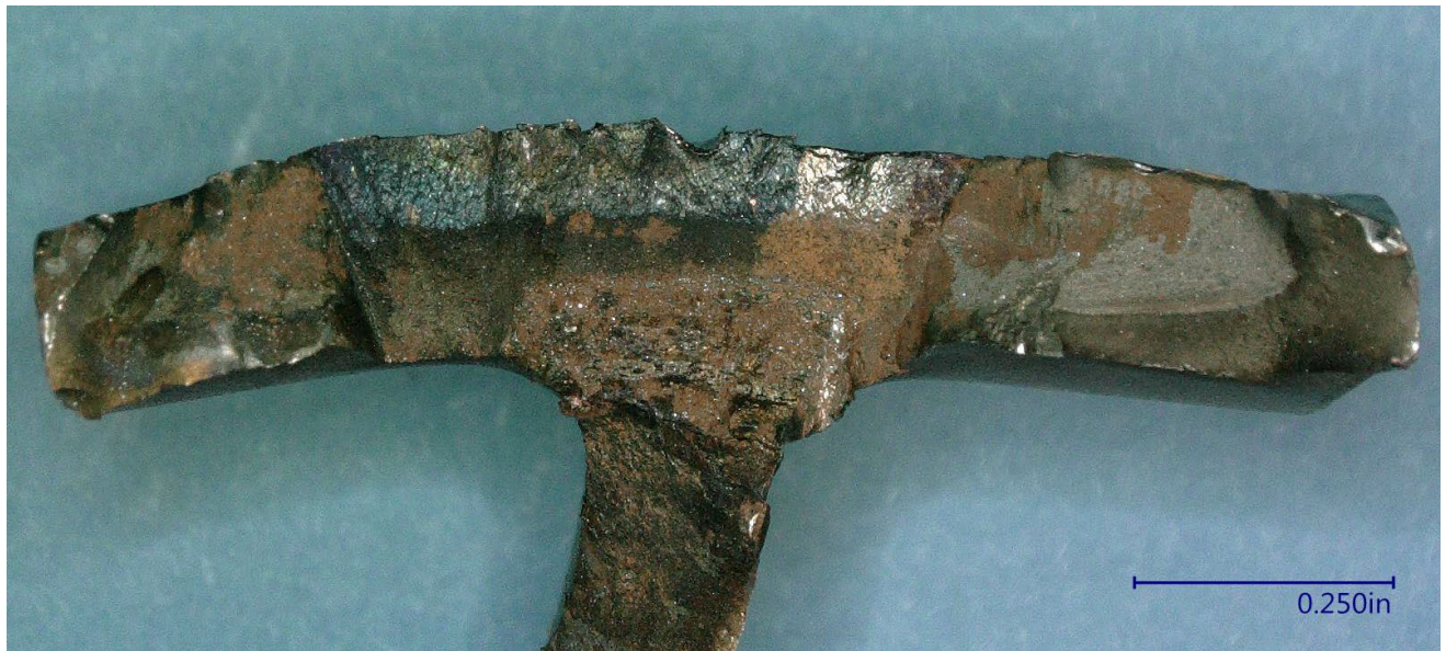
Figure 4 – Closer view of the upper flange in Figure 3, after sectioning but before cleaning.
