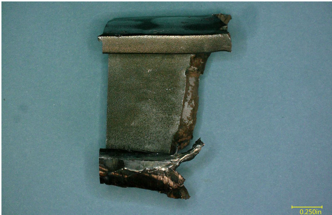
Figure 7 – Side view of the rod fragment fracture surface section, demonstrating the slanted fracture orientation on the web.
