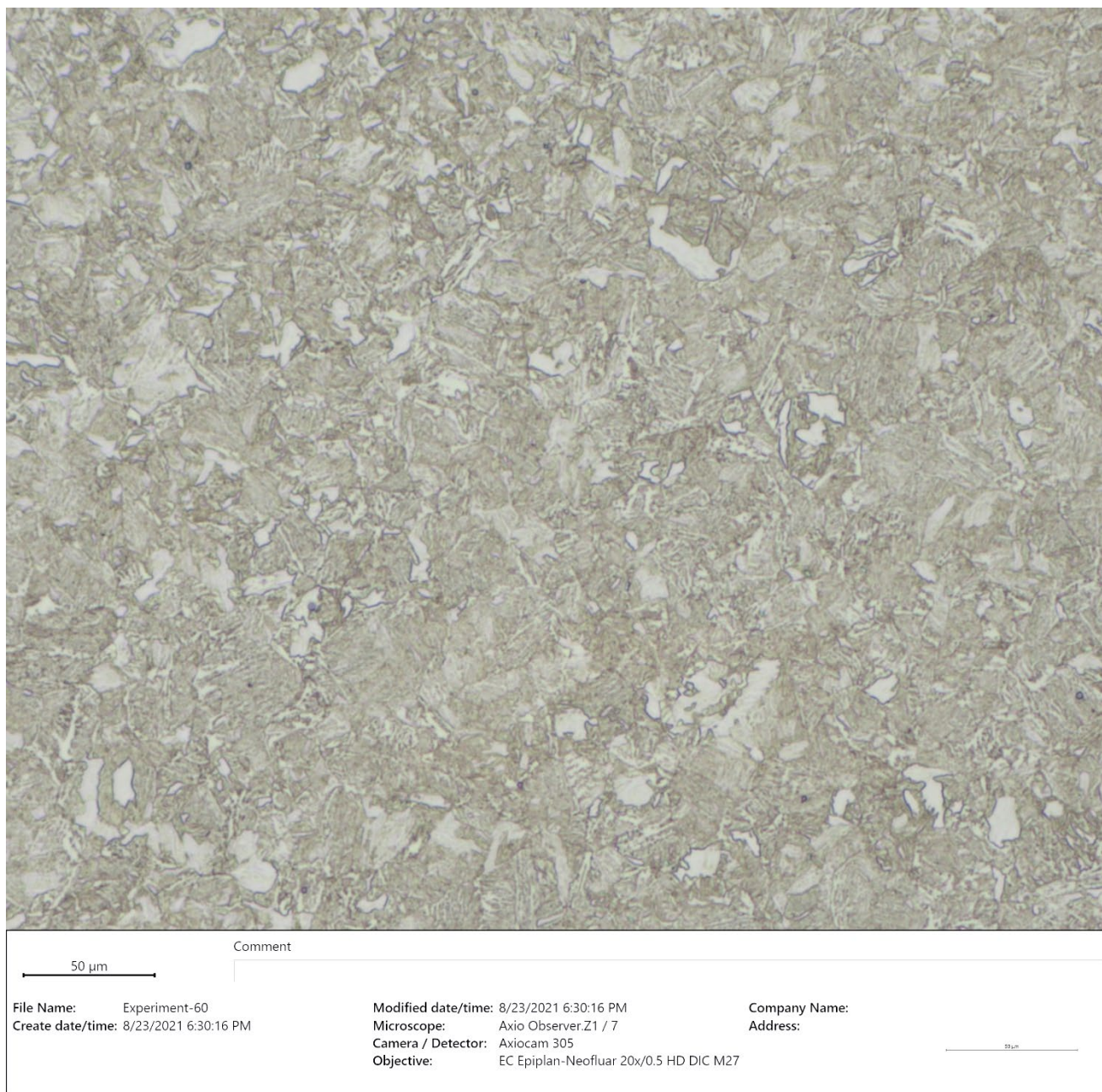
Figure 18 – Bright-field (BF) optical micrograph of a typical area of the rod microstructure from an area of the core, or away from the surface (~500X, etched 2% nital).
