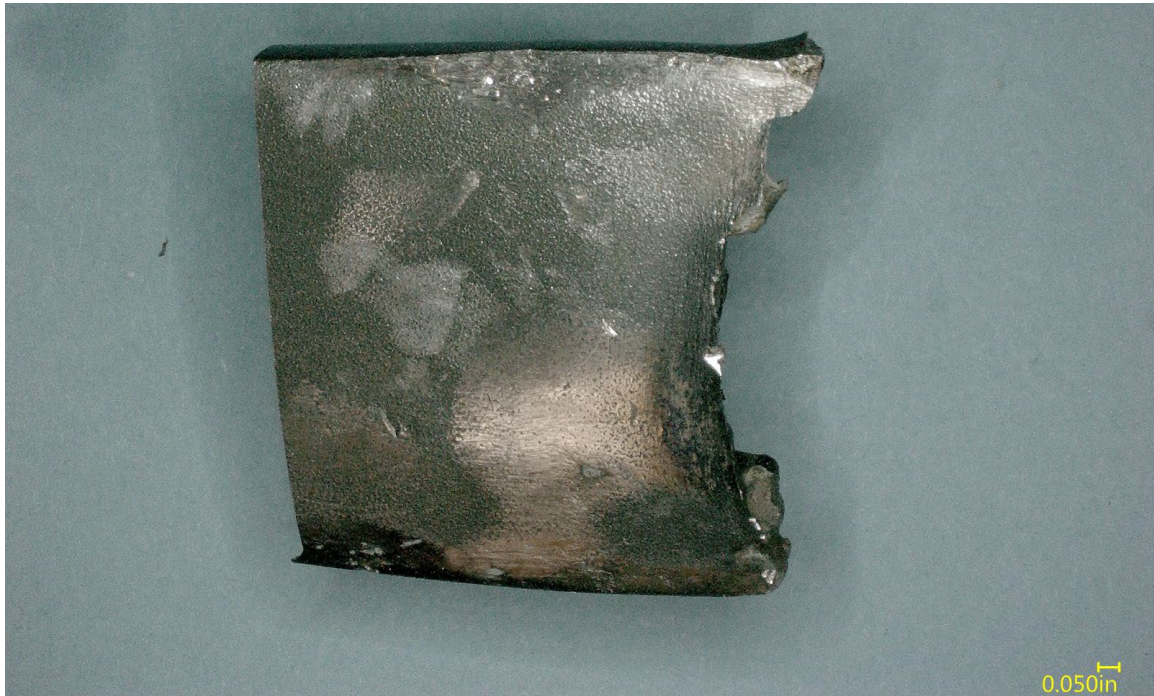
Figure 6 – Planar view of the face of the flange in Figure 4, showing deformation near the fracture.
