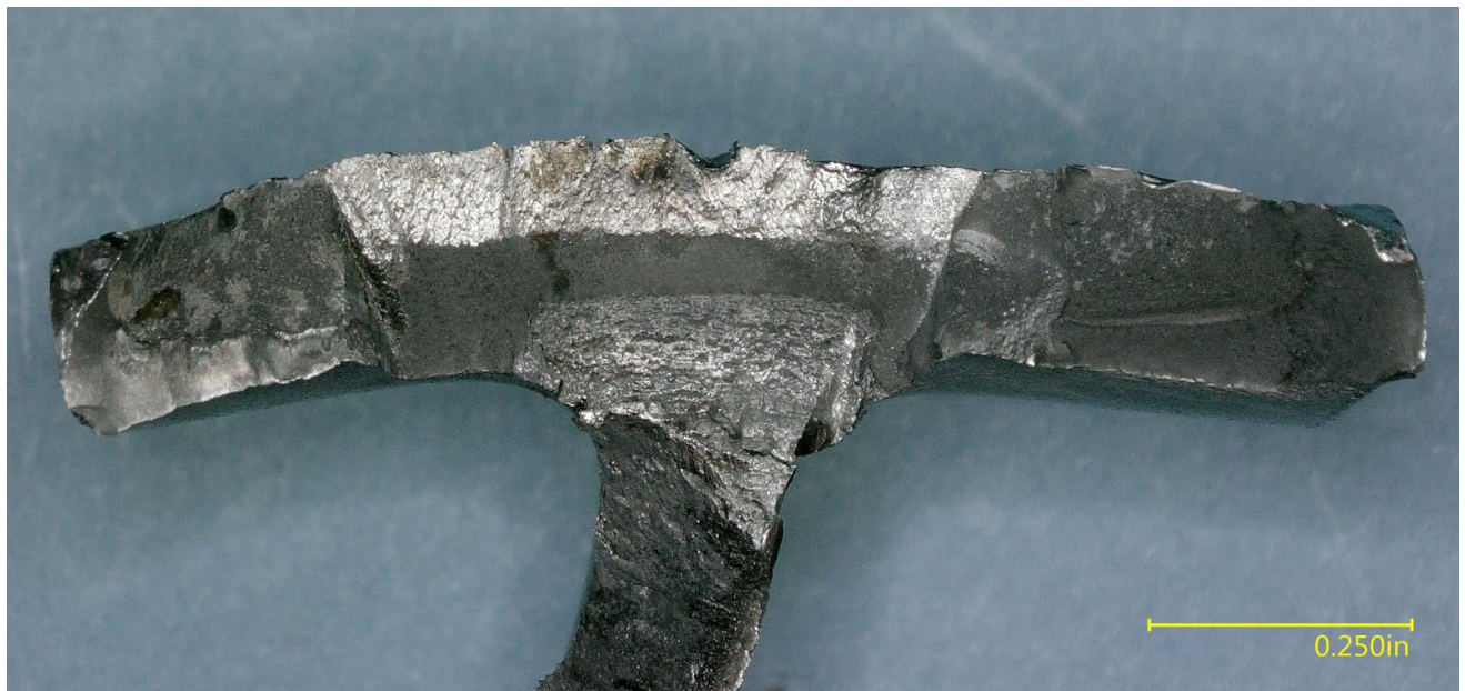
Figure 5 – The flange section shown in Figure 4, after cleaning.
