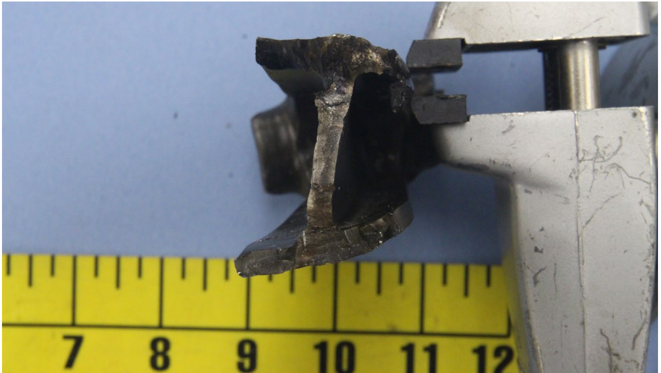
Figure 2 – View of the fracture surface of the connecting rod fragment, as received.
