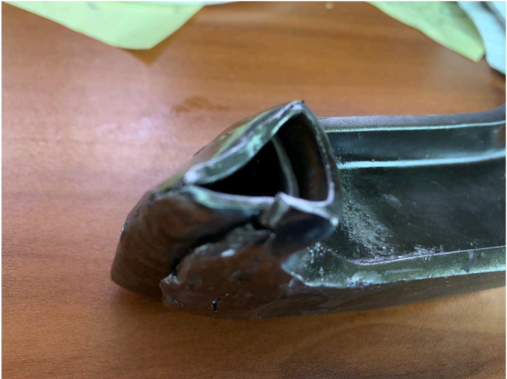
Photo 6 – Damaged connecting rod
