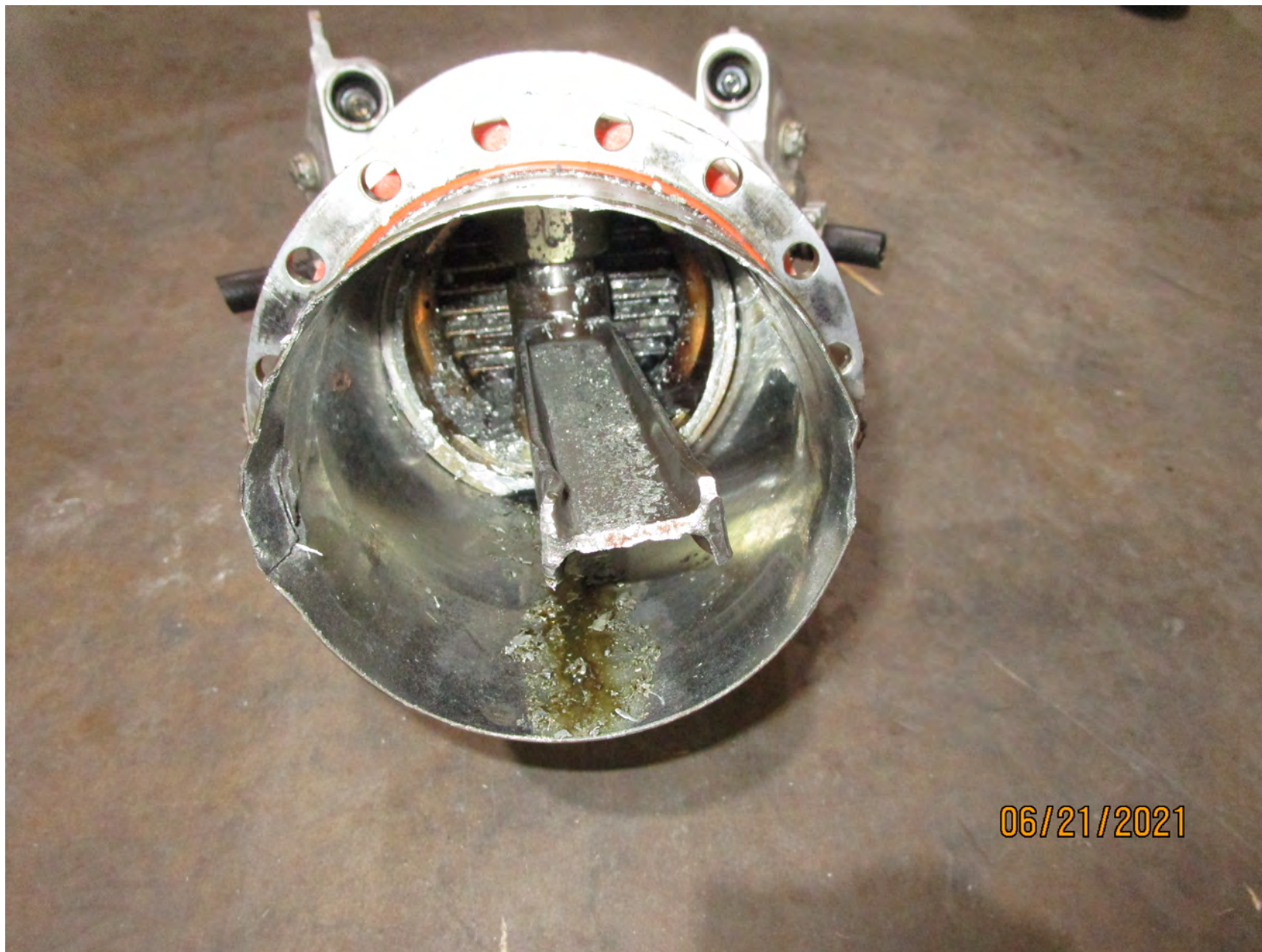
Photo 2 – Removed cylinder with broken connecting rod
