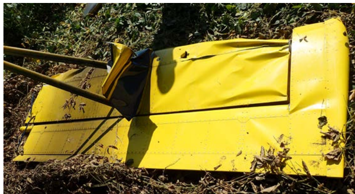
Left Horizontal Stabilizer and Elevator Wreckage
