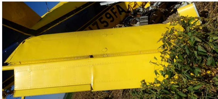
Right Horizontal Stabilizer and Elevator Wreckage
