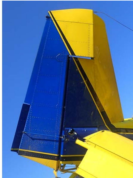
Vertical Stabilizer and Rudder Wreckage
